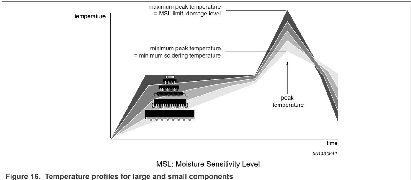
Figure 16. Temperature profiles for large and small components
