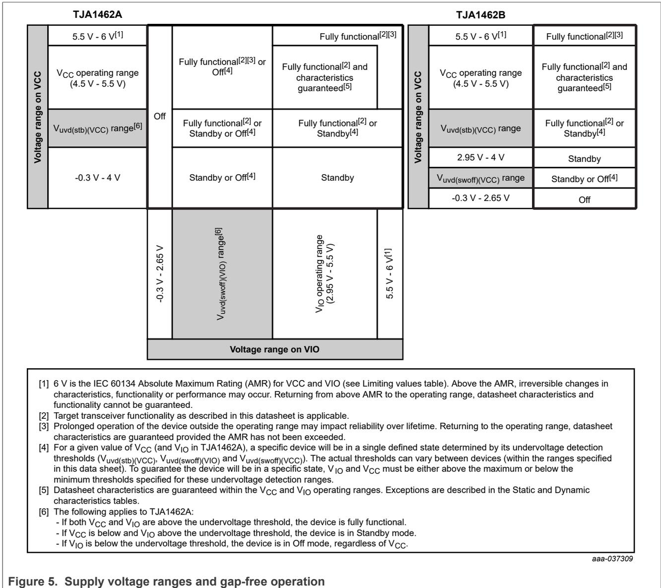
Figure 5. Supply voltage ranges and gap-free operation
