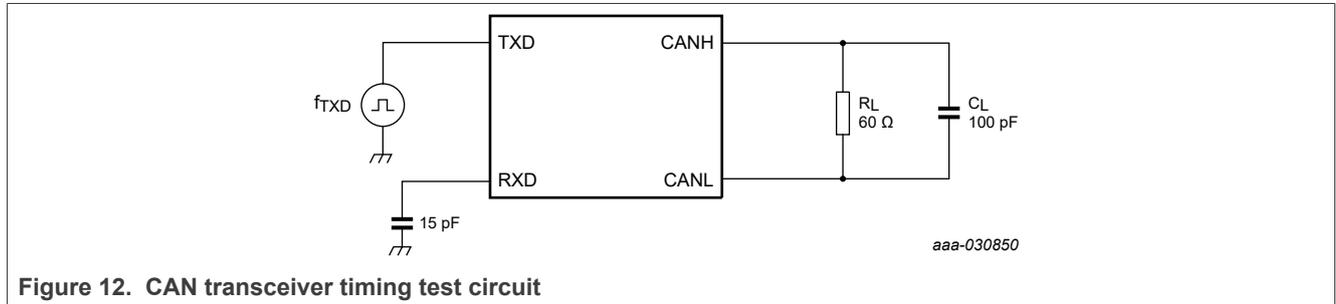
Figure 12. CAN transceiver timing test circuit
