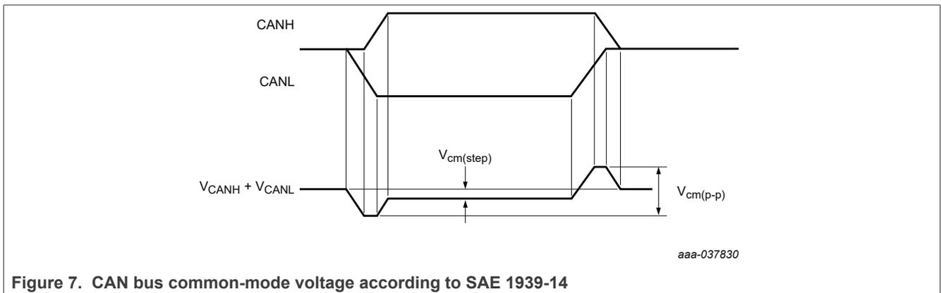
Figure 7. CAN bus common-mode voltage according to SAE 1939-14
