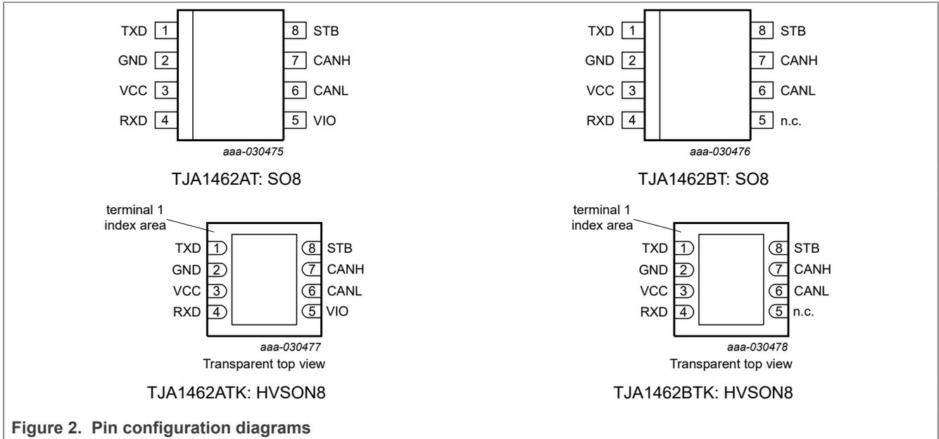
Figure 2. Pin configuration diagrams
