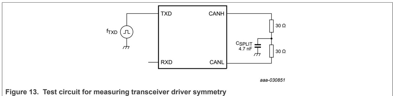
Figure 13. Test circuit for measuring transceiver driver symmetry
