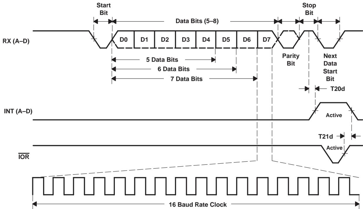
Figure 16. Receive Timing
