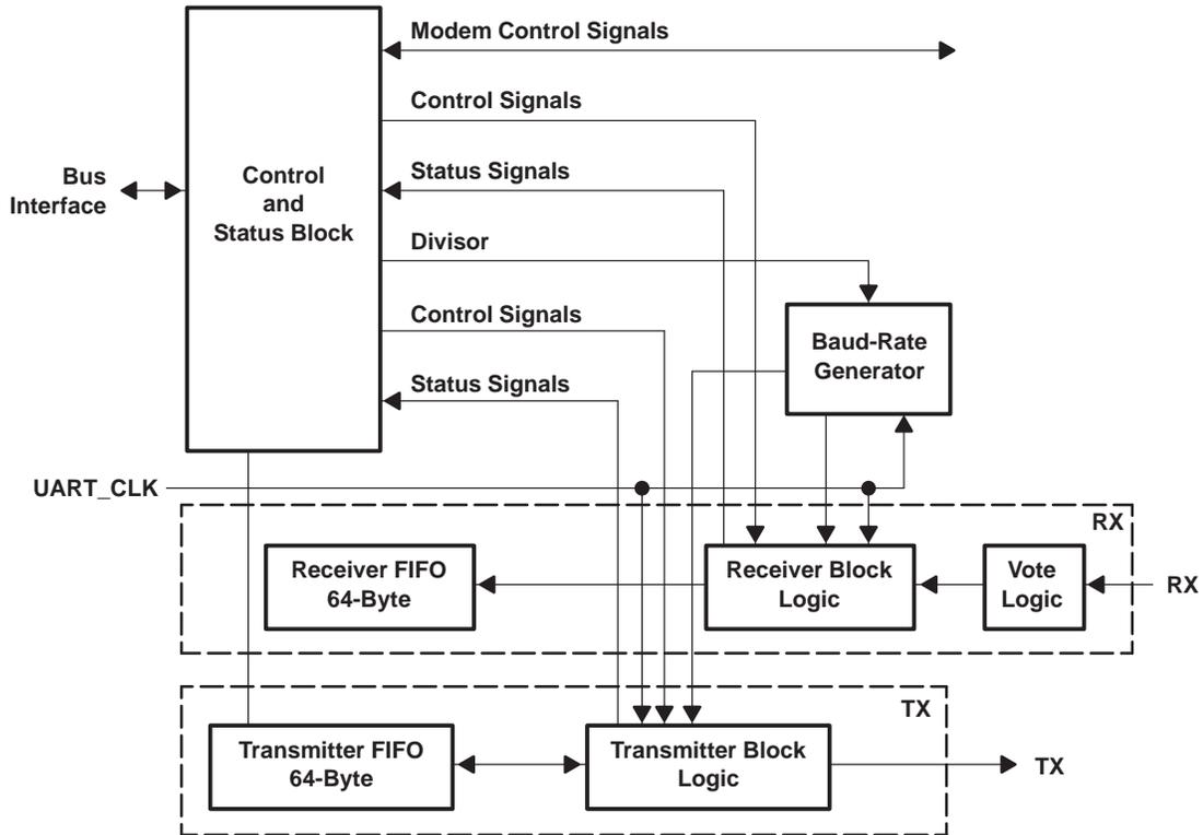
NOTE: The Vote logic determines whether the RX data is a logic 1 or 0. It takes three samples of the RX line and uses a majority vote to determine the logic level received. The Vote logic operates on all bits received.
