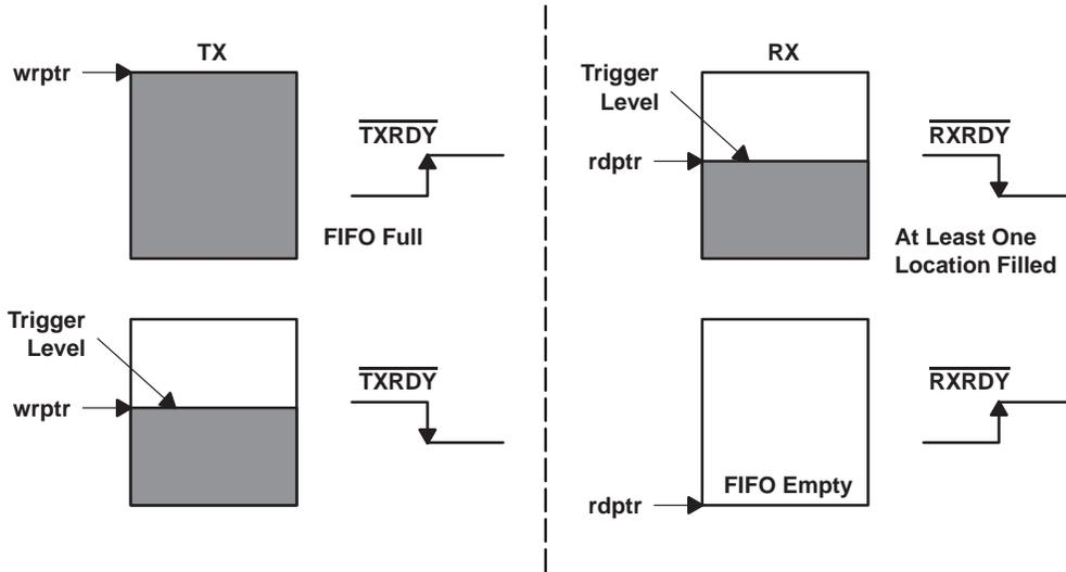
**Figure 8.  $\overline{\text{TXRDY}}$  and  $\overline{\text{RXRDY}}$  in DMA Mode 1**
