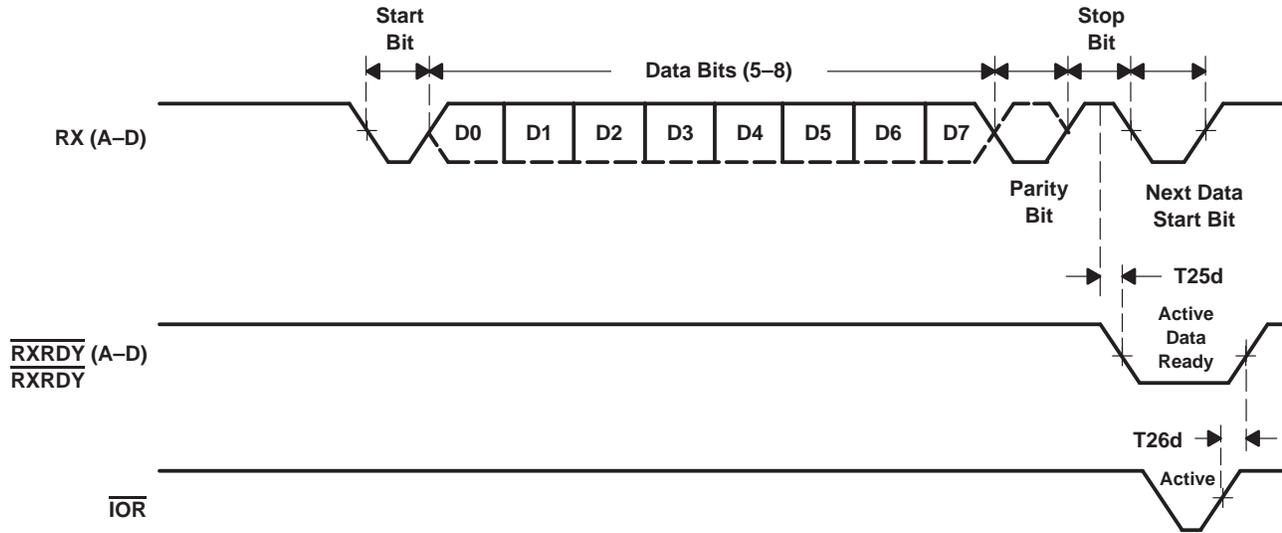
Figure 17. Receive Ready Timing in None FIFO Mode
