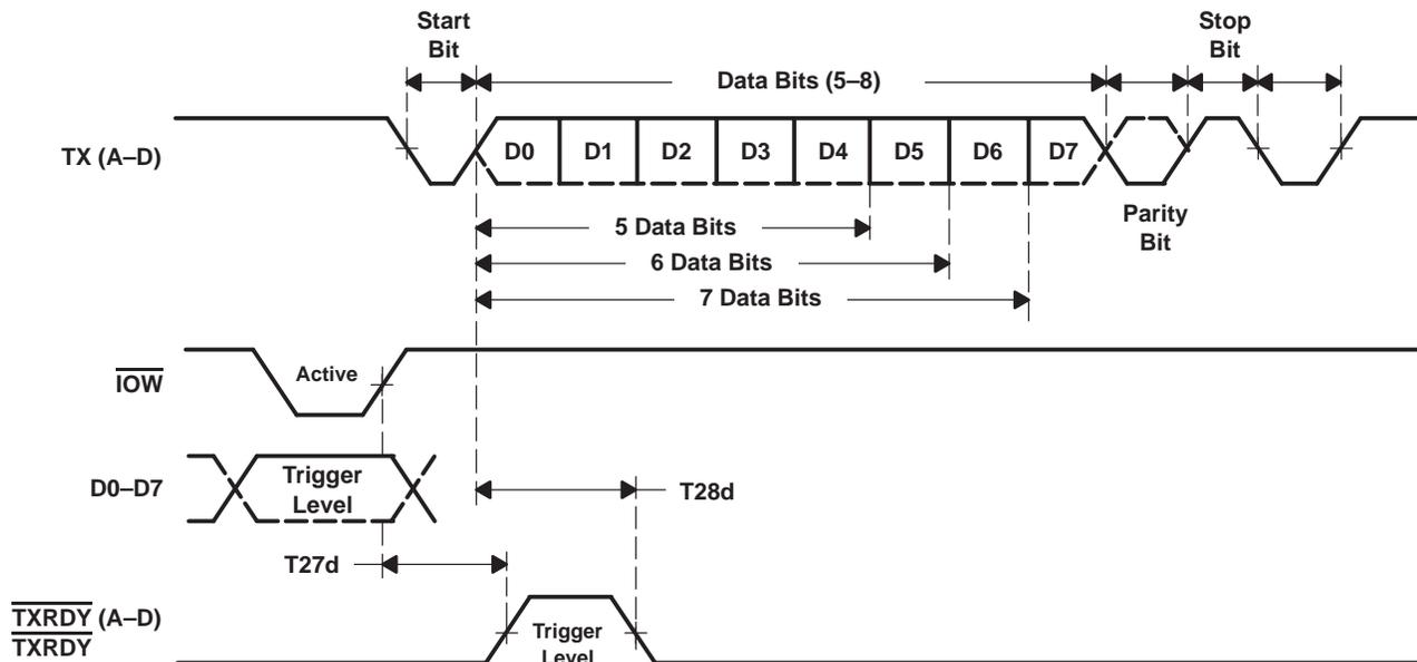
Figure 21. Transmit Ready Timing in FIFO Mode
