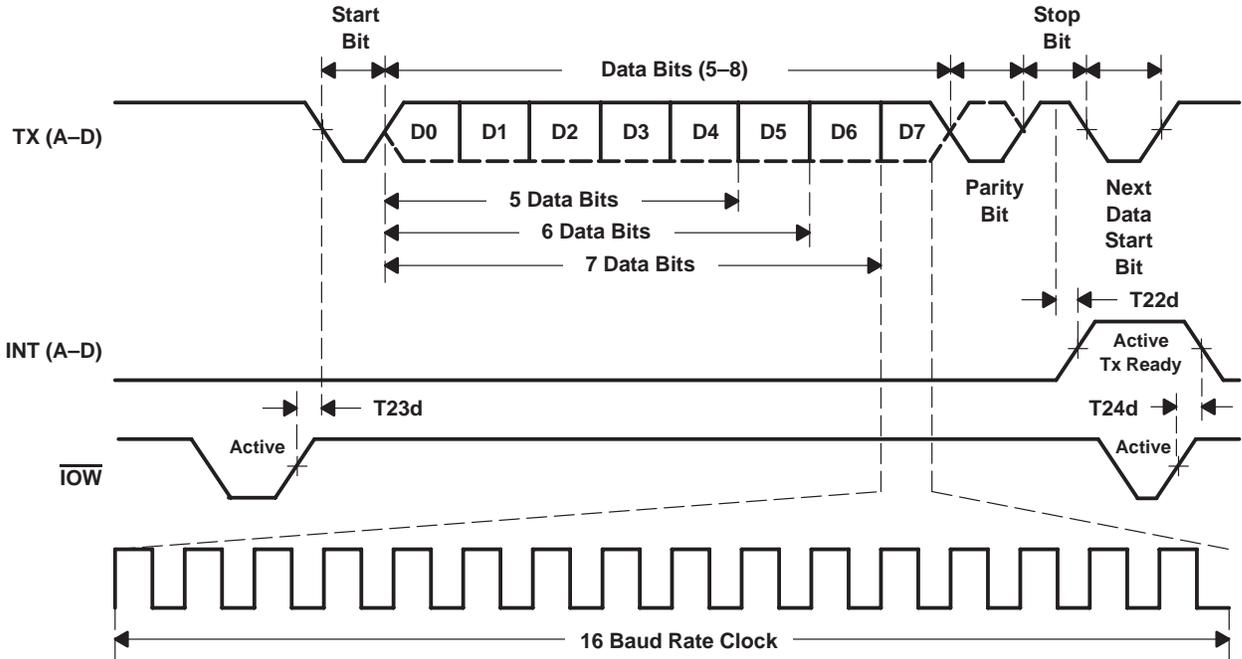
Figure 19. Transmit Timing
