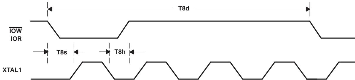
Figure 14. Alternate Read/Write Strobe Timing
