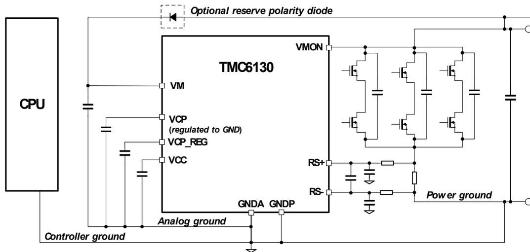
Figure 1.4 Ground connections
