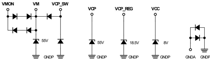
Figure 1.5 Supply connections
