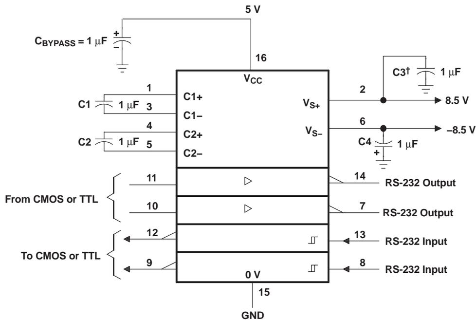
† C3 can be connected to V<sub>CC</sub> or GND.
