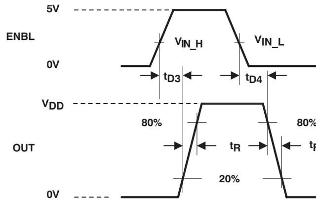
A. The 20% and 80% thresholds depict the dynamics of the Bipolar output devices that dominate the power MOSFET transition through the Miller regions of operation.
