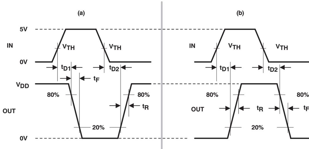
A. The 20% and 80% thresholds depict the dynamics of the Bipolar output devices that dominate the power MOSFET transition through the Miller regions of operation.
