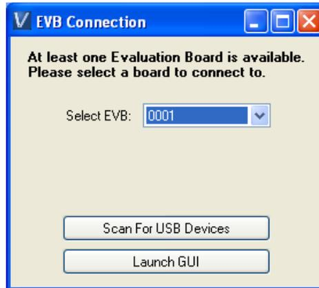
The EVB serial number should appear. If not, click on “Scan For USB Devices.” Select that EVB serial number then click “Launch GUI”. The Register List window will appear as shown in Figure 5.
