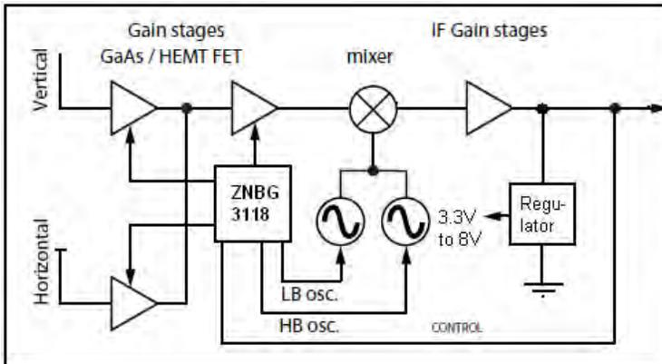
Figure 1 Typical single universal LNB system diagram
