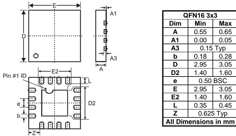
**Note:** Controlling dimensions are in millimetres. Approximate dimensions are provided in inches.
