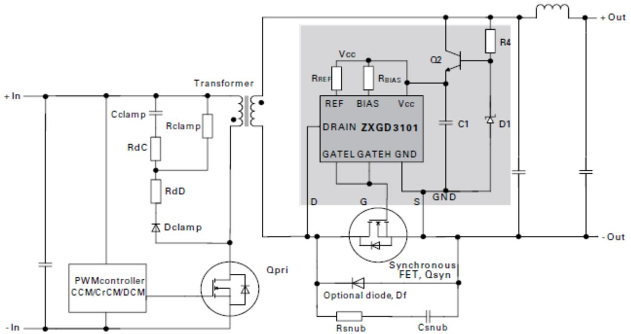
**Figure 2 - Example connection for low side synchronous rectification**
