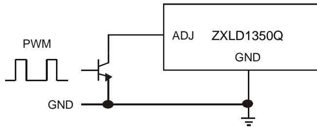
This scheme uses the 200kΩ resistor between the ADJ pin and the internal voltage reference as a pull-up resistor for the external transistor.
