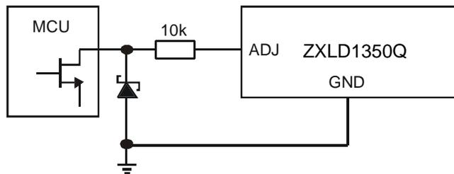
The diode and resistor suppress possible high amplitude negative spikes on the ADJ input resulting from the drain-source capacitance of the FET. Negative spikes at the input to the device should be avoided as they may cause errors in output current, or erratic device operation.
