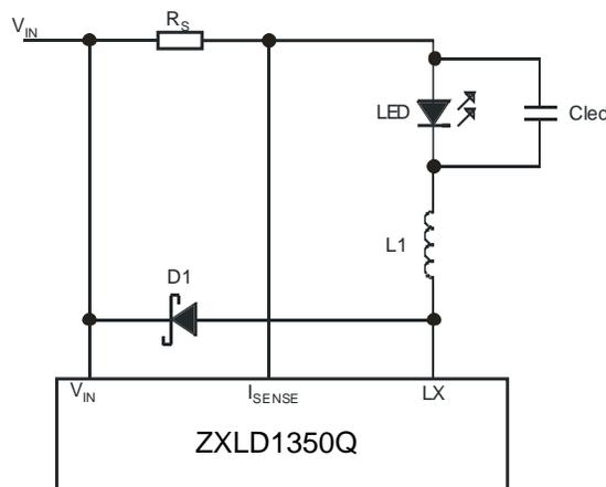
A value of 1µF will reduce nominal ripple current by a factor three (approx.). Proportionally lower ripple can be achieved with higher capacitor values. Note that the capacitor will not affect operating frequency or efficiency, but it will increase start-up delay, by reducing the rate of rise of LED voltage.
