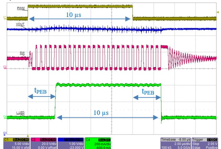
Figure 18: Zoom in view for PWM on-time = 10  $\mu$ s. Notice that the LED current is shifted with respect to PWM signal. Ripple at  $V_{OUT}$  is ~0.2 V when using  $2 \times 4.7 \mu$ F MLCC as output capacitors.
