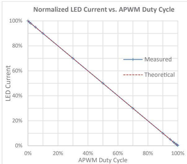
**Figure 24:** Showing LED current is inversely proportional to the APWM duty cycle. Test conditions:  $V_{IN} = 12\text{ V}$ ,  $V_{OUT} = 25\text{ V}$  ( $8 \times$  WLED), total LED current =  $100\text{ mA} \times 4$ , APWM frequency =  $100\text{ kHz}$
