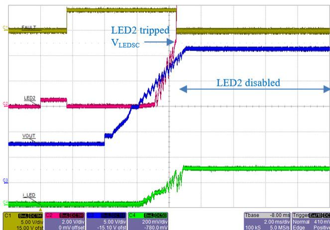
Figure 36: A80601 startup sequence when LED string#2 has a partial-short fault ( $6 \times \text{WLED}$  instead of 8). As soon as LED2 pin rises above  $V_{LESD}$  ( $\sim 5\text{ V}$ ), the channel is disabled and FAULT = Low.
