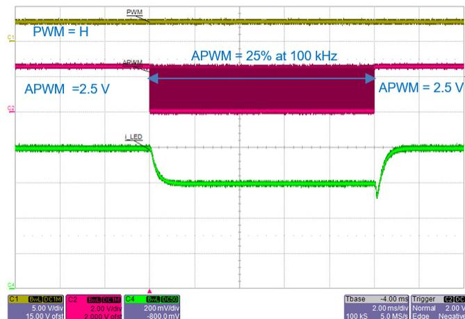
**Figure 25:** PWM = H. Total LED current drops from  $400\text{ mA}$  ( $4 \times 100\text{ mA/ch}$ ) to  $300\text{ mA}$  when APWM of 25% duty cycle is applied. Note that LED current takes  $\sim 0.5\text{ ms}$  to settle after change in APWM.
