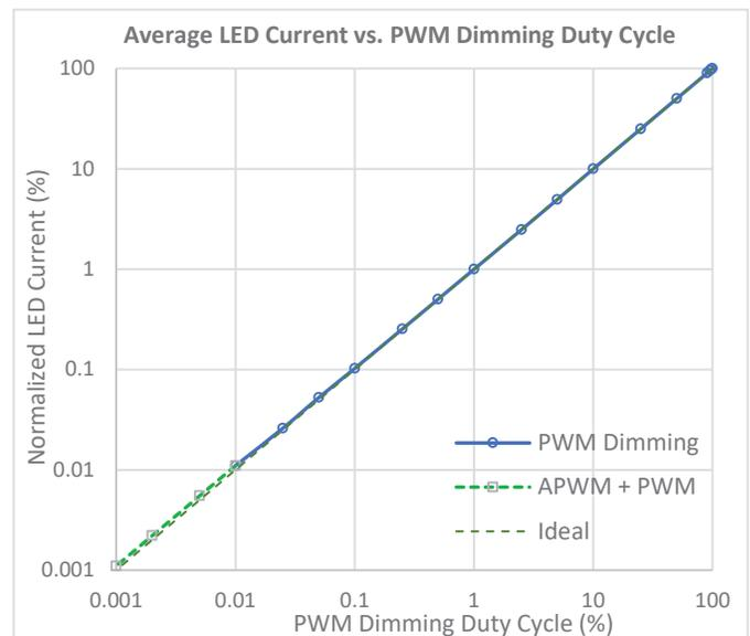
**Figure 27: How to achieve 100,000:1 dimming ratio by using both PWM and APWM. Test conditions:  $V_{IN} = 12$  V,  $V_{OUT} = 25$  V ( $8 \times$  WLED), total LED current = 400 mA, PWM frequency = 200 Hz, APWM frequency = 100 kHz.**
