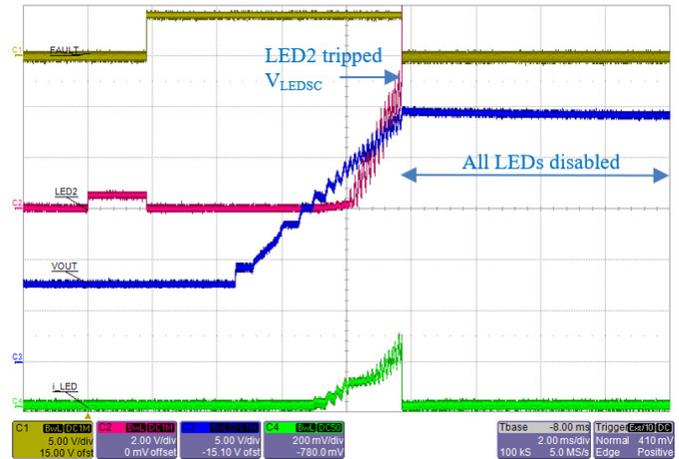
Figure 37: A80601-1 startup sequence when LED string#2 has a partial-short fault ( $6 \times \text{WLED}$  instead of 8). As soon as LED2 pin rises above  $V_{LESD}$  ( $\sim 5\text{ V}$ ), the channel is disabled but FAULT remains High.
