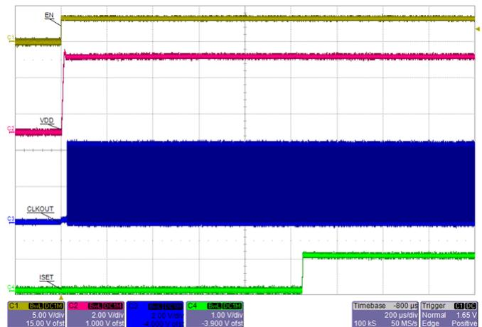
**Figure 3: Startup showing EN, VDD, CLKOUT, and ISET (PWM = L).**
