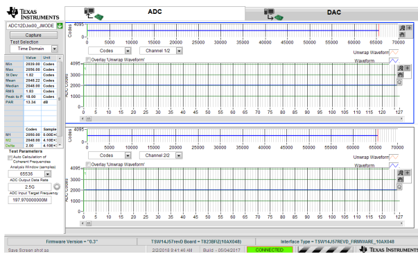
Figure 7-10. Idle-Channel Noise (No Input) for 2.5-GSPS, Dual-Channel Oscilloscope
