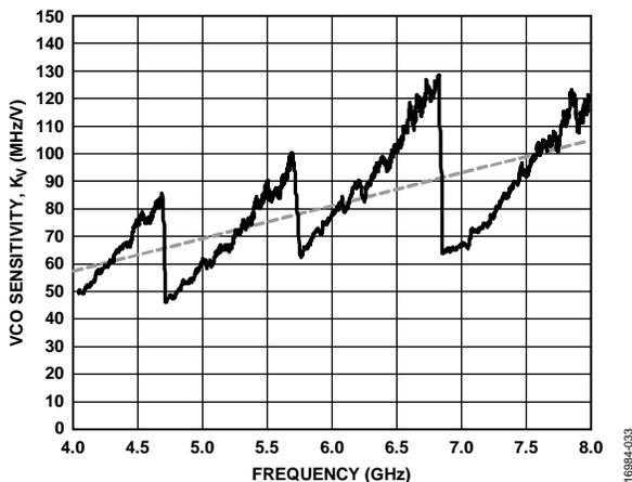
Figure 33. VCO Sensitivity,  $K_V$  vs. Frequency,  $VCC\_VCO = 5 V$
