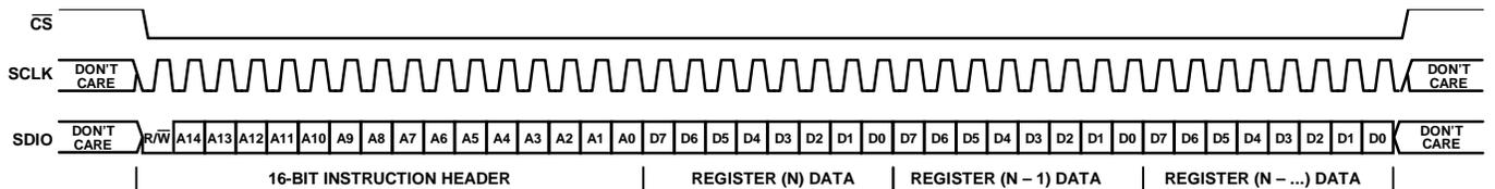
Figure 5. 3-Wire, MSB First, Descending Data, Streaming
