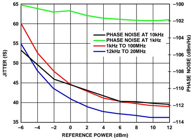
Figure 27. Jitter and Phase Noise,  $f_{\text{PFD}} = 250$  MHz
