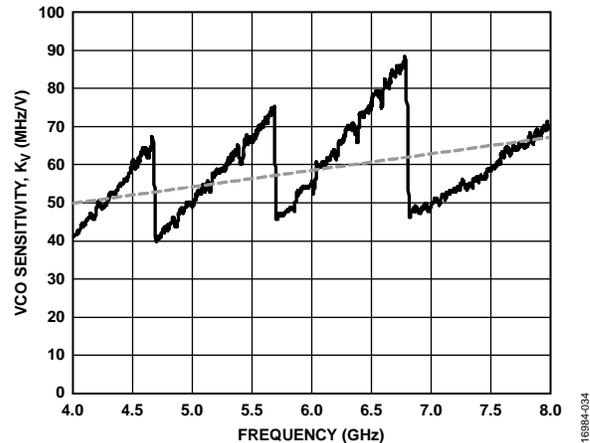
Figure 34. VCO Sensitivity,  $K_V$  vs. Frequency,  $VCC\_VCO = 3.3 V$
