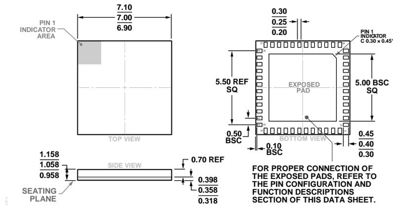
Figure 38. 48-Terminal Land Grid Array [LGA] (CC-48-4)
