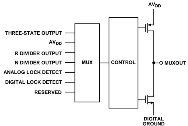
Figure 32. MUXOUT Schematic
