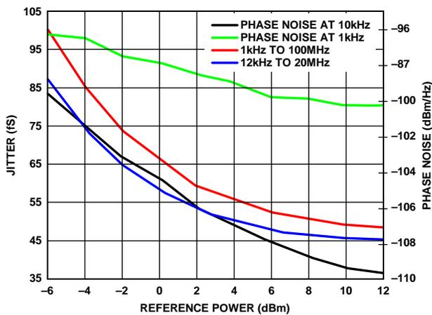
Figure 28. Jitter and Phase Noise,  $f_{\text{PFD}} = 100$  MHz
