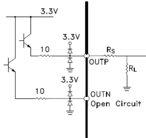
Figure 12 DC Coupled to CMOS Interface
