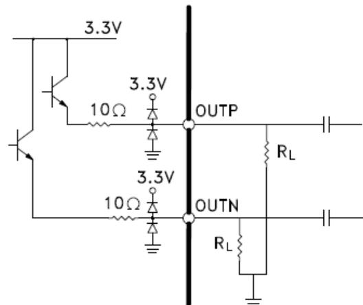
Figure 11 AC coupled to LVDS / CML / LVPECL / CMOS
