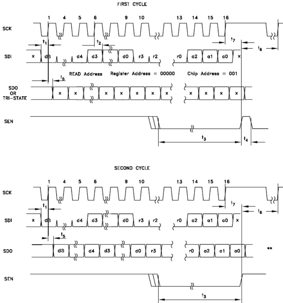
Figure 16 SPI Diagram, Read Operation 2- Cycles
