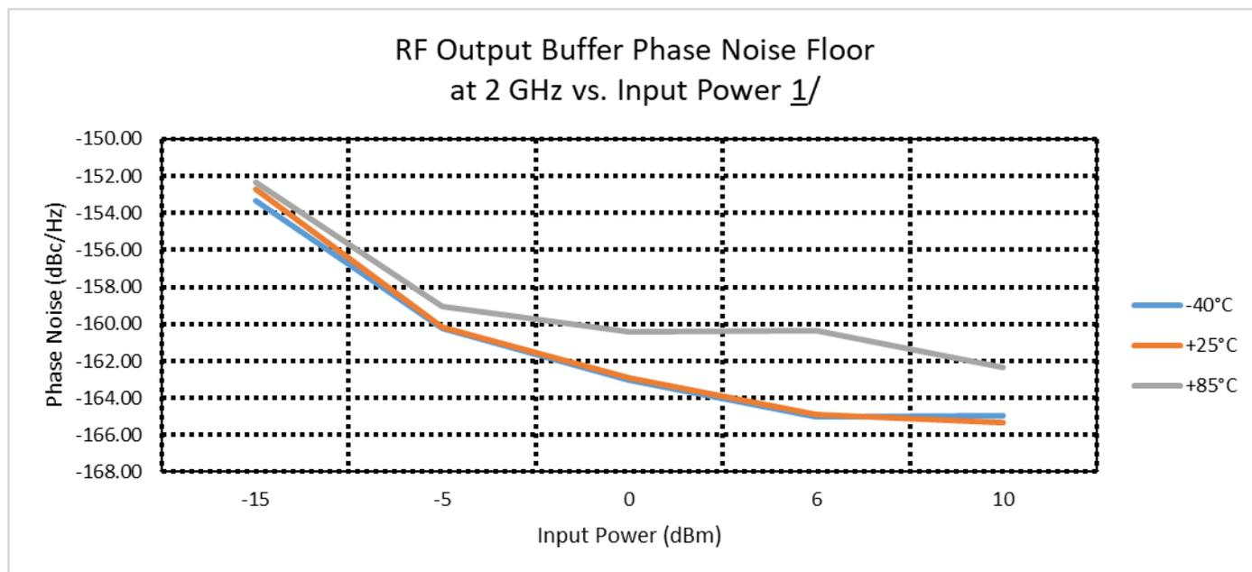
1/ Output not corrected for board, cable and adapter loss. Clock input driven differentially. Outputs are single-ended. Not tested post irradiation. Parameter is part of device initial characterization which is only repeated after design and process changes or with subsequent lots.
