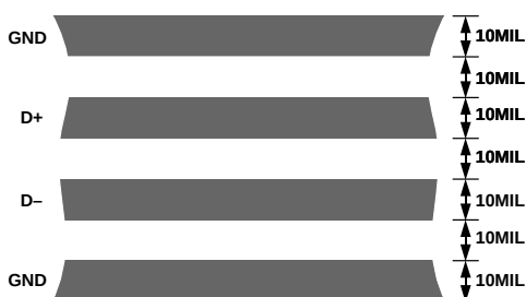
Figure 18. Arrangement of Signal Tracks
