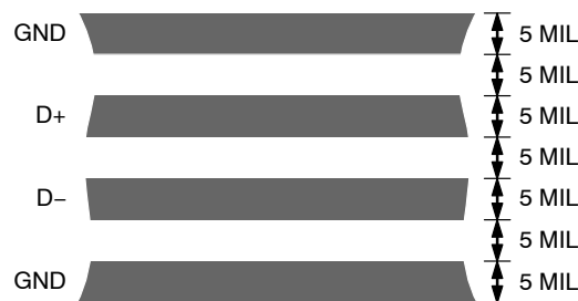
Figure 28. Arrangement of Signal Tracks
