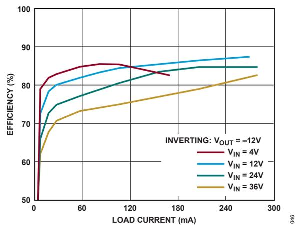
Figure 47. Efficiency vs. Load Current (Figure 46 Circuit)
