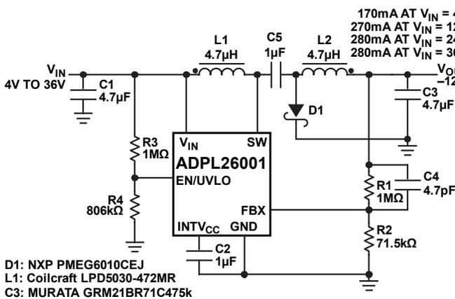
Figure 46. 4V to 36V Input, -12V Inverting Converter
