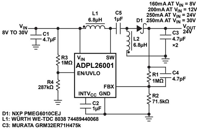
Figure 38. 8V to 30V, 24V SEPIC Converter
