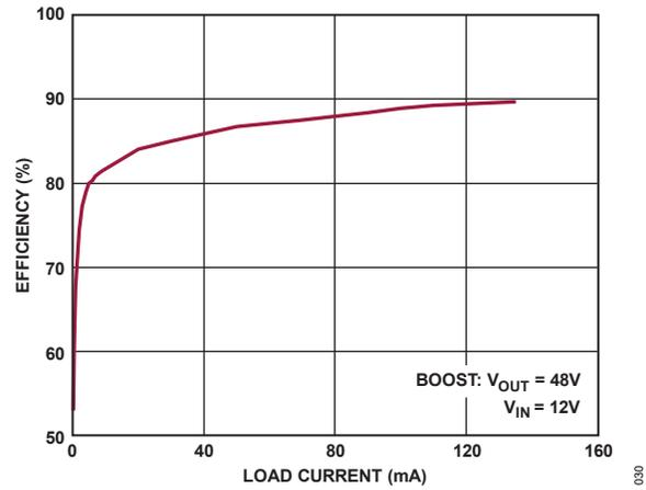
Figure 31. Efficiency vs. Load Current (Figure 30 Circuit)
