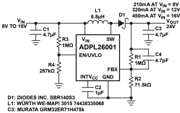
Figure 32. 8V to 16V Input, 24V Boost Converter
