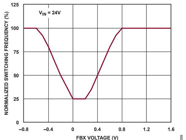
Figure 11. Normalized Switching Frequency vs. FBX Voltage
