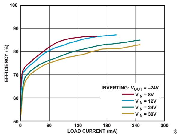
Figure 45. Efficiency vs. Load Current (Figure 44 Circuit)
