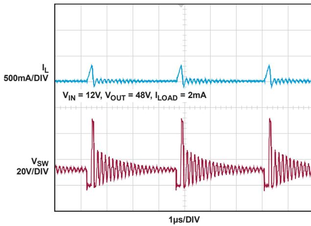
Figure 20. Switching Waveforms (Figure 30 Circuit in Deep Burst Mode)
