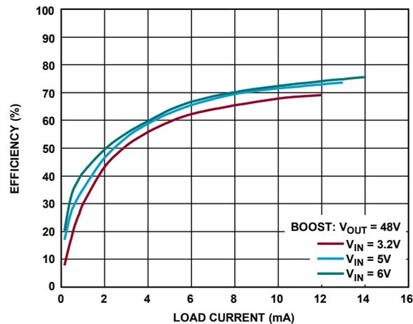
Figure 35. Efficiency vs. Load Current (Figure 34 Circuit)
