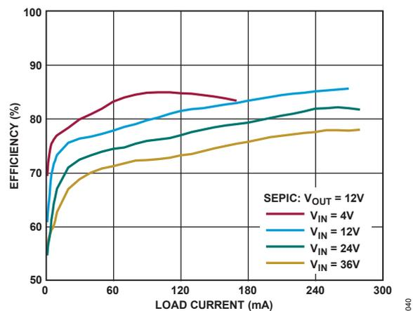
Figure 41. Efficiency vs. Load Current (Figure 40 Circuit)
