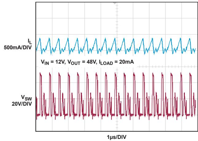
Figure 19. Switching Waveforms (Figure 30 Circuit in DCM/Light Burst Mode)
