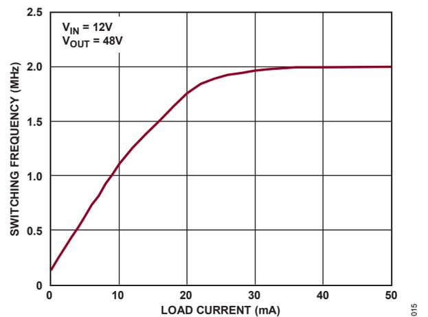
Figure 17. Burst Frequency vs. Load Current (Figure 30 Circuit)
