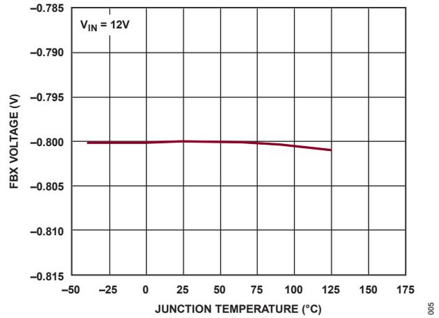
Figure 7. FBX Negative Regulation Voltage vs. Temperature
