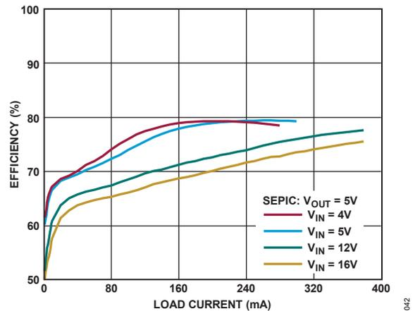
Figure 43. Efficiency vs. Load Current (Figure 42 Circuit)
