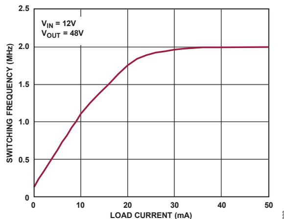
**Figure 23. Burst Frequency vs. Load Current (Figure 30 Circuit)**
