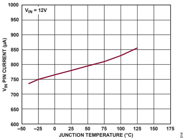
Figure 16. V<sub>IN</sub> Pin Current (Active Mode, Not Switching) vs. Temperature
