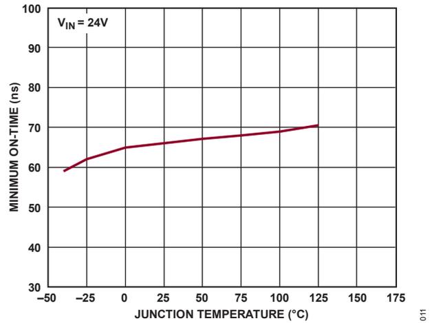
Figure 13. Switch Minimum On-Time vs. Temperature
