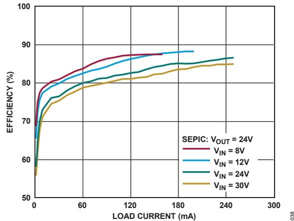
Figure 39. Efficiency vs. Load Current (Figure 38 Circuit)
