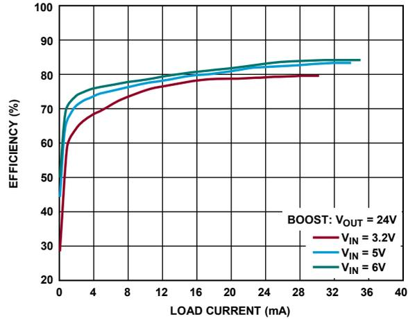
Figure 37. Efficiency vs. Load Current (Figure 36 Circuit)
