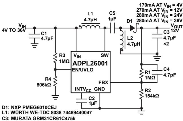
Figure 40. 4V to 36V, 12V SEPIC Converter
