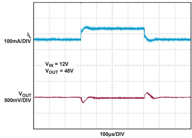
Figure 21.  $V_{OUT}$  Transient-Response: Load Current Transients from 67.5mA to 135mA to 67.5mA (Figure 30 Circuit)
