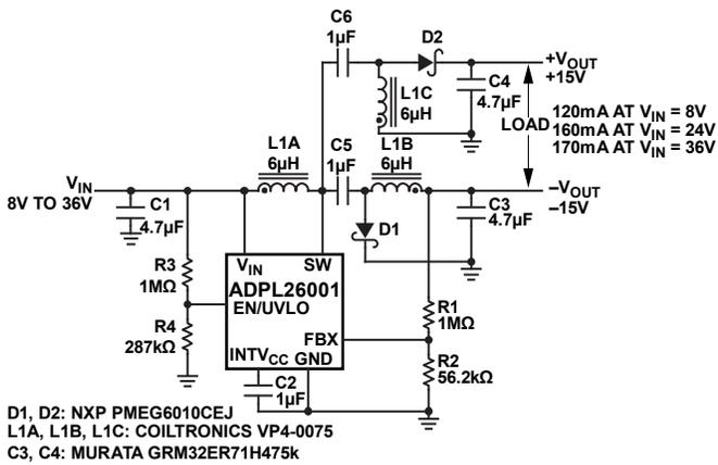
Figure 50. 8V to 40V Input, ±15V Converter
