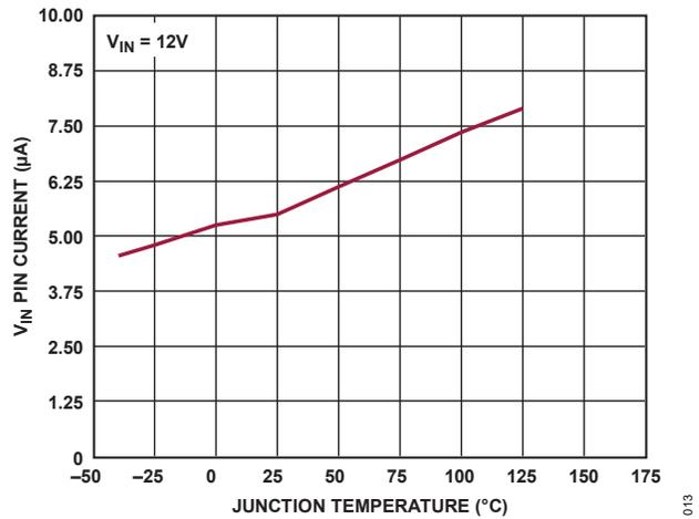
Figure 15. V<sub>IN</sub> Pin Current (Sleep Mode, Not Switching) vs. Temperature
