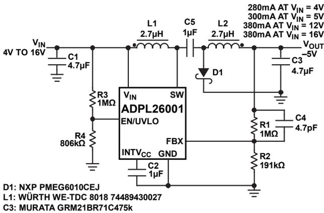
Figure 48. 4V to 16V Input, -5V Inverting Converter
