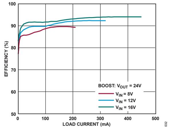
Figure 33. Efficiency vs. Load Current (Figure 32 Circuit)
