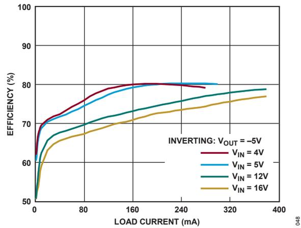
Figure 49. Efficiency vs. Load Current (Figure 48 Circuit)
