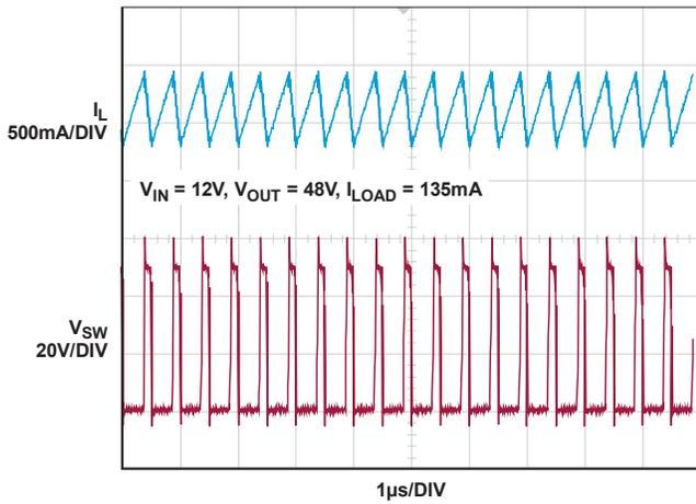
Figure 18. Switching Waveforms (Figure 30 Circuit in CCM)
