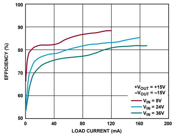
Figure 51. Efficiency vs. Load Current (Figure 50 Circuit)
