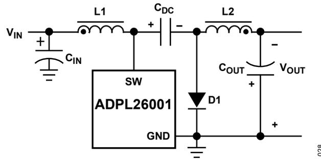
Figure 29. A Simplified Inverting Converter
