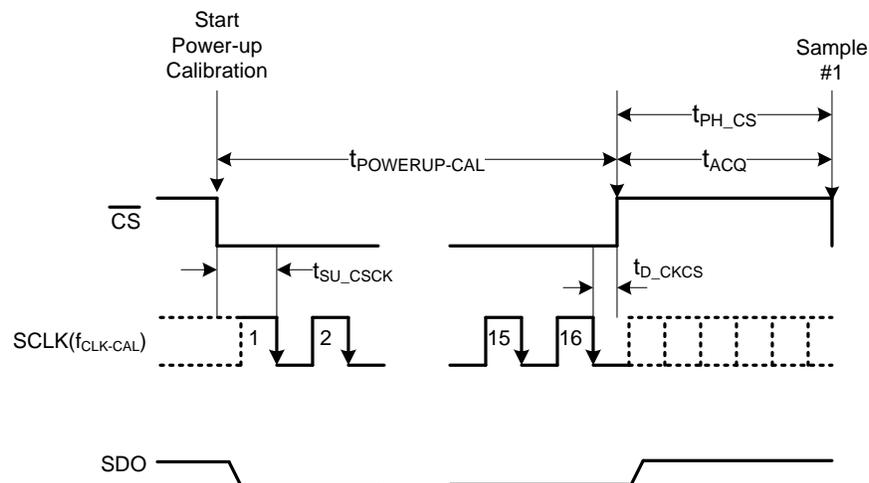
**Figure 38. Offset Calibration on Power-Up Timing Diagram**
