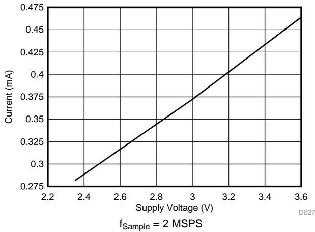
**Figure 26. AVDD Supply Current vs Supply Voltage**
