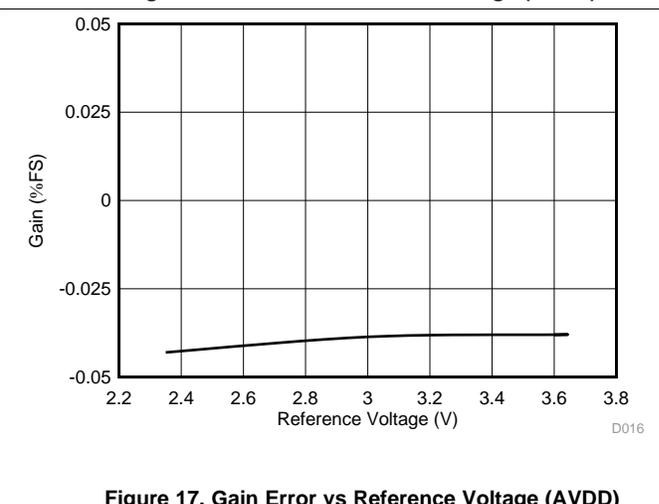
Figure 17. Gain Error vs Reference Voltage (AVDD)
