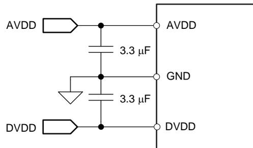
Figure 43. Power-Supply Decoupling
