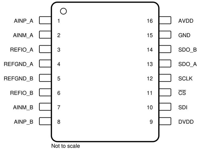
**Figure 5-1. PW Package, 16-Pin TSSOP (Top View)**
