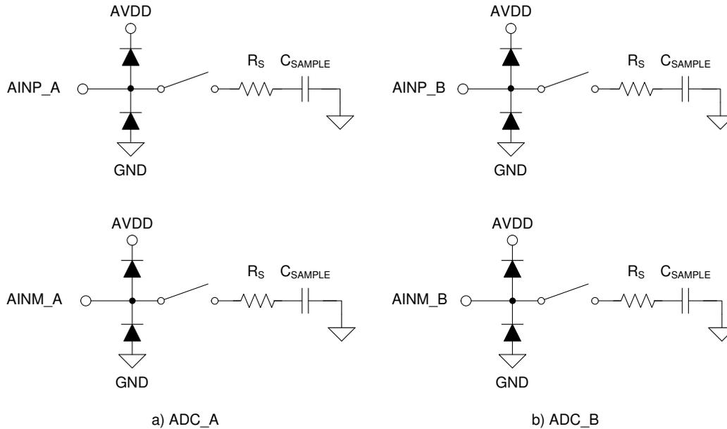
Figure 7-2. Equivalent Circuit for the Analog Input Pins
