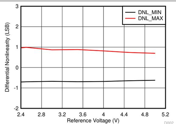
Figure 6-18. DNL vs Reference Voltage
