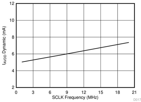
**Figure 6-10. Analog Supply Current vs SCLK Frequency**
