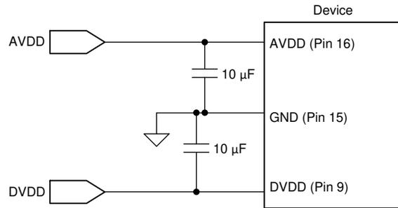
**Figure 8-5. Power-Supply Decoupling**
