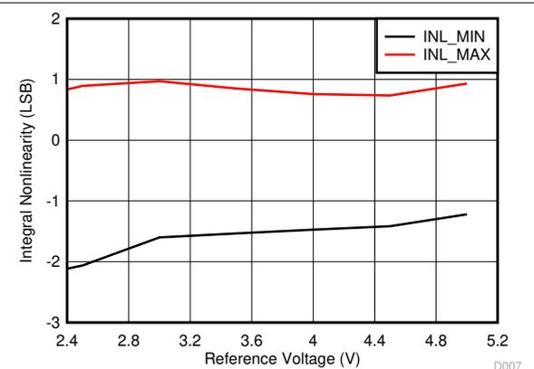
Figure 6-19. INL vs Reference Voltage
