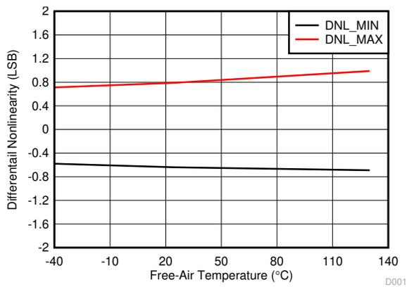
Figure 6-16. DNL vs Temperature
