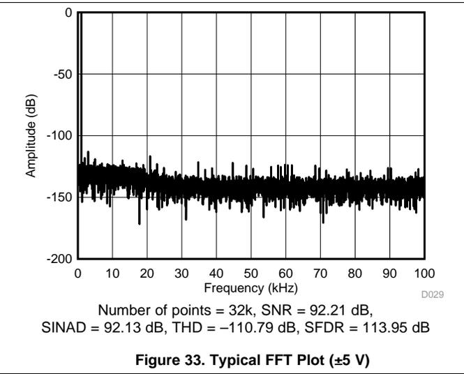
Figure 33. Typical FFT Plot ( $\pm 5\text{ V}$ )
