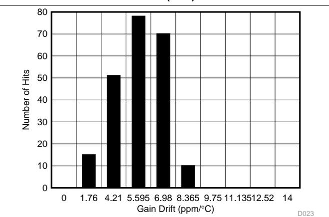
Figure 27. Gain Error Drift Histogram Distribution ( $\pm 10\text{ V}$ )
