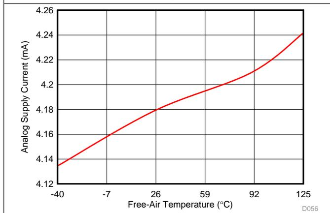
Figure 50. Analog Supply Current vs Temperature (Standby)
