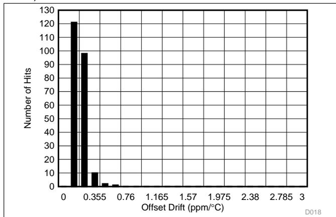
Figure 22. Offset Drift Histogram Distribution ( $\pm 10\text{ V}$ )
