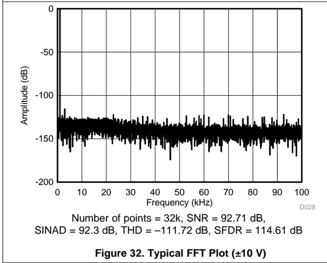
Figure 32. Typical FFT Plot ( $\pm 10\text{ V}$ )
