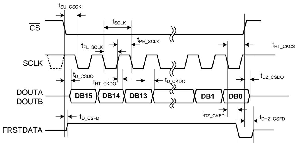
Figure 5. Serial Data Read Operation Timing Diagram
