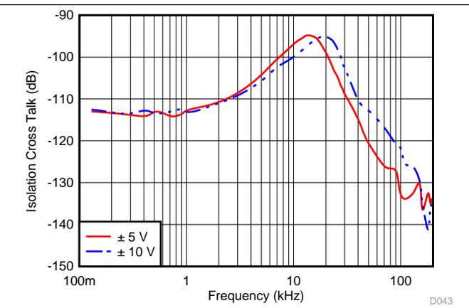
Figure 47. Isolation Crosstalk vs Noise Frequency (Saturated Inputs)
