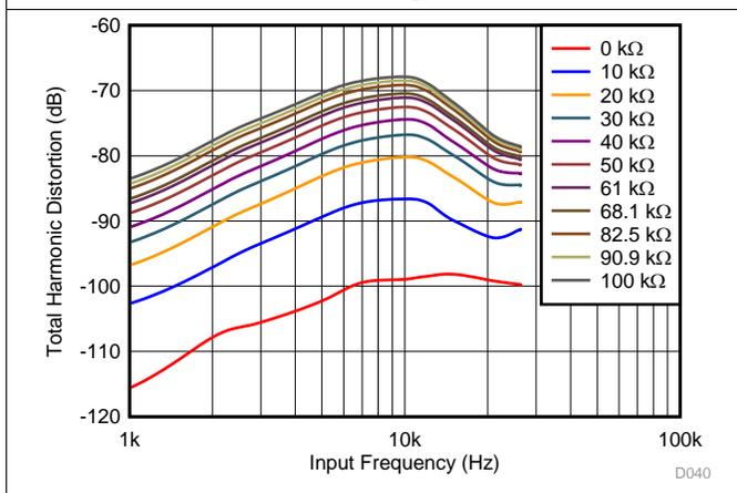
**Figure 44. THD vs Input Frequency for Different Source Impedances ( $\pm 10\text{ V}$ )**
