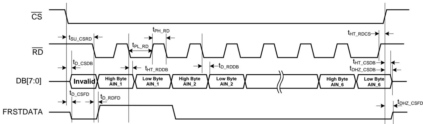
Figure 6. Byte Mode Data Read Operation Timing Diagram
