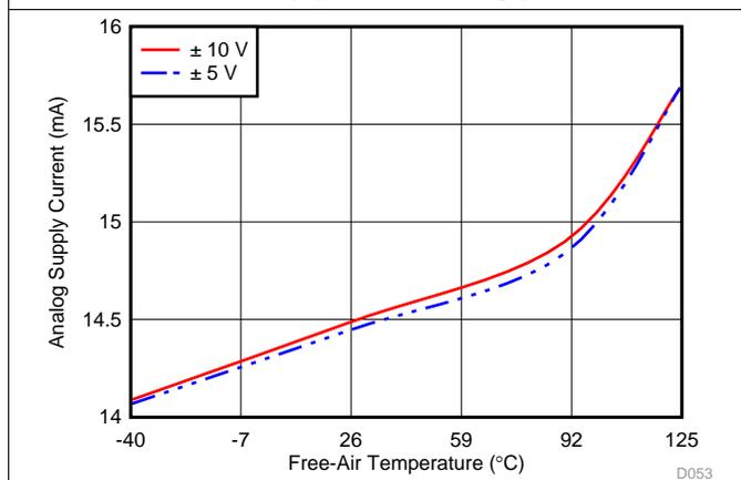
Figure 48. Analog Supply Current (Operational) vs Temperature
