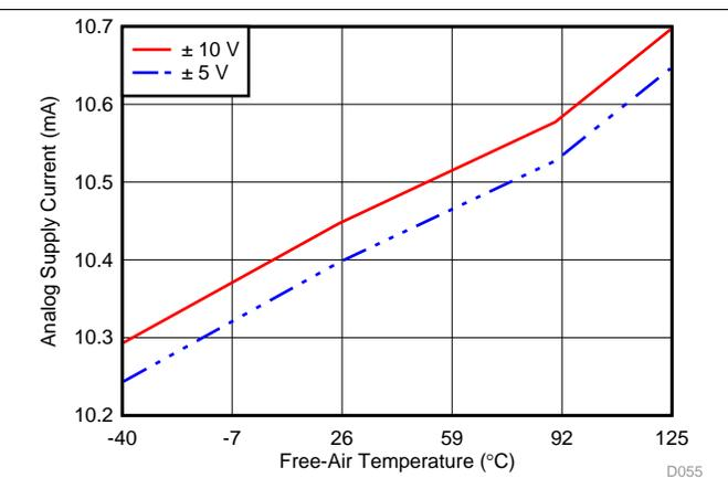
Figure 49. Analog Supply Current (Static) vs Temperature (Sampling)
