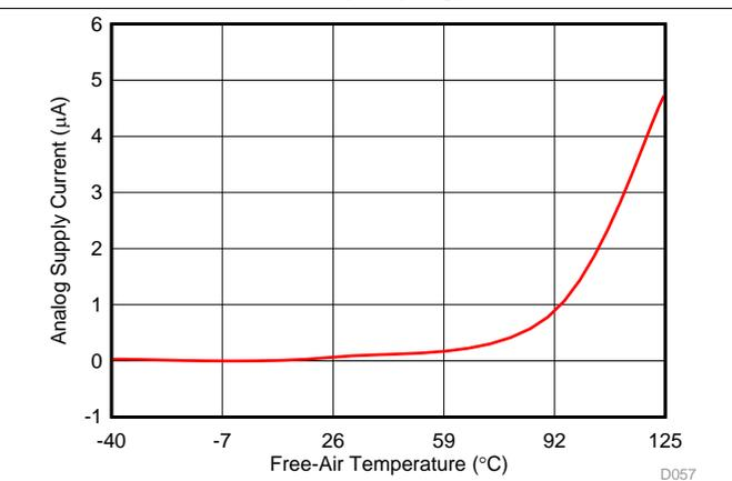
Figure 51. Analog Supply Current vs Temperature (Shutdown)
