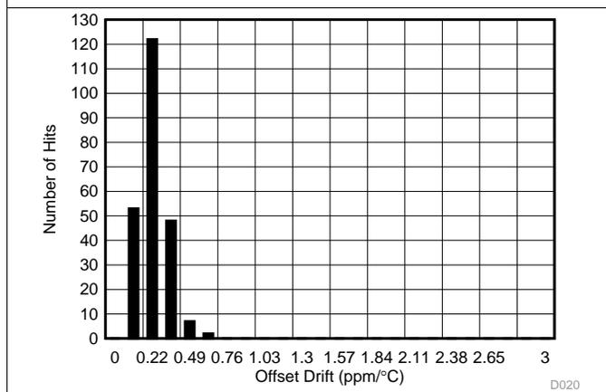
Figure 24. Offset Drift Histogram Distribution ( $\pm 5\text{ V}$ )
