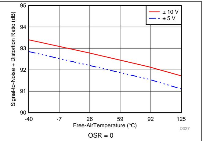
**Figure 41. SINAD vs Temperature for Different Input Ranges**
