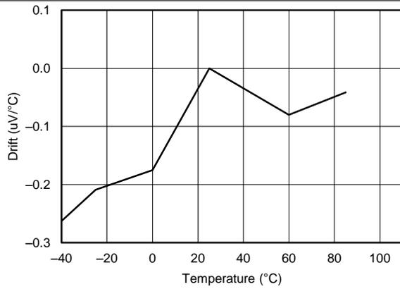
Figure 2. CC Input Offset Drift Overtemperature
