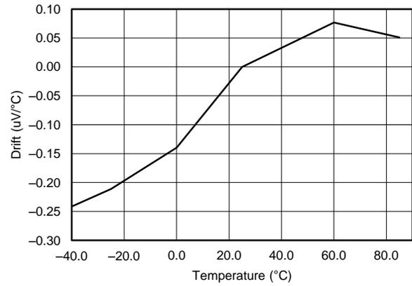
Figure 3. ADC Input Offset Drift Overtemperature
