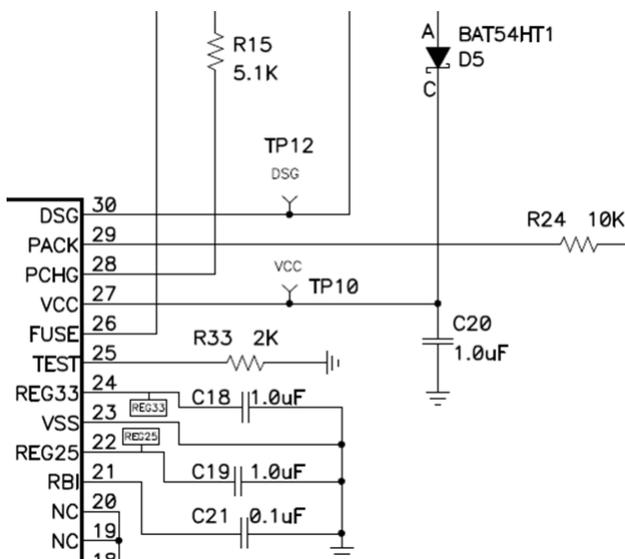
Figure 12. Power Supply Decoupling
