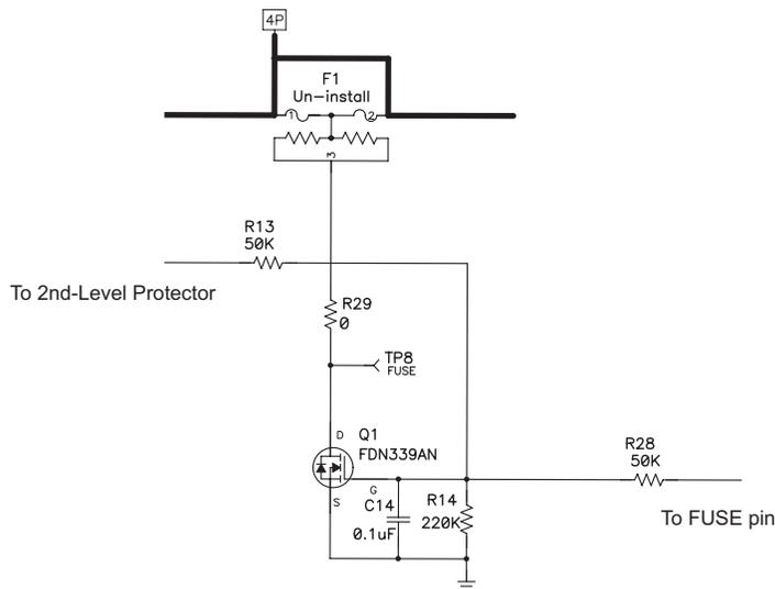
Figure 15. FUSE Circuit
