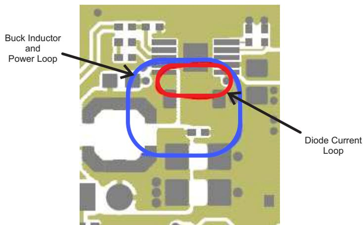
**Figure 14. DC-DC Buck Regulator Layout**
