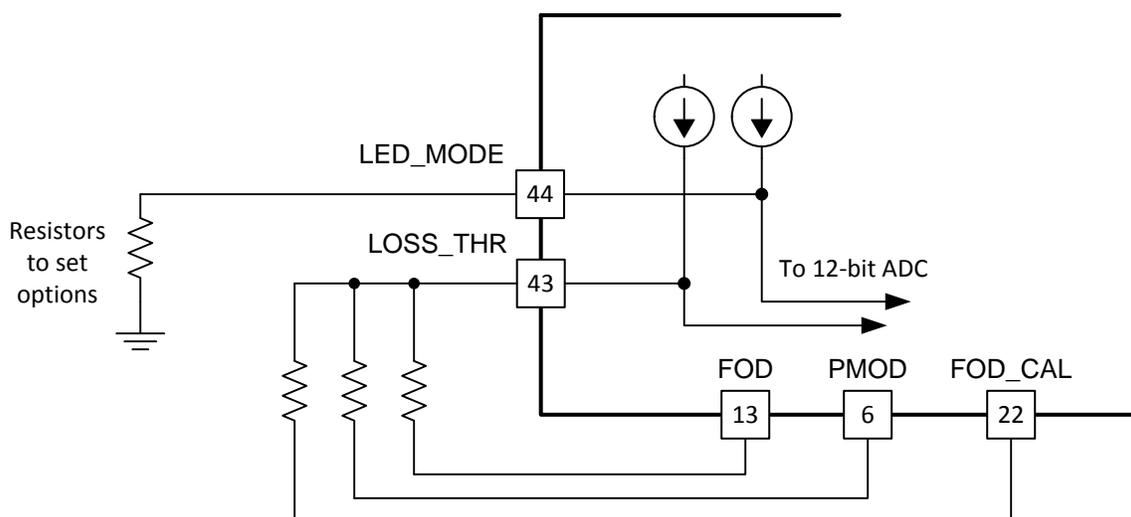
**Figure 5. Pin 43 LOSS\_THR and Pin 44 LED\_MODE Connections**
