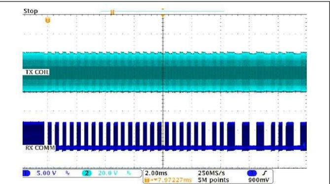
Figure 2. Typical Tx Coil and Rx Communication Signals
