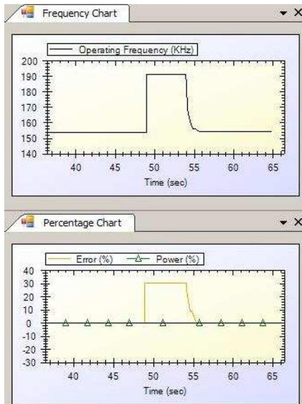
Figure 11. Qi Sniffer Capture of Frequency Shift Operation
