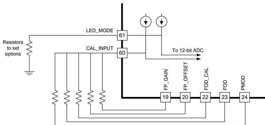
**Figure 5. Pin Connections for CAL\_INPUT and LED\_MODE**
