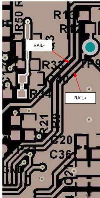
Figure 21. Balanced Differential Signal Layout
