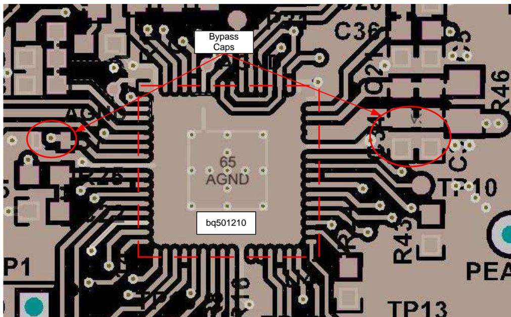
Figure 15. Bypass Capacitors Layout
