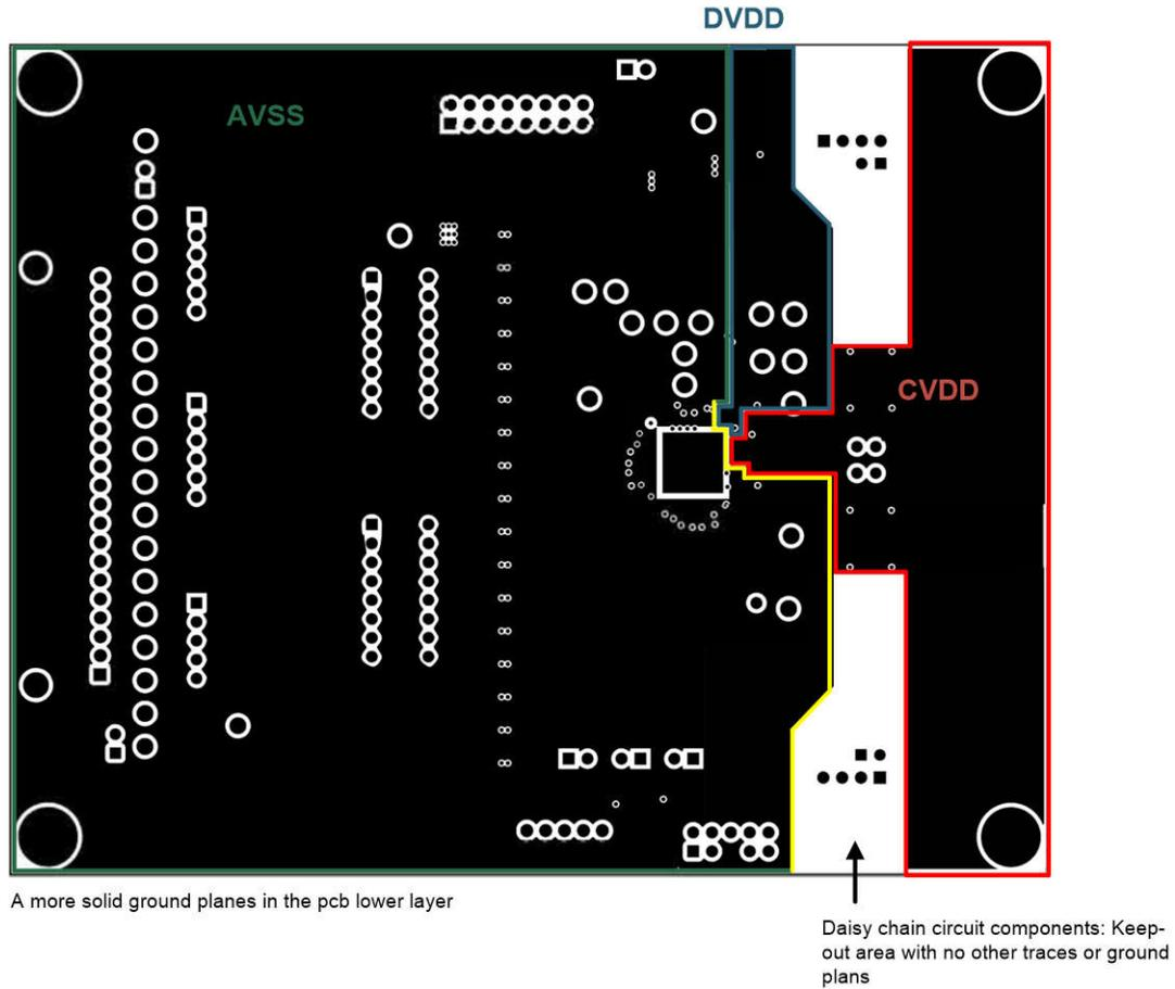
Figure 11-3. Second Layer with Solid, Separate Ground Planes
