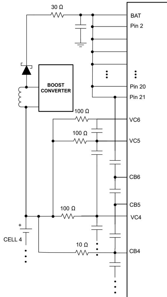
For 4S applications, short NC pins to BAT Pin and short VC5-6 to VC4
