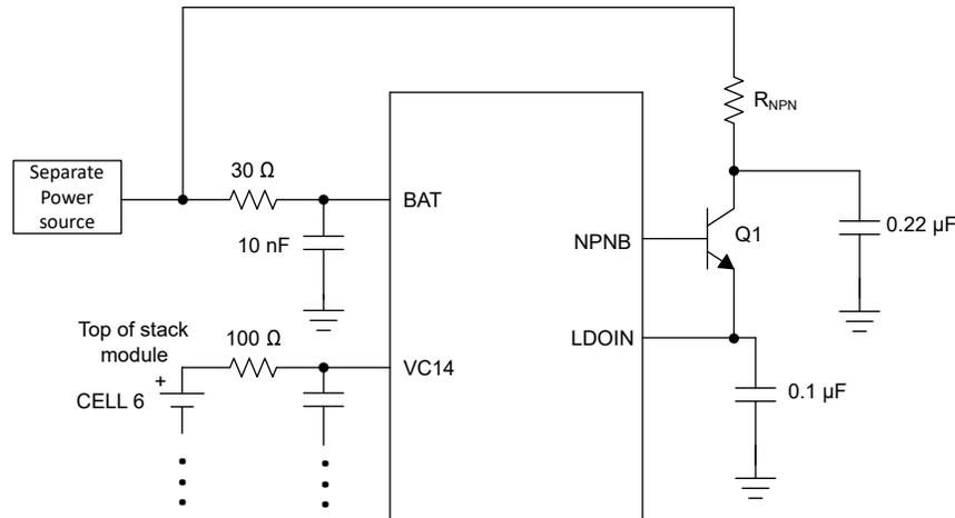
**Figure 9-9. Separate Power Source to BAT**
