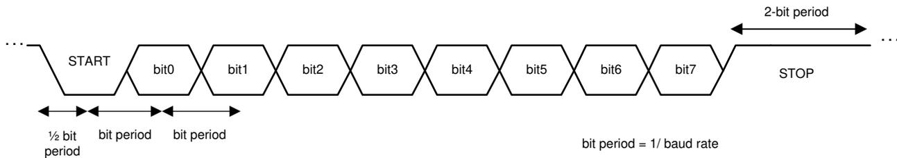
Figure 8-24. UART Response Frame with Two STOP Bits
