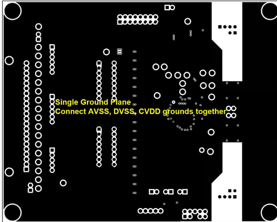
Figure 11-4. Thlrd Layer with Single Ground Plane
