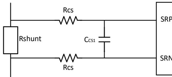
**Figure 9-12. Current Sense Input Connection**
