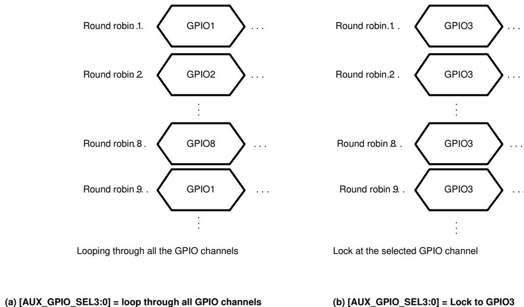
**Figure 8-10. GPIO Slot with Different *[AUX\_GPIO\_SEL3:0]* Setting**
