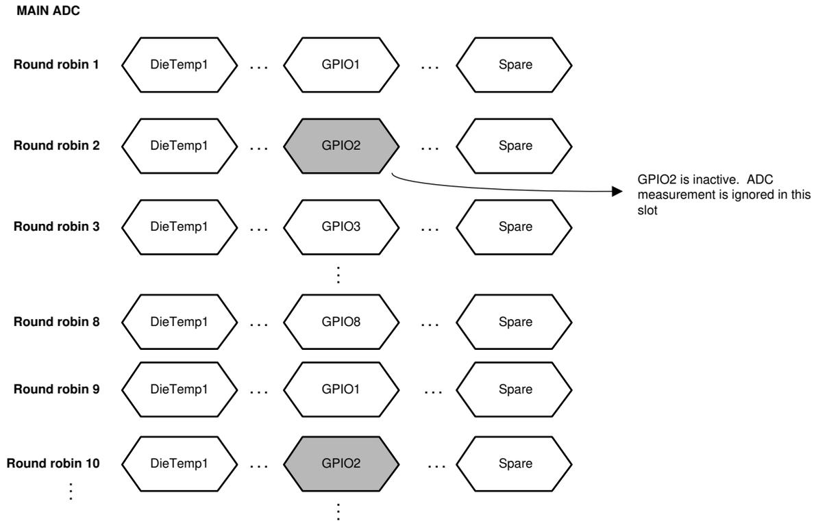
**Figure 8-6. GPIO2 Not Configured for ADC Measurement**
