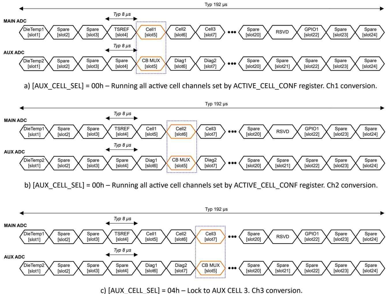
**Figure 8-11. Synchronization Between MAIN and AUX ADC Sampling**
