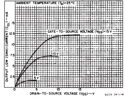
Fig. 5—Minimum n-channel output low (sink) current characteristics.
