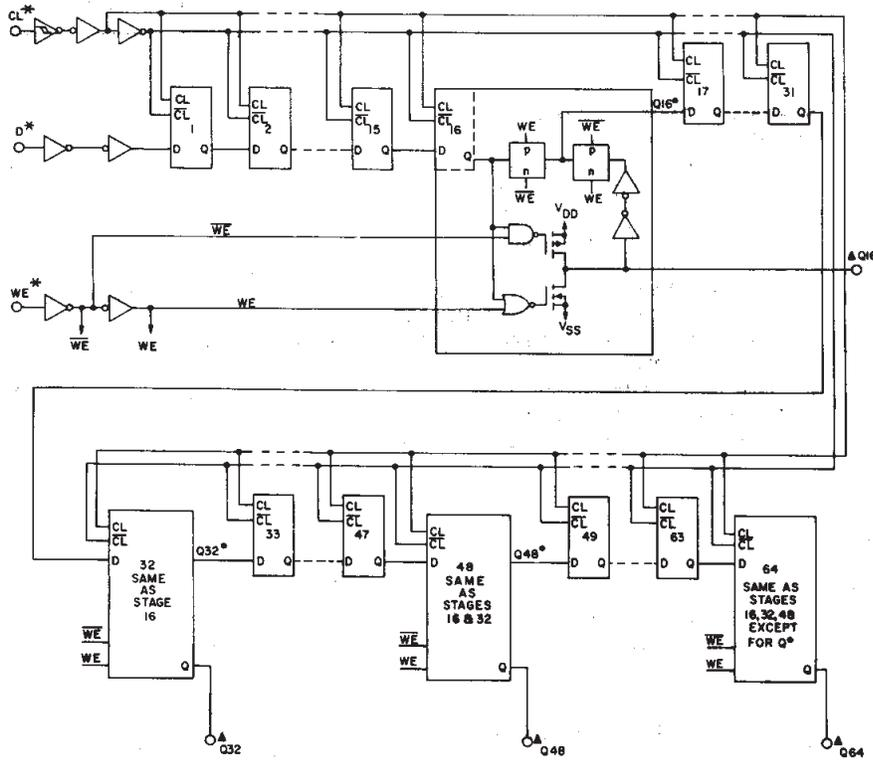
Fig. 2—CD4517B logic block diagram (one half).
