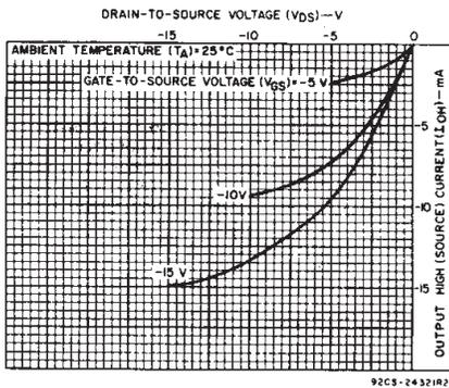
Fig. 7—Minimum p-channel output high (source) current characteristics.
