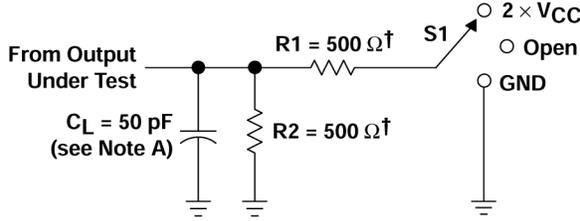
$^\dagger$  When  $V_{CC} = 1.5 \text{ V}$ ,  $R_1 = R_2 = 1 \text{ k}\Omega$
