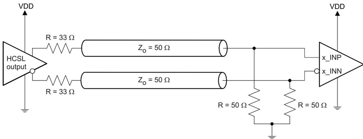
Figure 6. HCSL Input Configuration During Device Test
