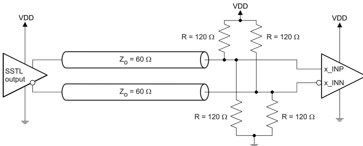
Figure 8. SSTL Input Configuration During Device Test
