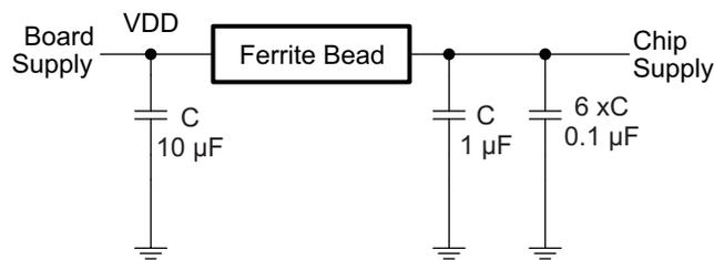
**Figure 24. Power-Supply Decoupling**
