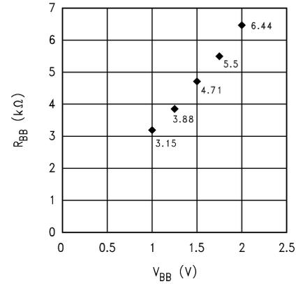
FIGURE 4.  $R_{BB}$  vs.  $V_{BB}$  for  $R_{REF} = 1.5$  k $\Omega$
