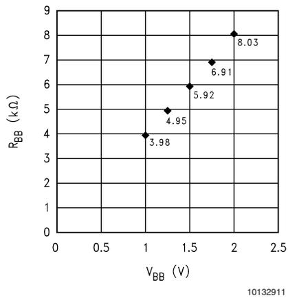
FIGURE 3.  $R_{BB}$  vs.  $V_{BB}$  for  $R_{REF} = 1.91$  k $\Omega$
