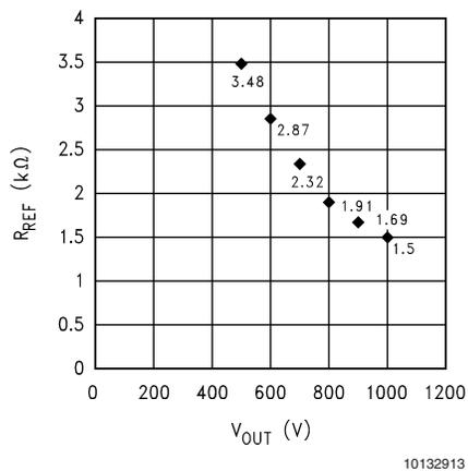
FIGURE 10. Output level's sensitivity to R<sub>REF</sub>
