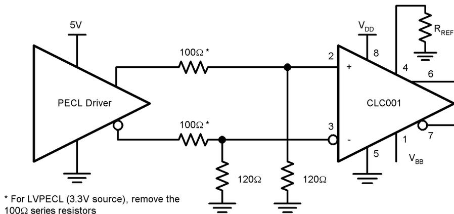
\* For LVPECL (3.3V source), remove the  $100\Omega$  series resistors
