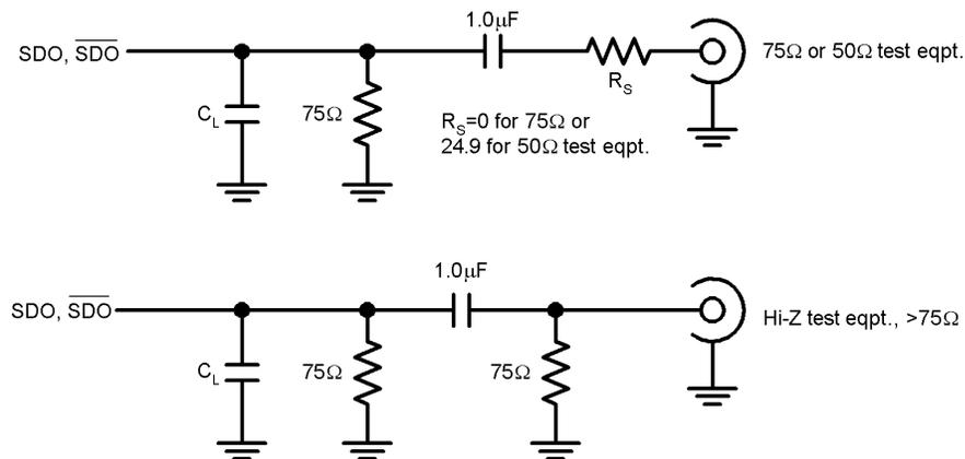
$C_L$  represents probe and test fixture capacitance and is not greater than 5pF.
