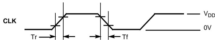
Output Rise time ( $T_r$ ) =  $(0.6 \times V_{DD})/SR1$  (or  $SR3$ )
