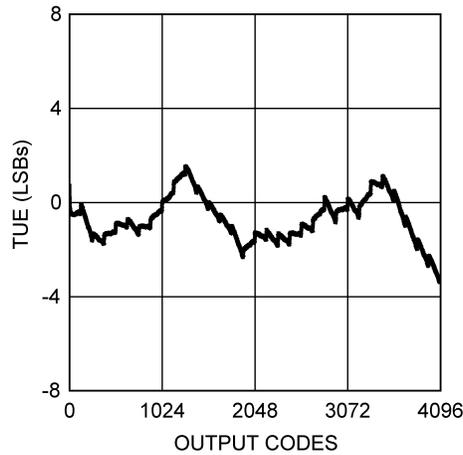
Figure 39. Total Unadjusted Error vs Output Code
