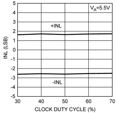
**Figure 17. 5.5-V INL vs Clock Duty Cycle**
