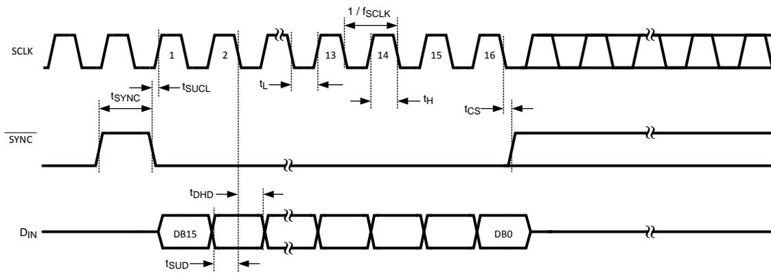
Figure 31. DAC121S101QML-SP Timing
