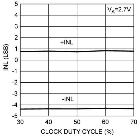
**Figure 16. 2.7-V INL vs Clock Duty Cycle**
