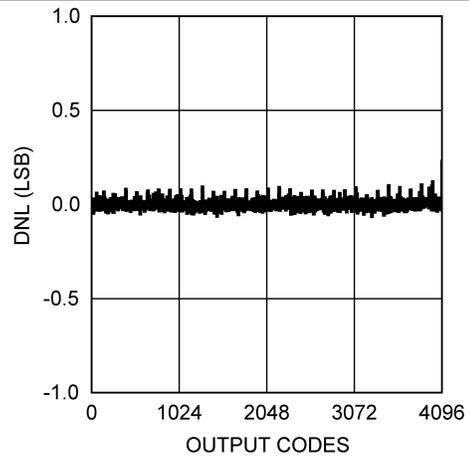
Figure 3. DNL at  $V_A = 5.5 \text{ V}$
