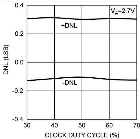
Figure 10. 2.7-V DNL vs Clock Duty Cycle
