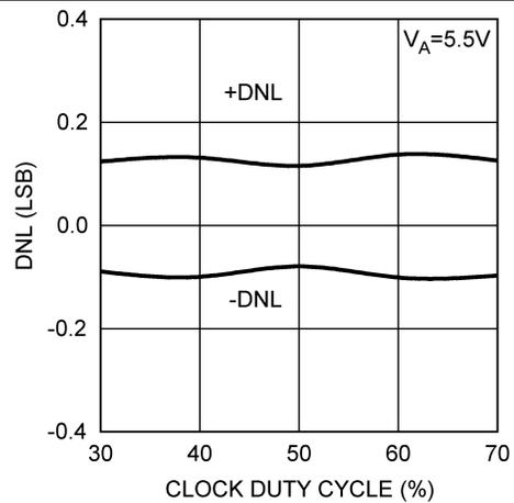
Figure 11. 5.5-V DNL vs Clock Duty Cycle
