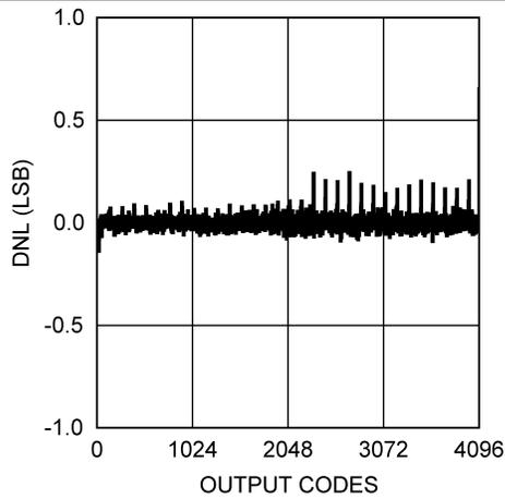
Figure 2. DNL at  $V_A = 2.7 \text{ V}$
