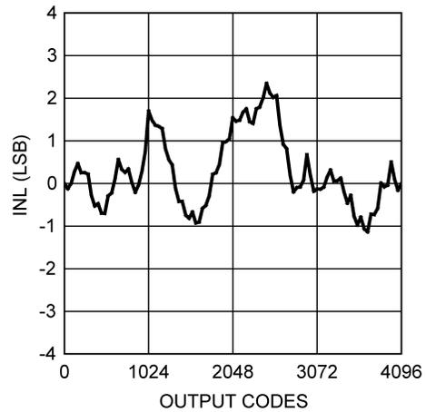
Figure 5. INL at  $V_A = 5.5 \text{ V}$
