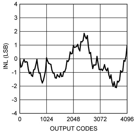
Figure 4. INL at  $V_A = 2.7 \text{ V}$
