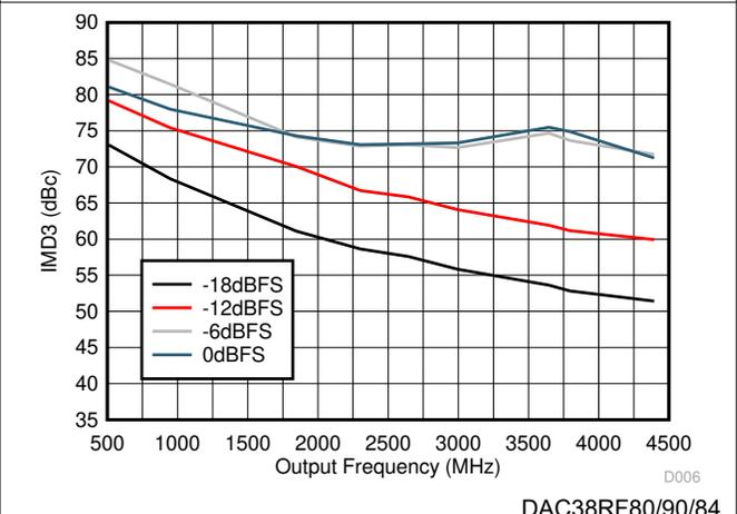
Figure 6-32. IMD3 vs Output Frequency Over Input Scale
