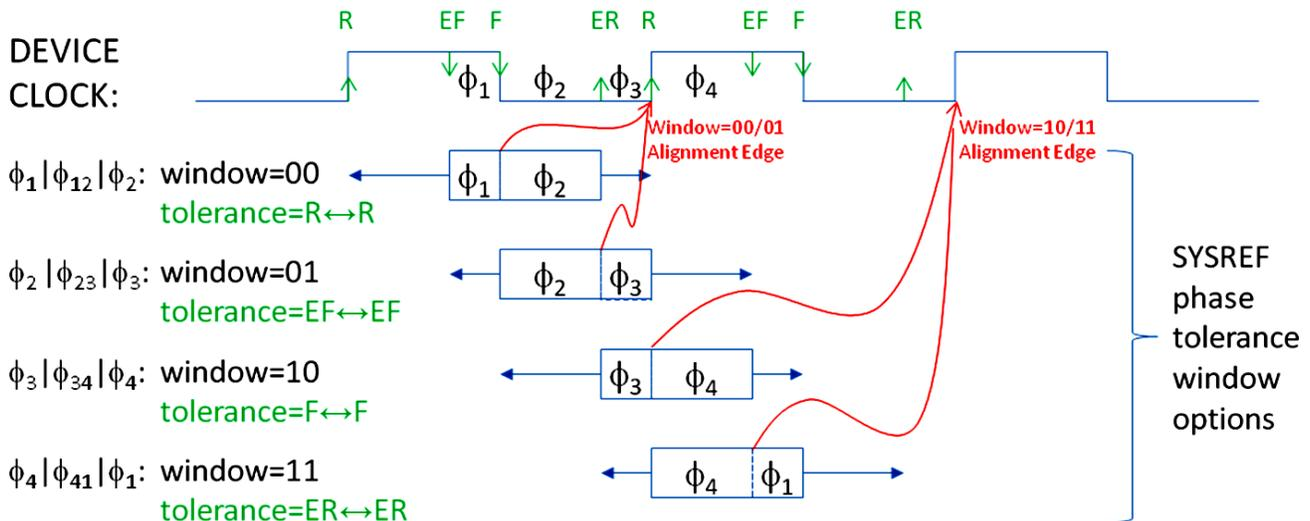
**Figure 7-11. SYSREF Capture Strategy and Phase Tolerance Windows**
