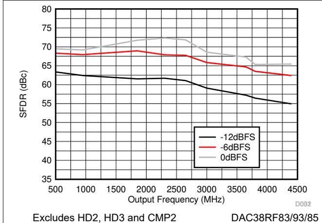
Figure 6-19. SFDR vs Output Frequency Over Input Scale
