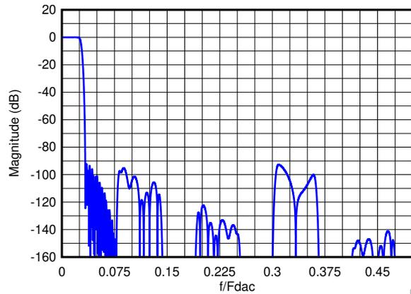
**Figure 7-19. Composite Magnitude Response for 18x Interpolation**
