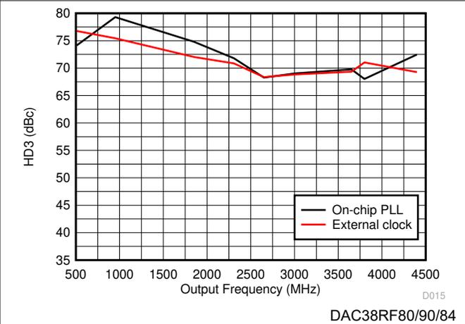
Figure 6-18. HD3 vs Output Frequency Over Clocking Option
