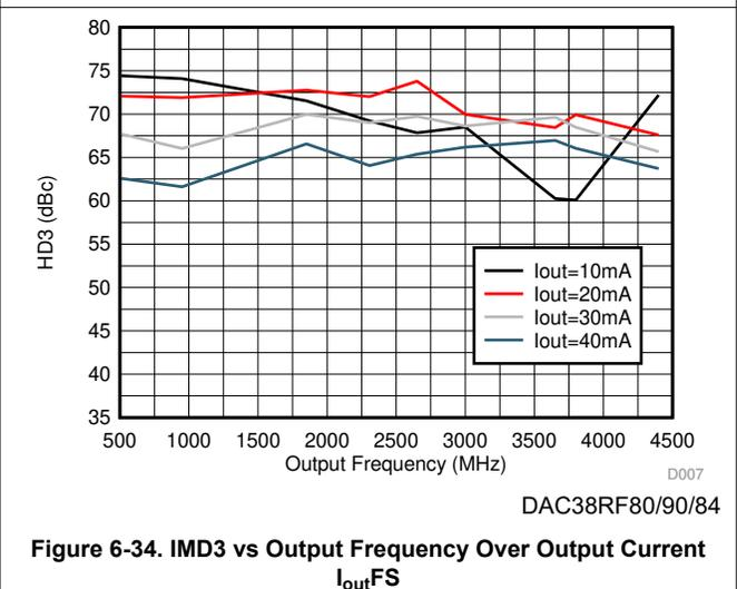
Figure 6-34. IMD3 vs Output Frequency Over Output Current  $I_{\text{outFS}}$
