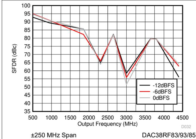
Figure 6-25. SFDR vs Output Frequency Over Input Scale
