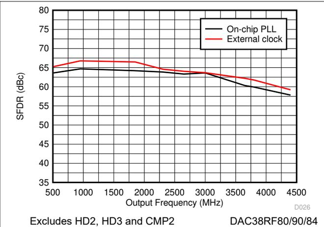
Figure 6-24. SFDR vs Output Frequency Over Cloning Option
