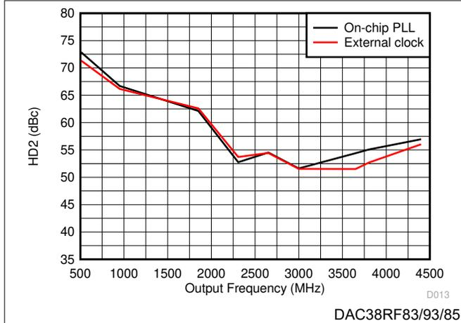
Figure 6-11. HD2 vs Output Frequency Over Clocking Option
