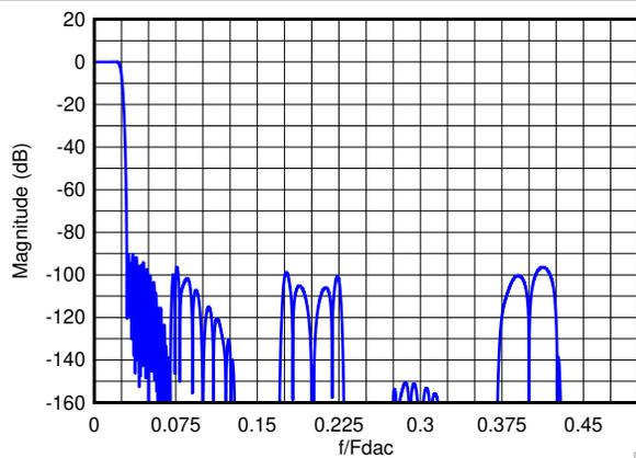
**Figure 7-20. Composite Magnitude Response for 20x Interpolation**
