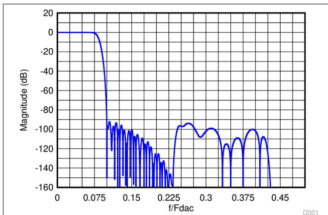
**Figure 7-14. Composite Magnitude Response for 6x Interpolation**
