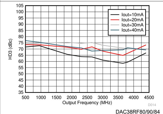
Figure 6-16. HD3 vs Output Frequency Over Output Current
