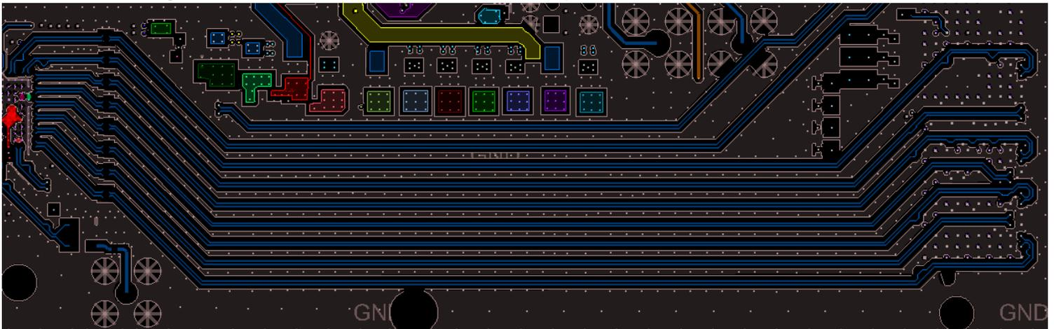
**Figure 8-10. Layout Example of High Speed SerDes Traces**
