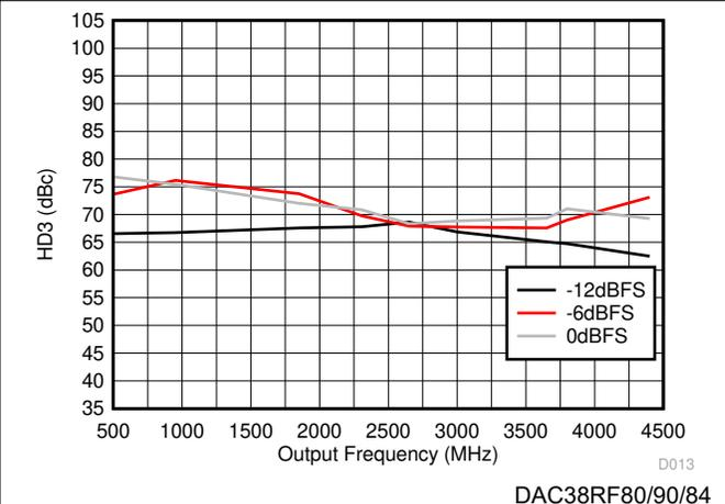
Figure 6-14. HD3 vs Output Frequency Over Input Scale
