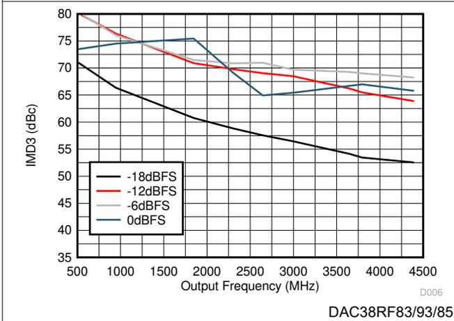
Figure 6-31. IMD3 vs Output Frequency Over Input Scale
