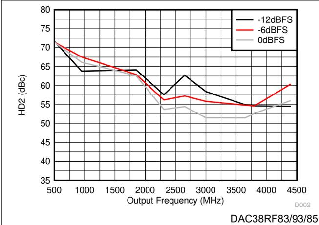
Figure 6-7. HD2 vs Output Frequency Over Input Scale
