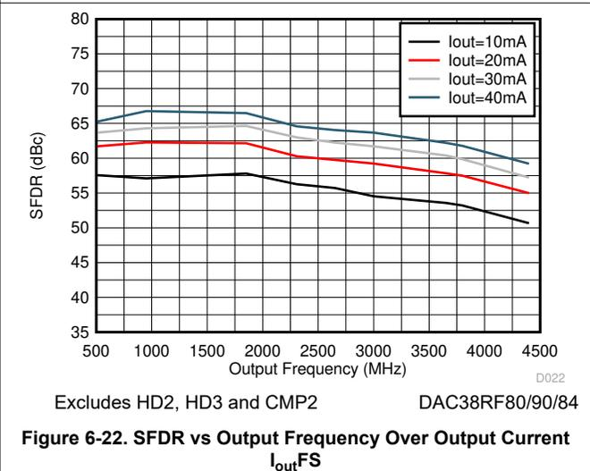
Figure 6-22. SFDR vs Output Frequency Over Output Current  $I_{\text{outFS}}$
