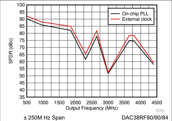
Figure 6-30. SFDR vs Output Frequency Over Clocking Option
