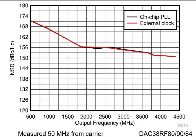
Figure 6-6. NSD vs Output Frequency Over Clocking Option
