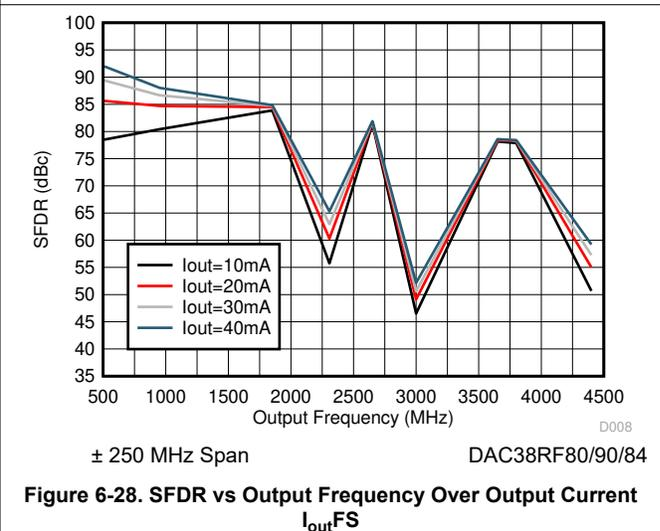
Figure 6-28. SFDR vs Output Frequency Over Output Current  $I_{\text{outFS}}$
