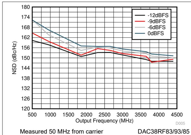
Figure 6-1. NSD vs Output Frequency Over Input Scale
