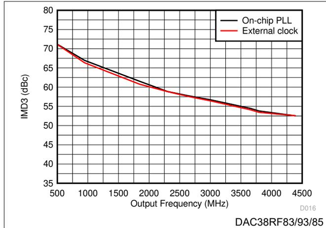
Figure 6-35. IMD3 vs Output Frequency Over Clocking Option
