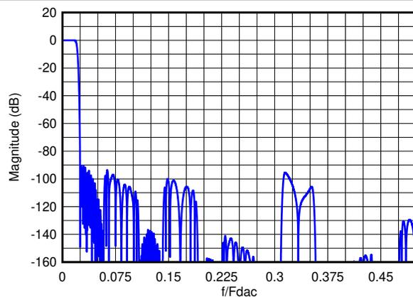
**Figure 7-21. Composite Magnitude Response for 24x Interpolation**
