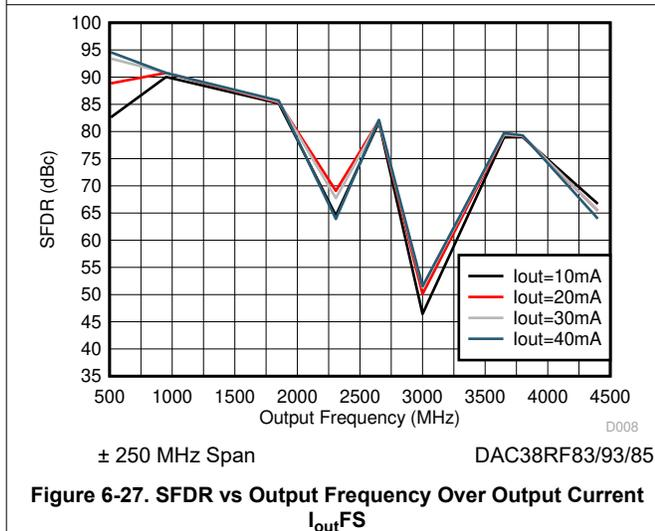
Figure 6-27. SFDR vs Output Frequency Over Output Current  $I_{\text{outFS}}$
