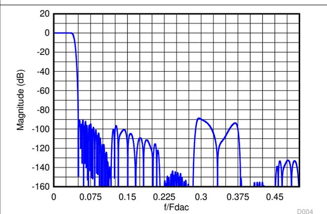
**Figure 7-17. Composite Magnitude Response for 12x Interpolation**
