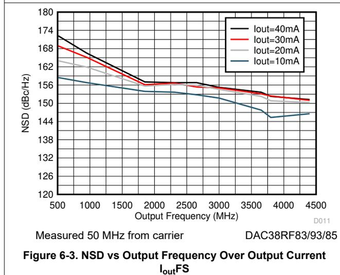
Figure 6-3. NSD vs Output Frequency Over Output Current  $I_{\text{outFS}}$
