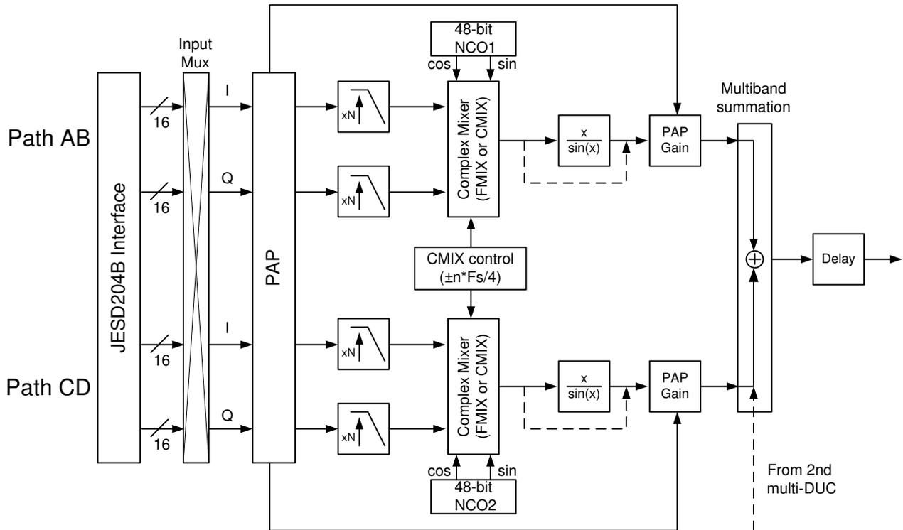
Figure 7-13. DAC38RFxx multi-DUC Signal Processing Block Diagram
