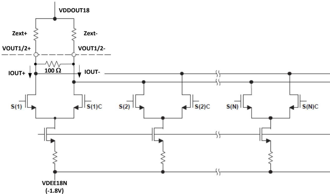
Figure 7-27. Current Steering DAC Architecture
