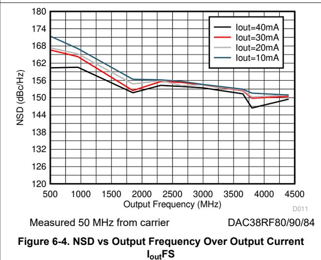
Figure 6-4. NSD vs Output Frequency Over Output Current  $I_{\text{outFS}}$
