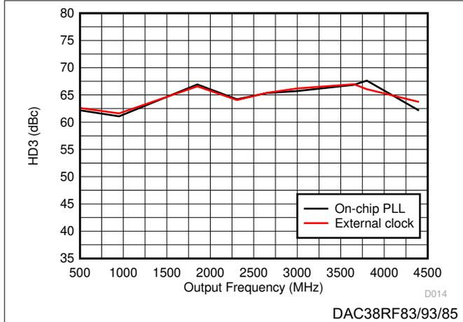
Figure 6-17. HD3 vs Output Frequency Over Clocking Option
