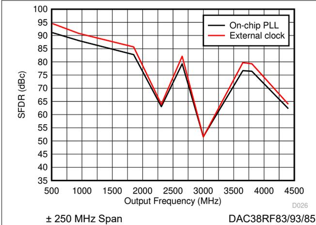
Figure 6-29. SFDR vs Output Frequency Over Clocking Option
