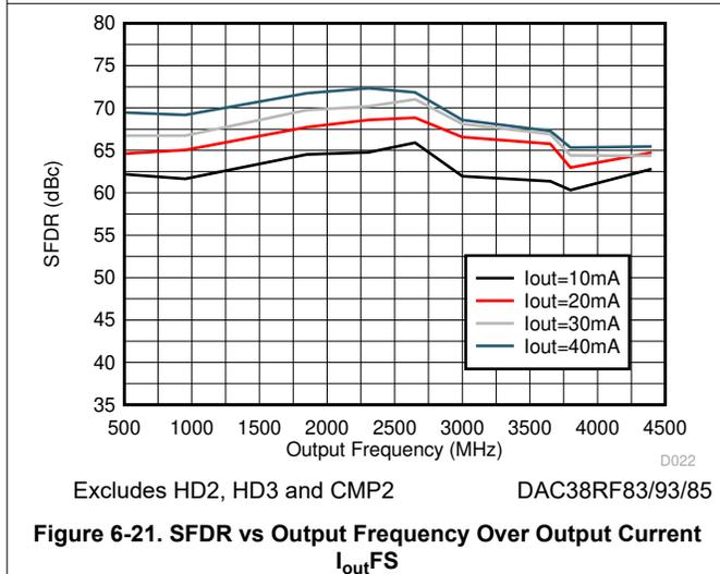
Figure 6-21. SFDR vs Output Frequency Over Output Current  $I_{\text{outFS}}$
