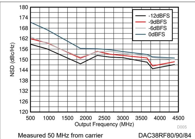
Figure 6-2. NSD vs Output Frequency Over Input Scale
