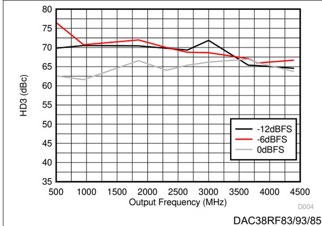
Figure 6-13. HD3 vs Output Frequency Over Input Scale
