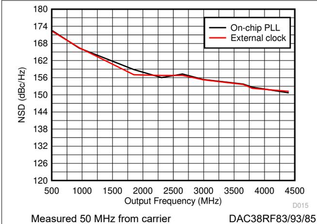
Figure 6-5. NSD vs Output Frequency Over Clocking Option
