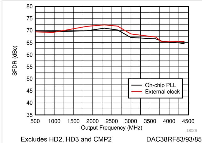
Figure 6-23. SFDR vs Output Frequency Over Cloning Option
