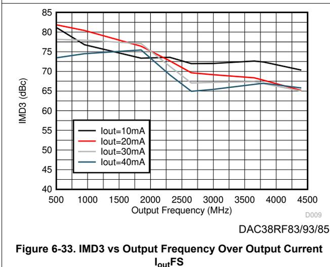
Figure 6-33. IMD3 vs Output Frequency Over Output Current  $I_{\text{outFS}}$
