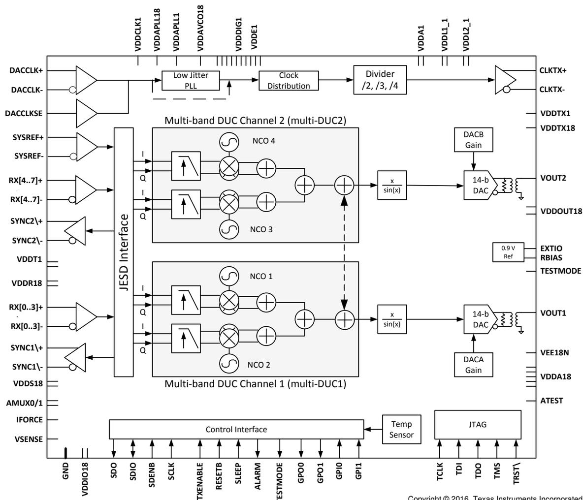
Figure 7-1. DAC38RF80 Block Diagram
