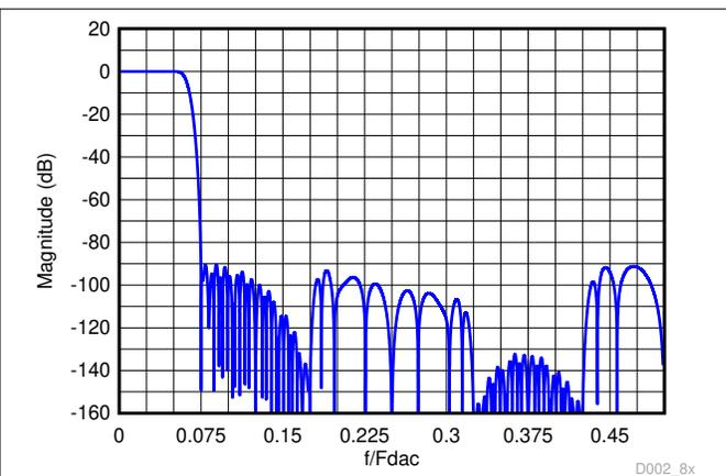
**Figure 7-15. Composite Magnitude Response for 8x Interpolation**
