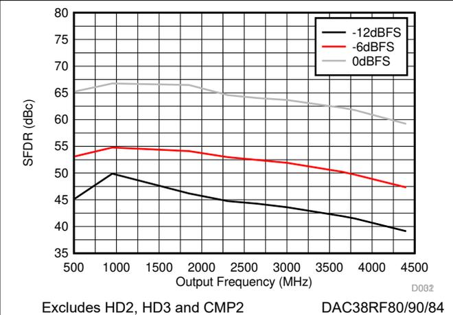
Figure 6-20. SFDR vs Output Frequency Over Input Scale
