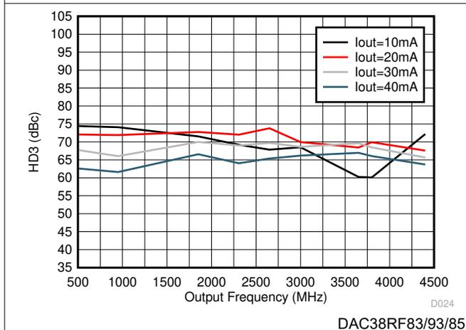
Figure 6-15. HD3 vs Output Frequency Over Output Current
