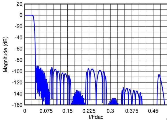
**Figure 7-18. Composite Magnitude Response for 16x Interpolation**
