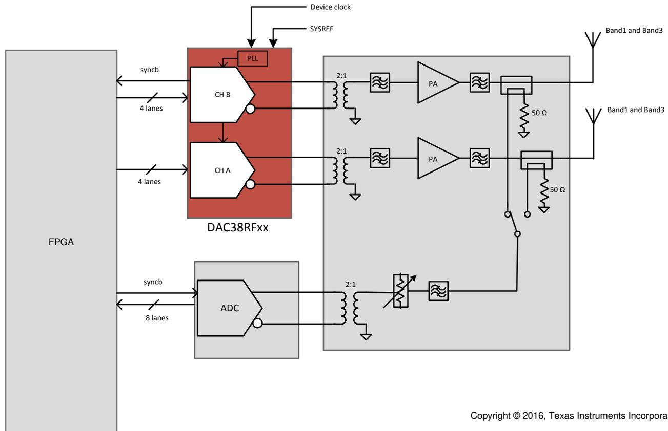
Figure 8-2. Two Antennae Multi-band Radio Frequency Transmitter
