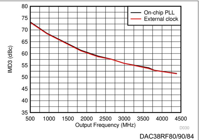
Figure 6-36. IMD3 vs Output Frequency Over Clocking Option
