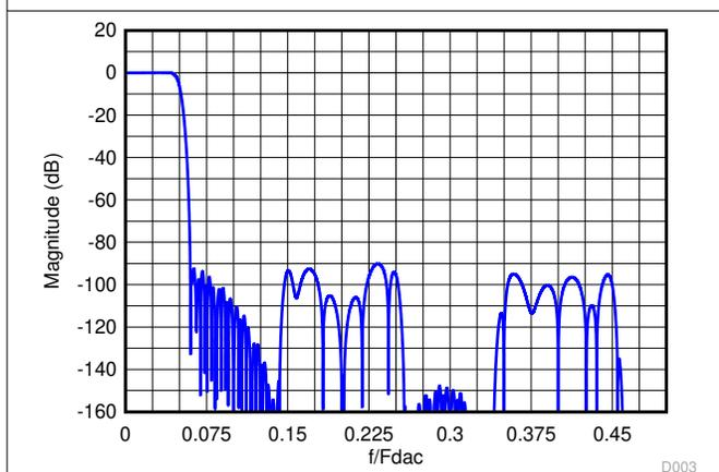
**Figure 7-16. Composite Magnitude Response for 10x Interpolation**
