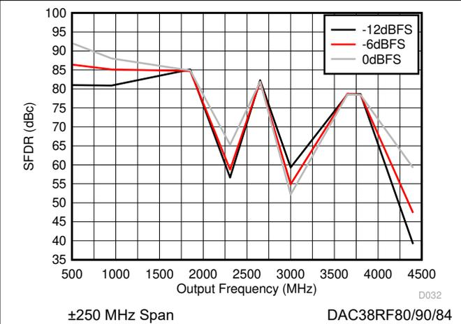
Figure 6-26. SFDR vs Output Frequency Over Input Scale
