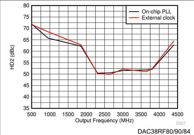
Figure 6-12. HD2 vs Output Frequency Over Clocking Option
