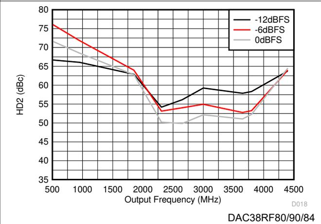
Figure 6-8. HD2 vs Output Frequency Over Input Scale
