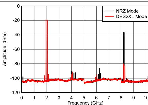
100 MHz tone spacing, includes PCB, cable and balun loss
