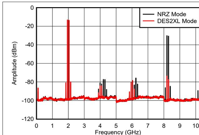
100 MHz tone spacing, includes PCB, cable and balun loss
