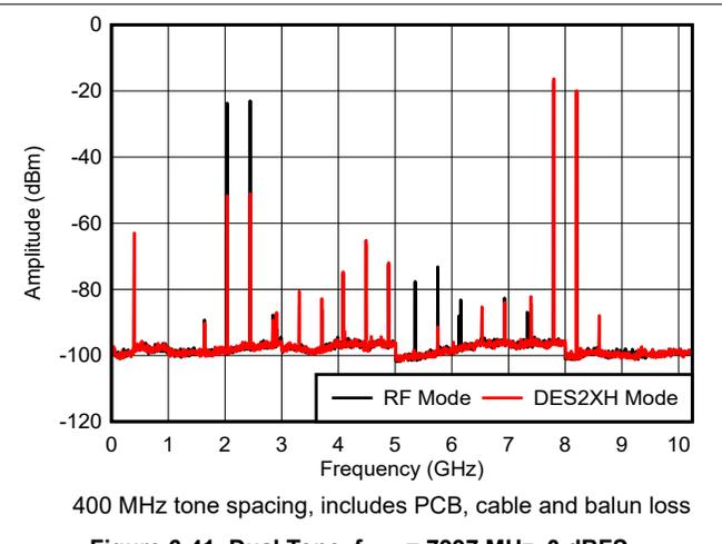
**Figure 6-41. Dual Tone,  $f_{\text{OUT}} = 7997 \text{ MHz}$ , 0 dBFS**
