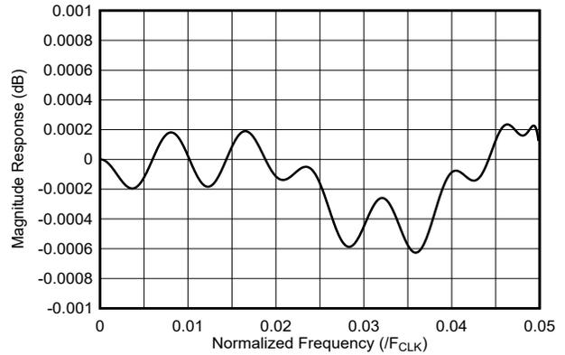
**Figure 7-23. 8x Interpolation Filter Passband Response**
