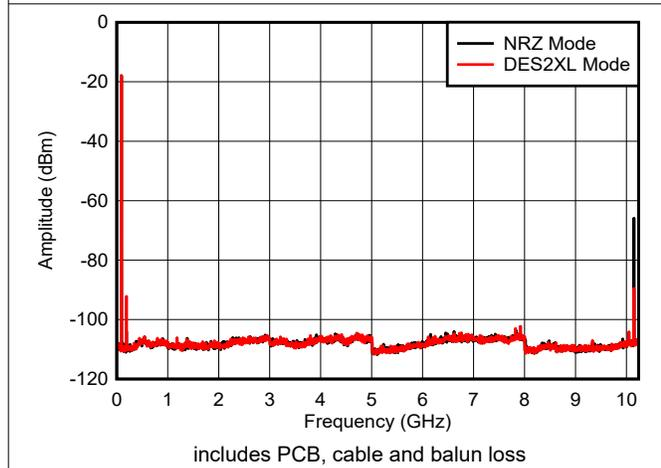
Figure 6-10.  $f_{\text{OUT}} = 97 \text{ MHz}$ , -12 dBFS
