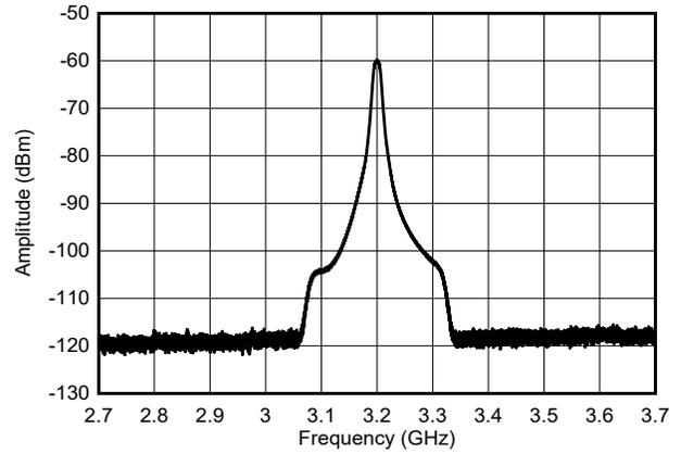
**Figure 8-18. NLFM Chirp Output Spectra across 1 GHz**
