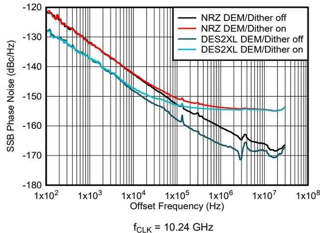
**Figure 8-5. Phase Noise vs Offset Frequency at 1 GHz**
