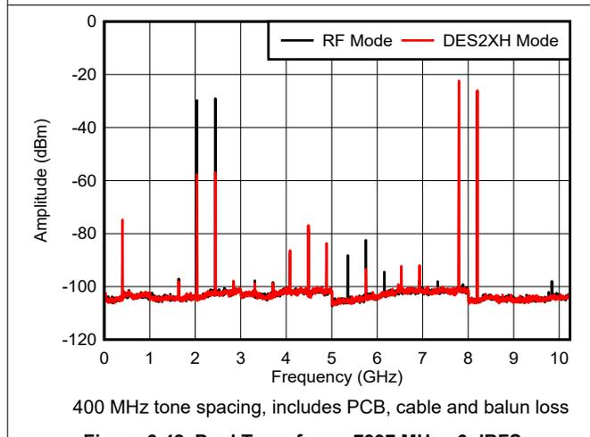
**Figure 6-42. Dual Tone,  $f_{\text{OUT}} = 7997 \text{ MHz}$ , -6 dBFS**
