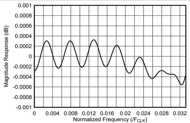
**Figure 7-25. 12x Interpolation Filter Passband Response**
