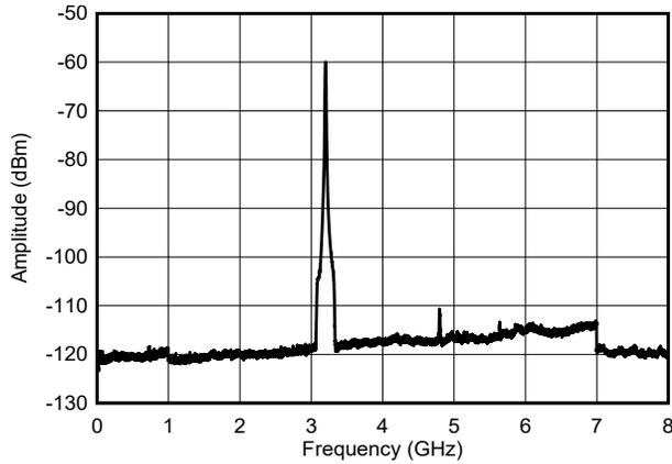
**Figure 8-17. NLFM Chirp Output Spectra across 0 - 8 GHz**
