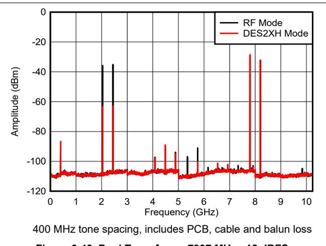
**Figure 6-43. Dual Tone,  $f_{\text{OUT}} = 7997 \text{ MHz}$ , -12 dBFS**
