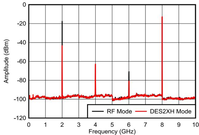
**Figure 8-4. Output Spectra Comparing DES2XH and RF Modes**
