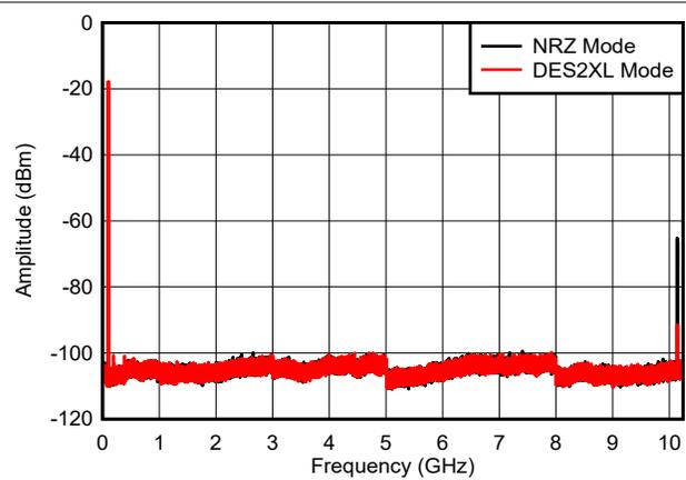
10 MHz tone spacing, includes PCB, cable and balun loss
