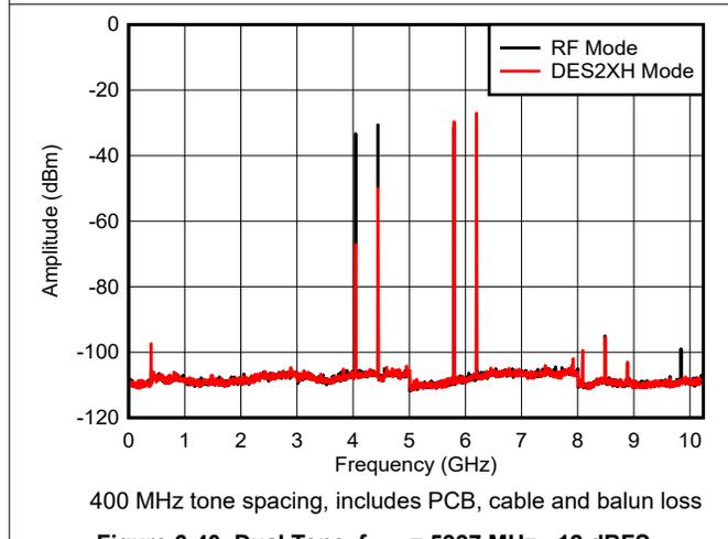
**Figure 6-40. Dual Tone,  $f_{\text{OUT}} = 5997 \text{ MHz}$ , -12 dBFS**
