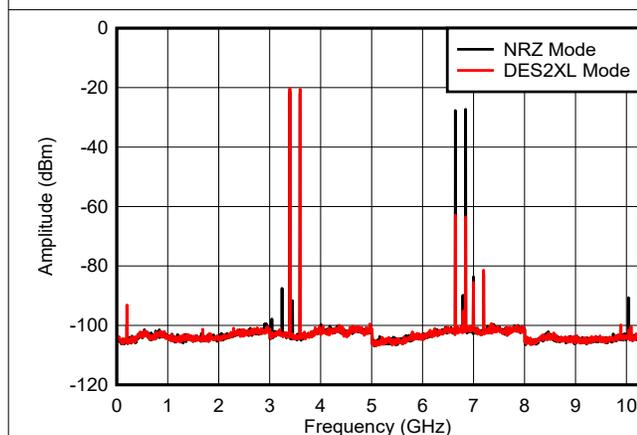
200 MHz tone spacing, includes PCB, cable and balun loss
