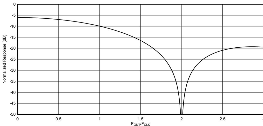
**Figure 7-6. RTZ Mode Output Frequency Response**
