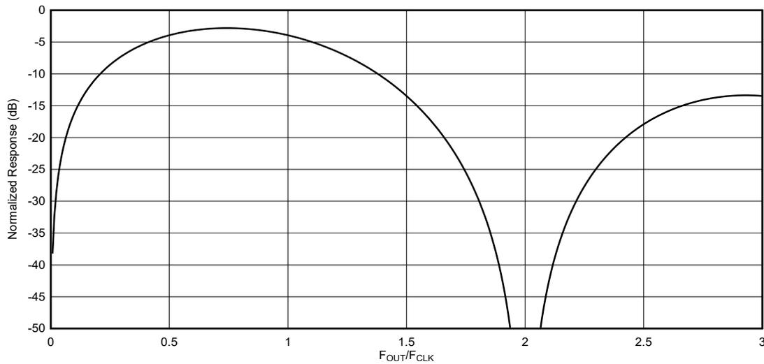
**Figure 7-8. RF Mode Output Frequency Response**
