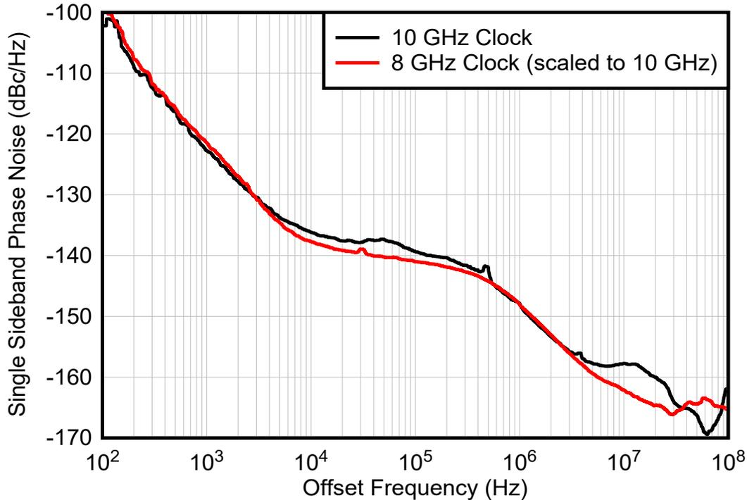
Figure 8-12. 8 GHz and 10 GHz Clock Phase Noise
