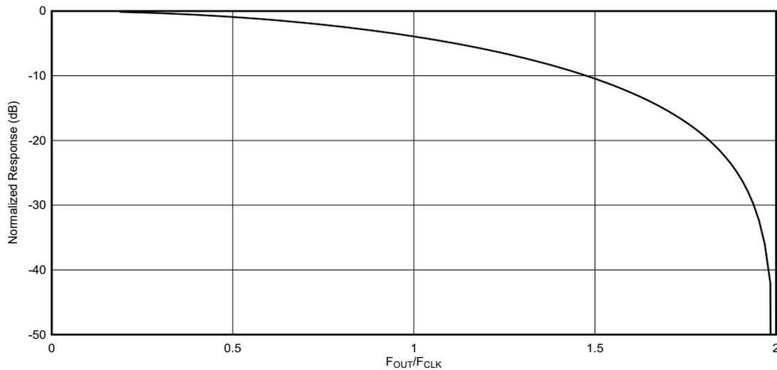
**Figure 7-10. DES1X Output Frequency Response**
