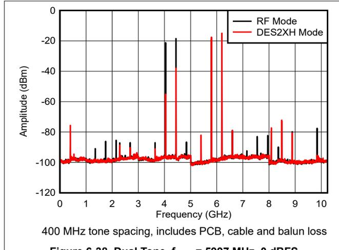
**Figure 6-38. Dual Tone,  $f_{\text{OUT}} = 5997 \text{ MHz}$ , 0 dBFS**
