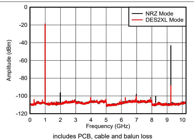
Figure 6-13.  $f_{\text{OUT}} = 997 \text{ MHz}$ , -12 dBFS
