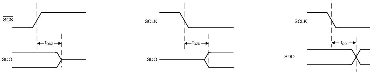
Figure 6-3. SPI Data Output Timing Diagram
