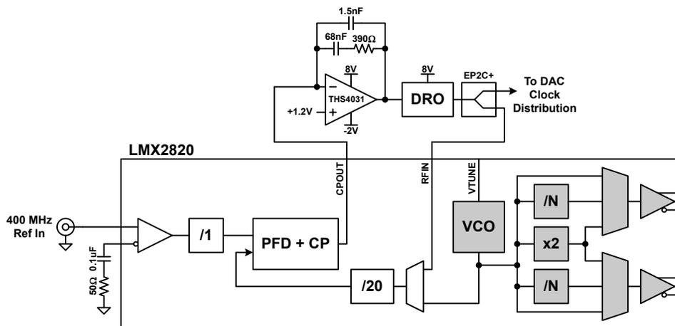
**Figure 8-8. External LMX2820 with an External VCO**
