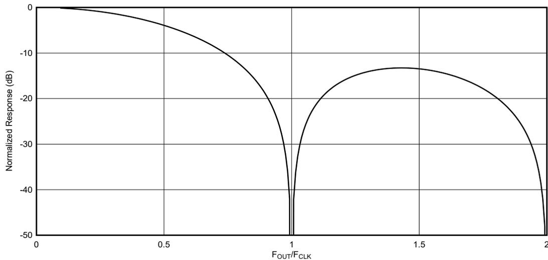
**Figure 7-4. NRZ Mode Output Frequency Response**
