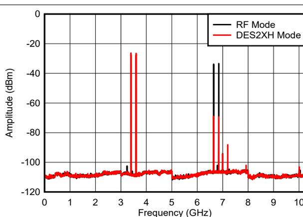
200 MHz tone spacing, includes PCB, cable and balun loss
