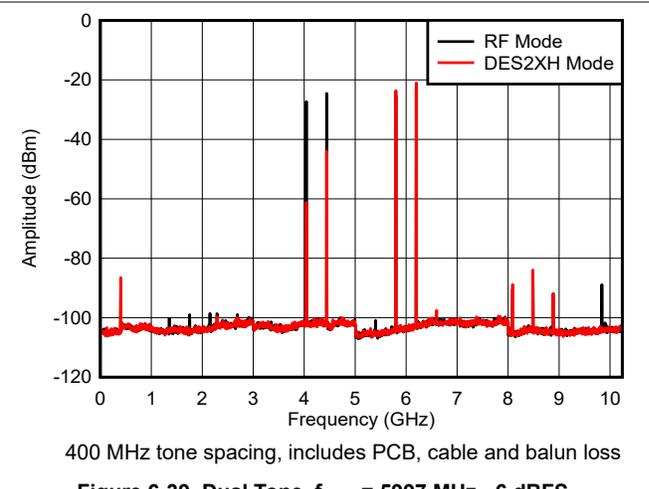
**Figure 6-39. Dual Tone,  $f_{\text{OUT}} = 5997 \text{ MHz}$ , -6 dBFS**
