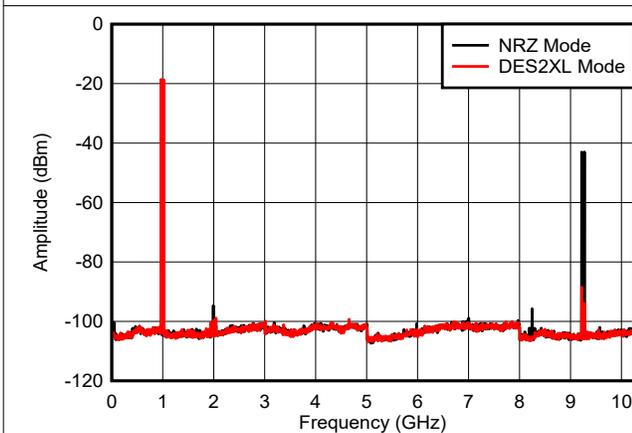
50 MHz tone spacing, includes PCB, cable and balun loss
