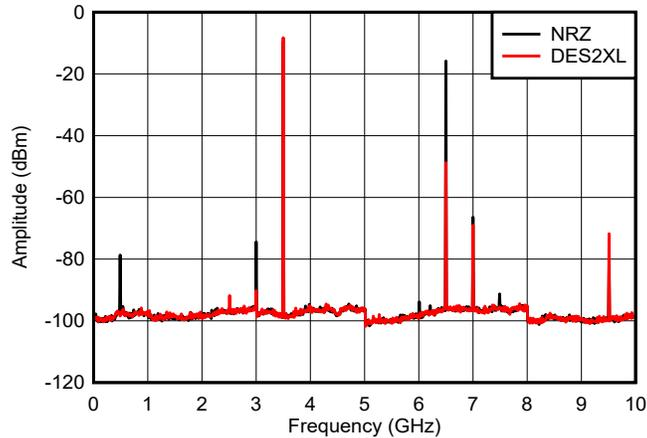
**Figure 8-3. Output Spectra Comparing DES2XL and NRZ Modes**
