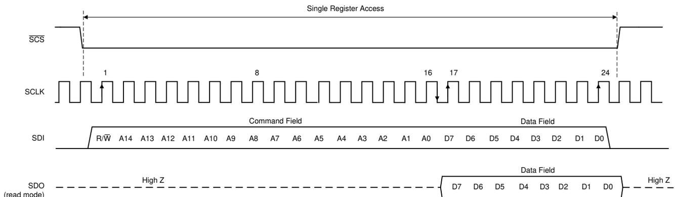
**Figure 7-58. Serial Interface Protocol: Single Read and Write**
