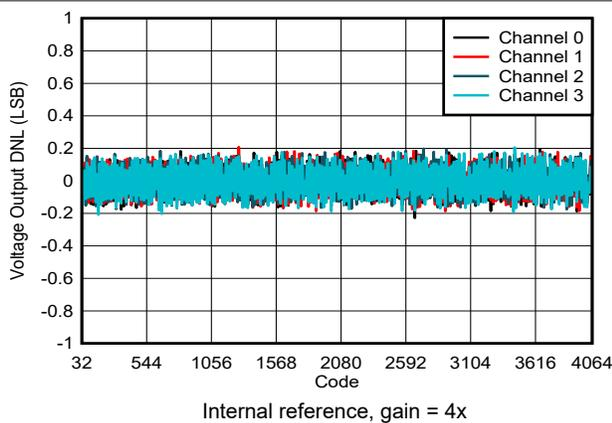
Figure 6-8. Voltage Output DNL vs Digital Input Code
