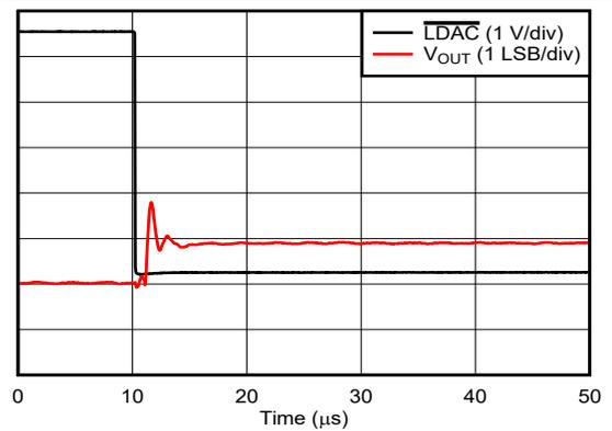
Figure 6-19. Voltage Output Code-to-Code Glitch - Rising Edge
