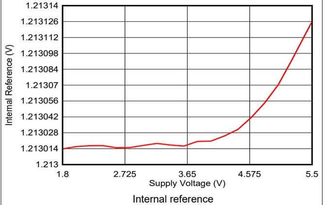
**Figure 6-55. Internal Reference vs Supply Voltage**
