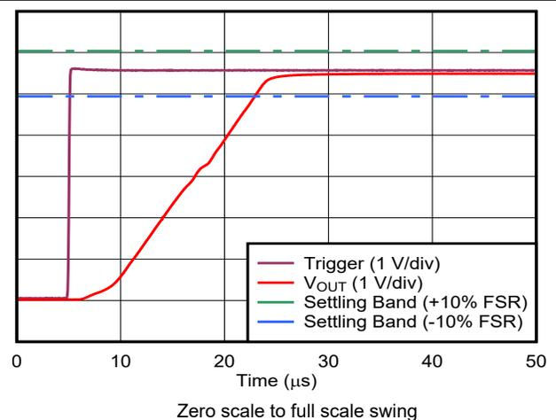
Figure 6-21. Voltage Output Setting Time - Rising Edge
