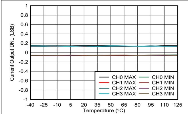
Figure 6-35. Current Output DNL vs Temperature
