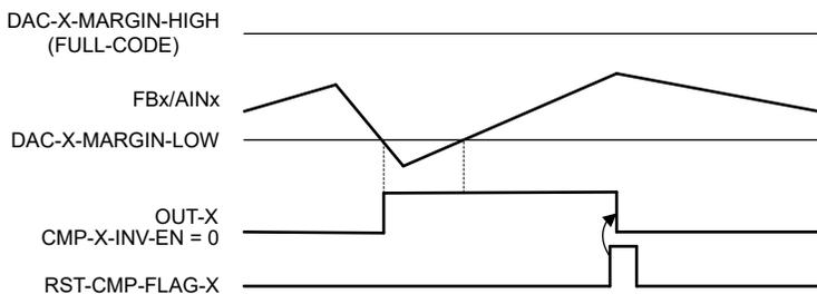
**Figure 7-7. Latching Comparator With Active High Output**
