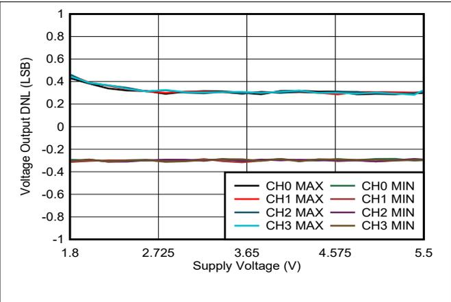
**Figure 6-11. Voltage Output DNL vs Supply Voltage**
