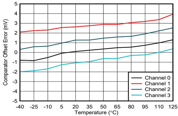
**Figure 6-53. Comparator Offset Error vs Temperature**
