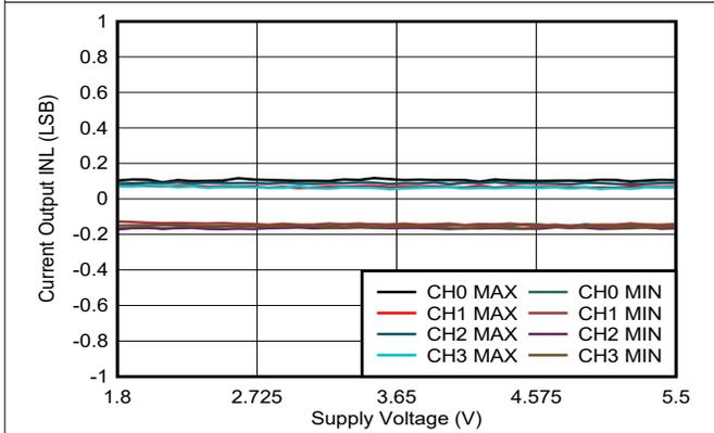
Figure 6-33. Current Output INL vs Supply Voltage
