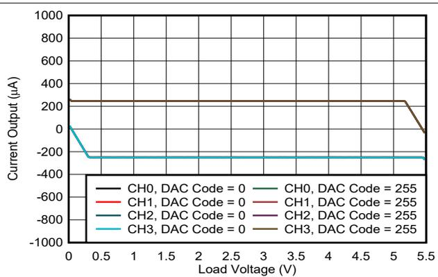
Figure 6-42. Current Output vs Load Voltage
