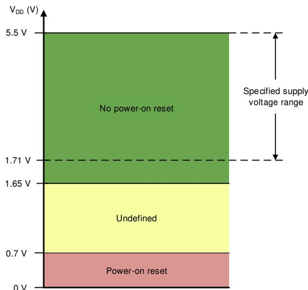
Figure 7-15. Threshold Levels for  $V_{DD}$  POR Circuit
