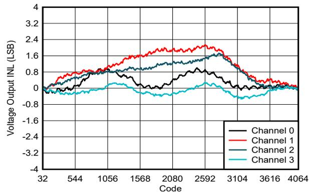
Figure 6-5. Voltage Output INL vs Digital Input Code
