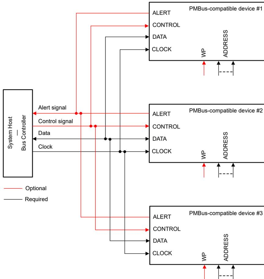
**Figure 7-11. PMBus Connections**
