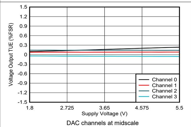
**Figure 6-15. Voltage Output TUE vs Supply Voltage**
