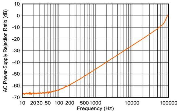
**Figure 6-30. Voltage Output AC PSRR vs Frequency**
