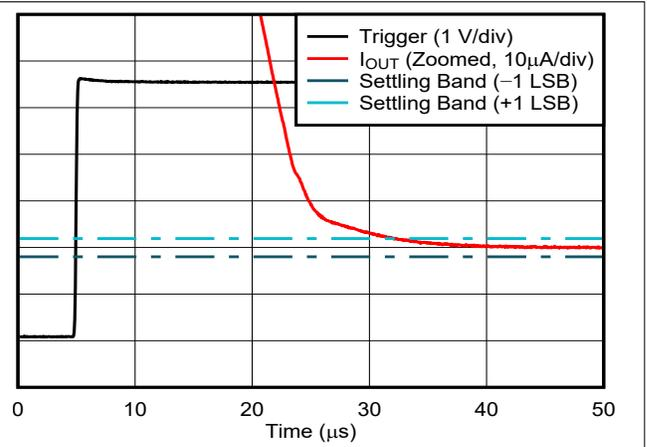
Figure 6-44. Current Output Setting Time, Falling Edge
