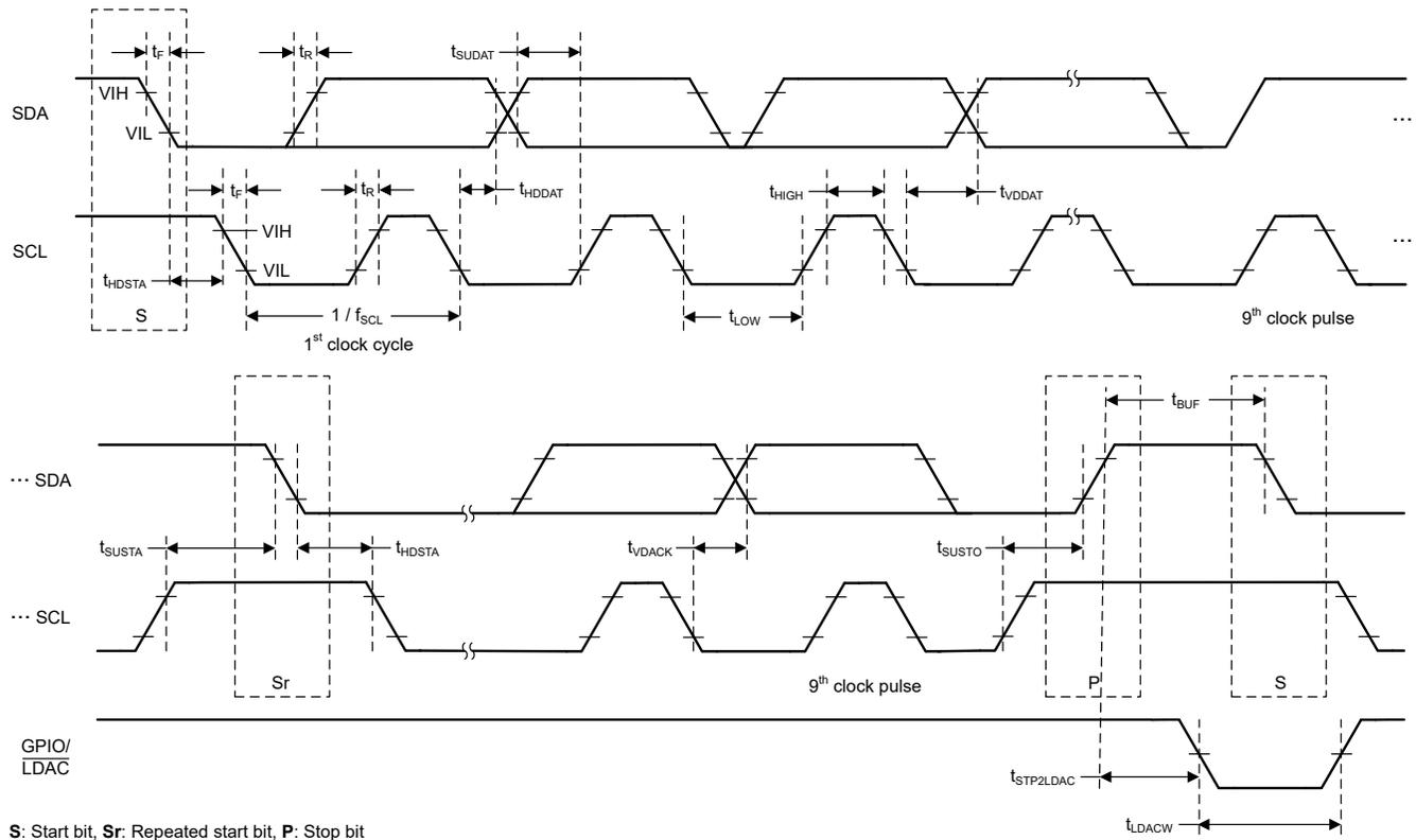
Figure 6-1. I<sup>2</sup>C Timing Diagram
