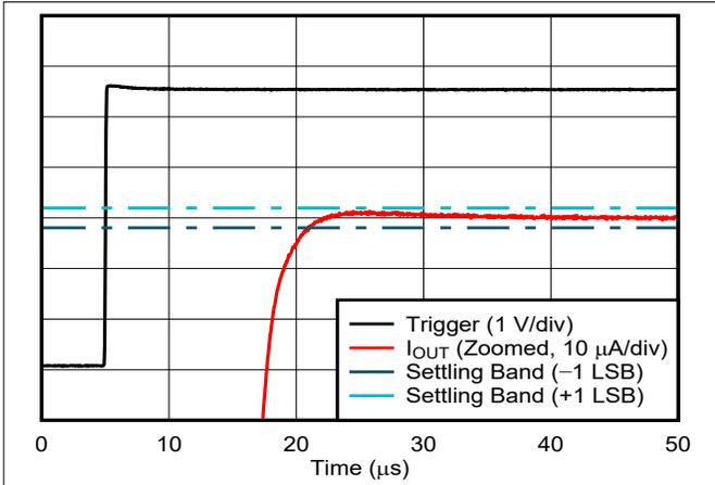
Figure 6-43. Current Output Setting Time, Rising Edge
