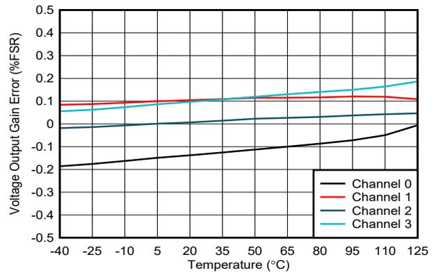
Figure 6-17. Voltage Output Gain Error vs Temperature
