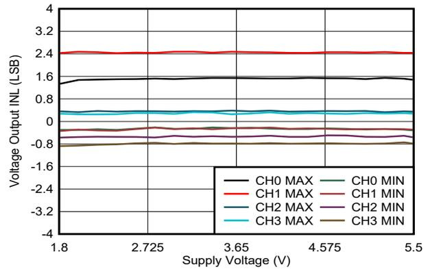
Figure 6-7. Voltage Output INL vs Supply Voltage
