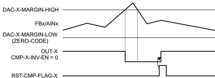
**Figure 7-6. Latching Comparator With Active Low Output**
