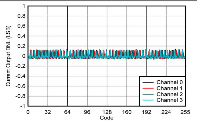
Figure 6-34. Current Output DNL vs Digital Input Code
