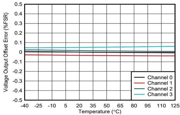
Figure 6-16. Voltage Output Offset Error vs Temperature
