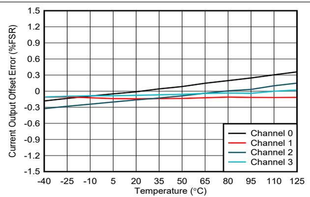
Figure 6-40. Current Output Offset Error vs Temperature
