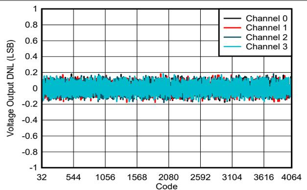
Figure 6-9. Voltage Output DNL vs Digital Input Code
