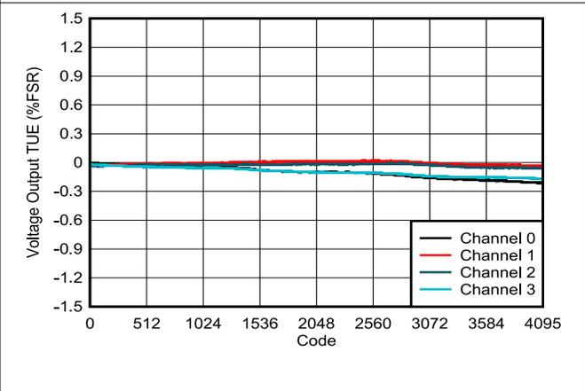
**Figure 6-13. Voltage Output TUE vs Digital Input Code**
