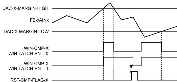
**Figure 7-8. Window Comparator Operation**
