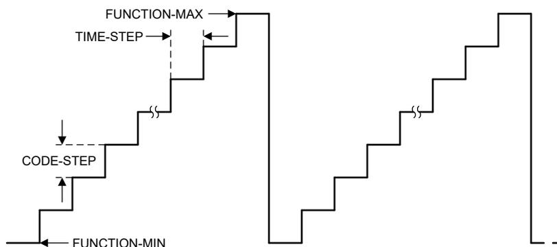
**Figure 7-13. Sawtooth Waveform**
