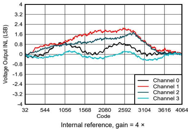
Figure 6-4. Voltage Output INL vs Digital Input Code
