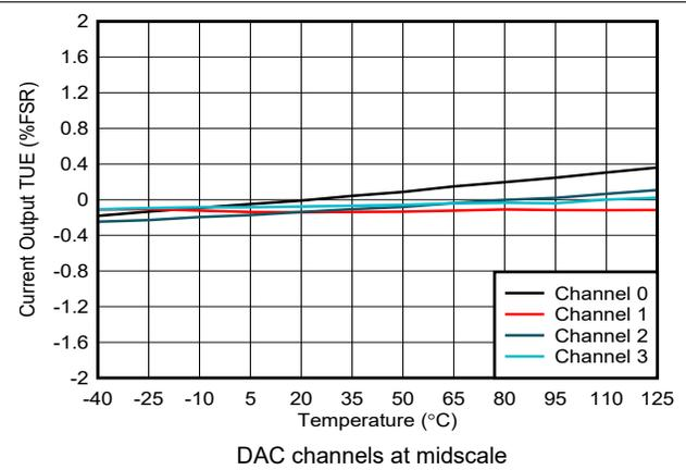
Figure 6-38. Current Output TUE vs Temperature
