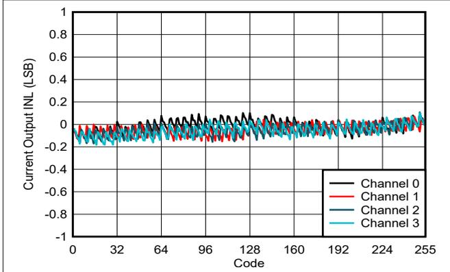
Figure 6-31. Current Output INL vs Digital Input Code
