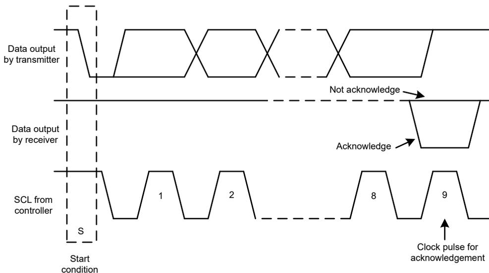
**Figure 7-20. Acknowledge and Not Acknowledge on the I<sup>2</sup>C Bus**
