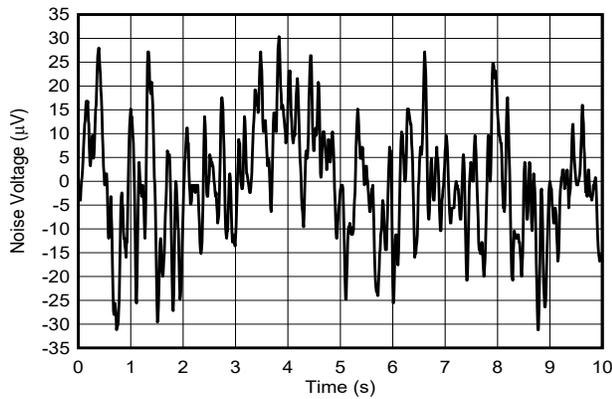
Internal reference, gain = 4 ×, f = 0.1 Hz to 10 Hz
