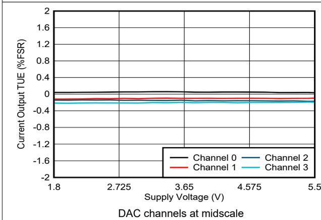
Figure 6-39. Current Output TUE vs Supply Voltage
