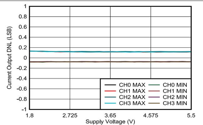
Figure 6-36. Current Output DNL vs Supply Voltage
