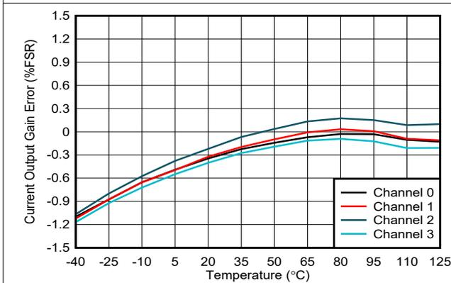
Figure 6-41. Current Output Gain Error vs Temperature
