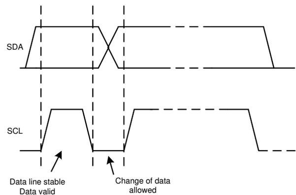
**Figure 7-22. Bit Transfer on the I<sup>2</sup>C Bus**
