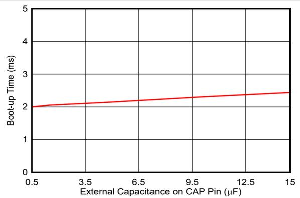
**Figure 6-57. Boot-up Time vs Capacitance on CAP pin**
