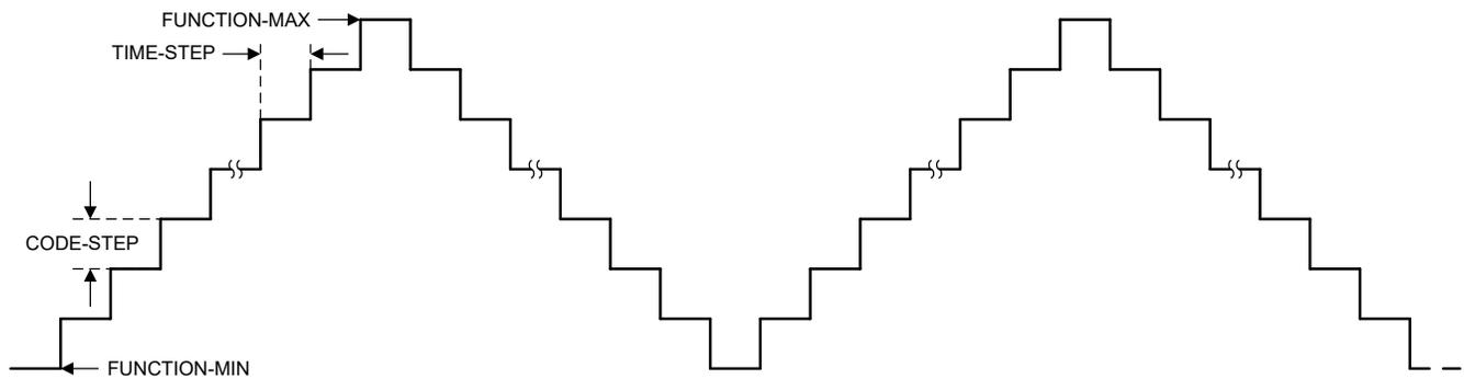
**Figure 7-12. Triangle Waveform**
