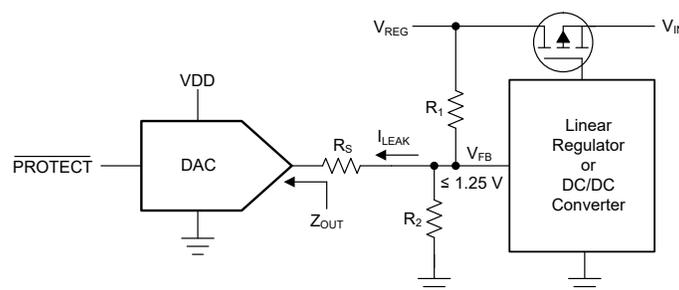
**Figure 7-9. High-Impedance (Hi-Z) Output and  $\overline{\text{PROTECT}}$  Input**
