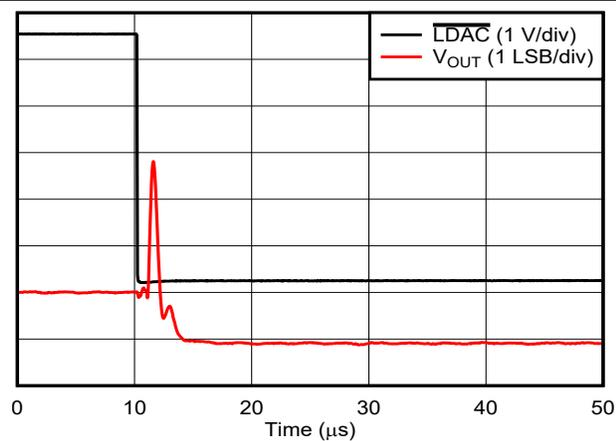
Figure 6-20. Voltage Output Code-to-Code Glitch - Falling Edge
