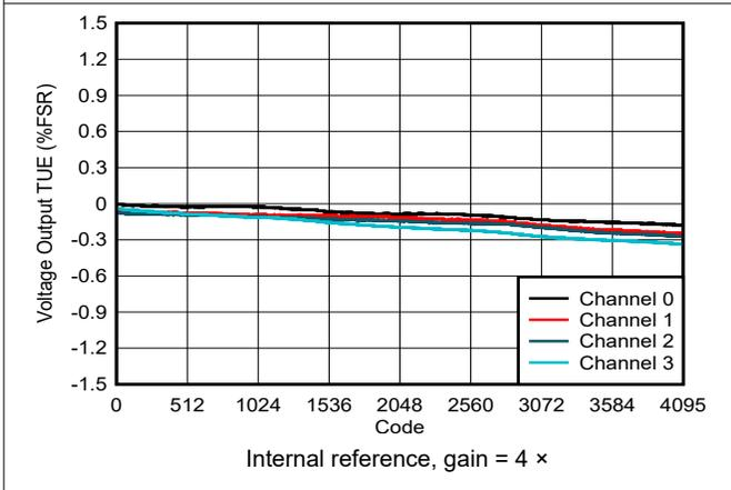
**Figure 6-12. Voltage Output TUE vs Digital Input Code**
