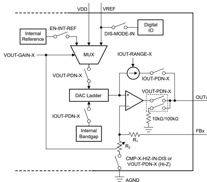
Figure 7-2. Voltage Reference Selection and Power-Down Logic
