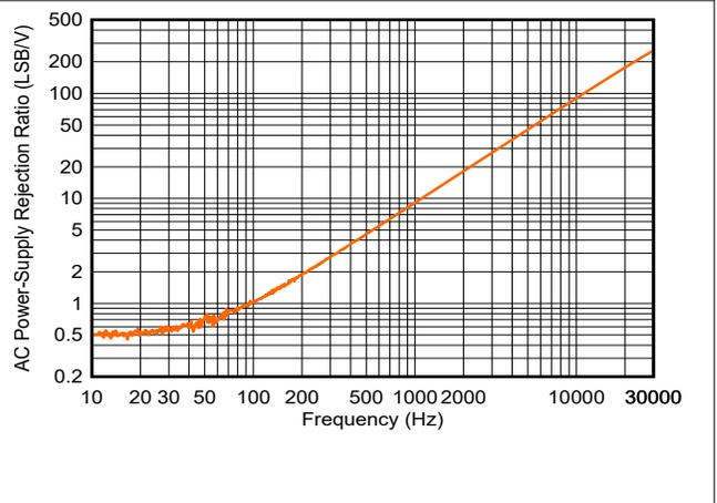
Figure 6-48. Current Output AC PSRR vs Frequency
