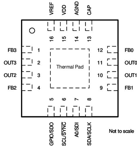
**Figure 5-1. RTE Package, 16-pin WQFN, Top View**
