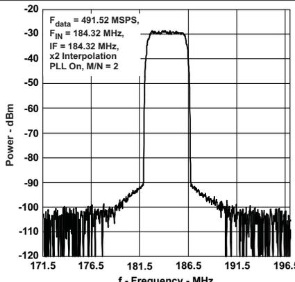
Figure 16. Single Carrier W-CDMA Test Model 1
