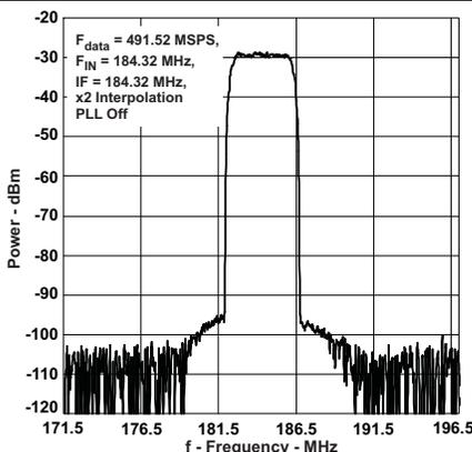
Figure 15. Single Carrier W-CDMA Test Model 1
