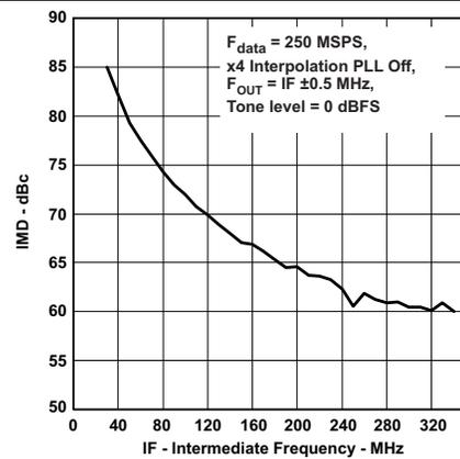
Figure 8. Two-Tone IMD vs Output Frequency
