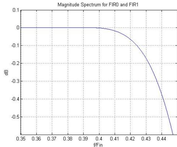
**Figure 26. FIR0 and FIR1 Transition Band**
