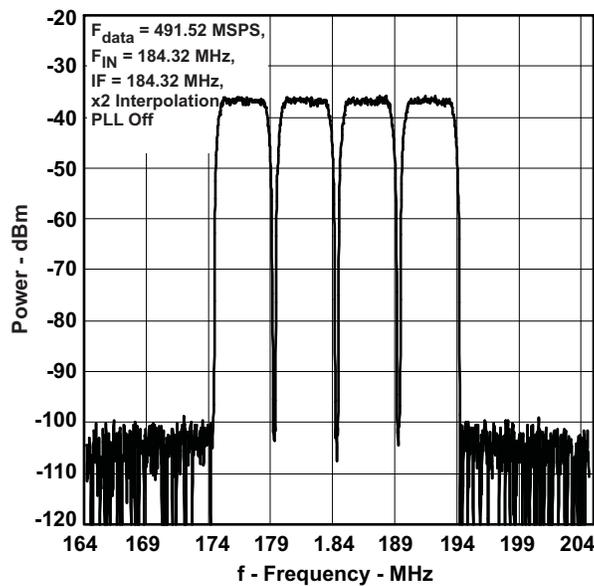
Figure 66. Four Carrier W-CDMA Test Model 1
