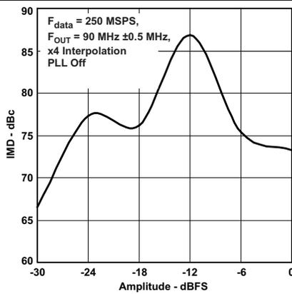
Figure 9. Two-Tone IMD vs Amplitude
