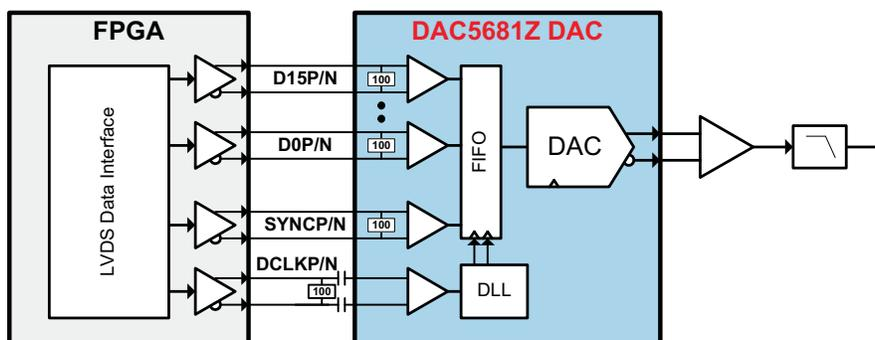
**Figure 41. System Diagram of Arbitrary Waveform Generator**
