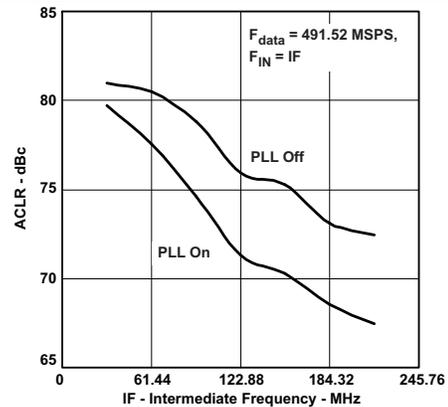
Figure 12. Single Carrier W-CDMA Test Model 1
