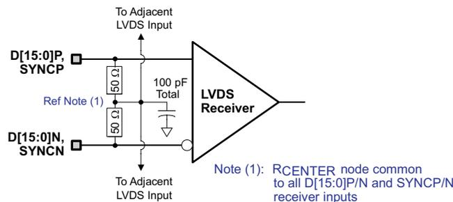
Figure 30. D[15:0]P/N and SYNC P/N LVDS Input Configuration
