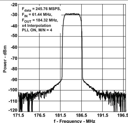
Figure 18. Single Carrier W-CDMA Test Model 1
