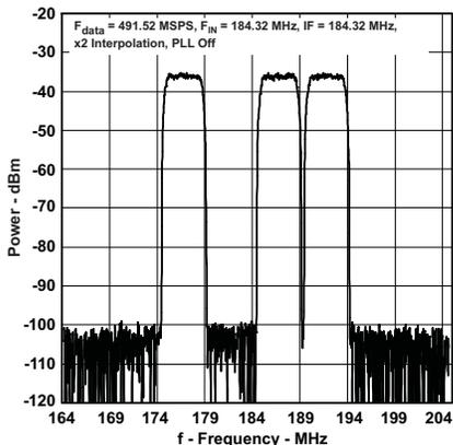
Figure 23. Three Carrier W-CDMA Test Model 1 With Gap
