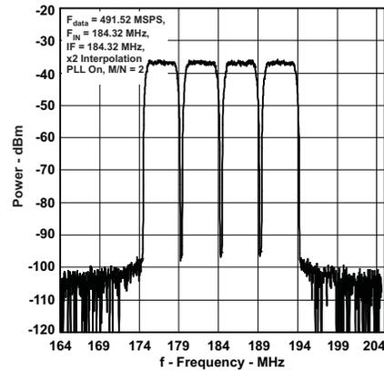
Figure 22. Four Carrier W-CDMA Test Model 1
