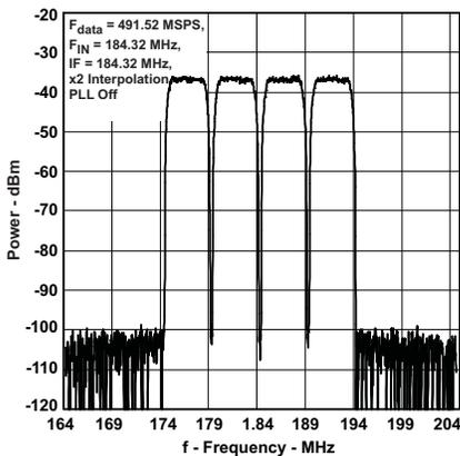
Figure 21. Four Carrier W-CDMA Test Model 1
