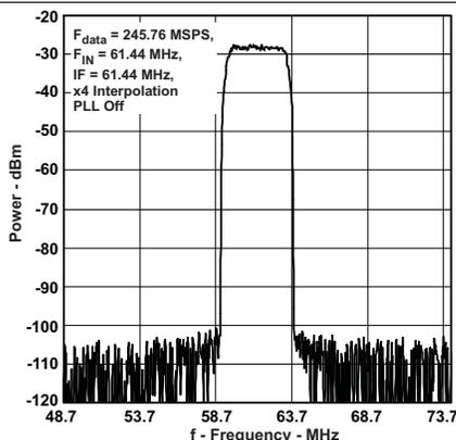
Figure 13. Single Carrier W-CDMA Test Model 1
