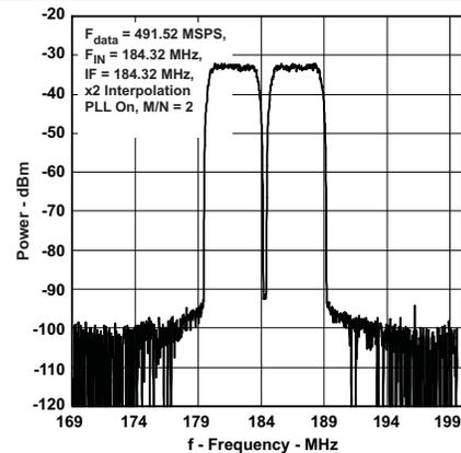
Figure 20. Two Carrier W-CDMA Test Model 1
