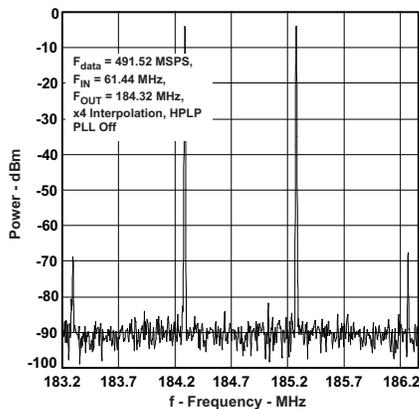
Figure 11. Two-Tone IMD Spectral Plot
