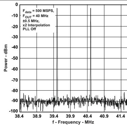
Figure 10. Two-Tone IMD Spectral Plot
