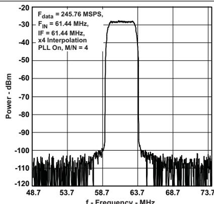
Figure 14. Single Carrier W-CDMA Test Model 1
