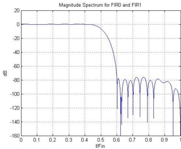
**Figure 25. Magnitude Spectrum For FIR0 and FIR1**
