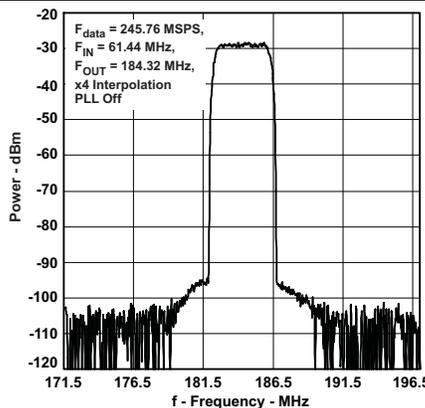
Figure 17. Single Carrier W-CDMA Test Model 1
