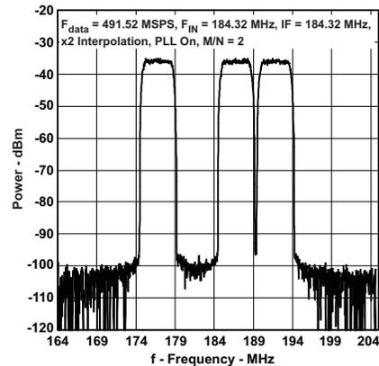
Figure 24. Three Carrier W-CDMA Test Model 1 With Gap
