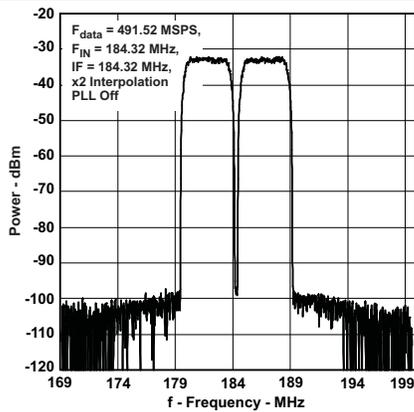
Figure 19. Two Carrier W-CDMA Test Model 1
