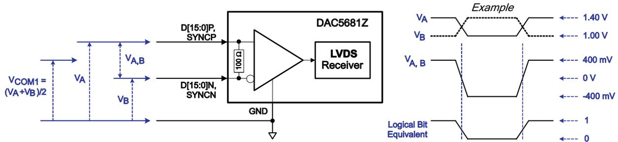
Figure 31. LVDS Data (D[15:0]P/N, SYNCN/P Pairs) Input Levels
