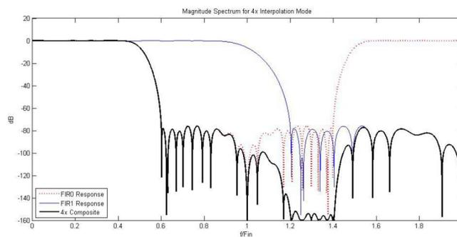
**Figure 27. Magnitude Composite Spectrum for 4x Interpolation Mode**
