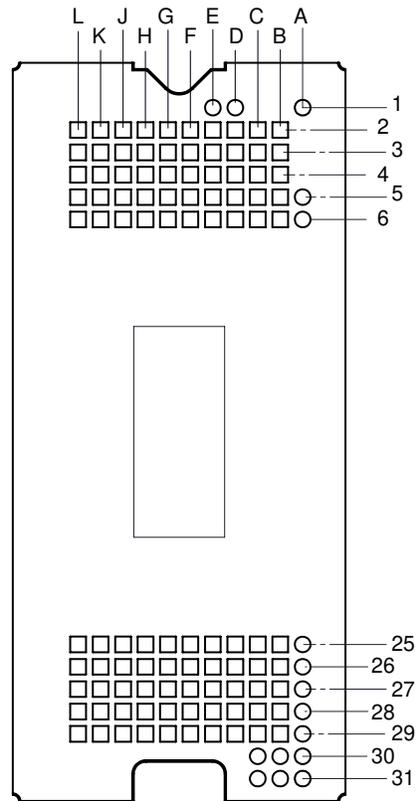
Figure 5-1. FQL Package 100-Pin LGA Bottom View
