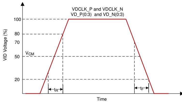
Figure 6-5. SubLVDS Input Rise and Fall Slew Rate
