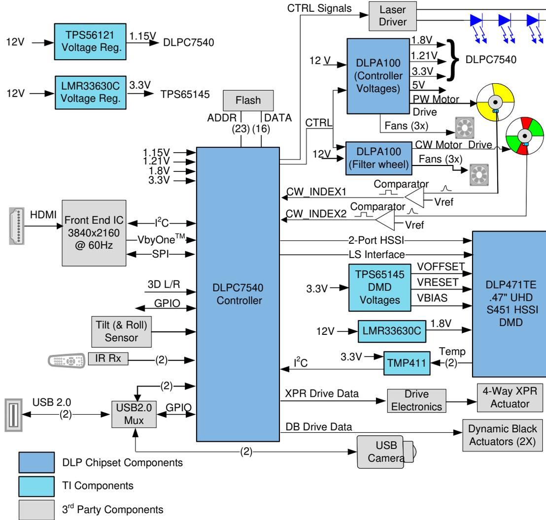
**Figure 7-1. Typical 4K UHD Laser Phosphor Application Diagram**
