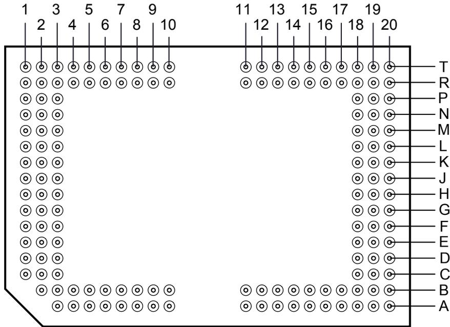
Figure 4-1. FYN Package 149-Pin PGA Bottom View
