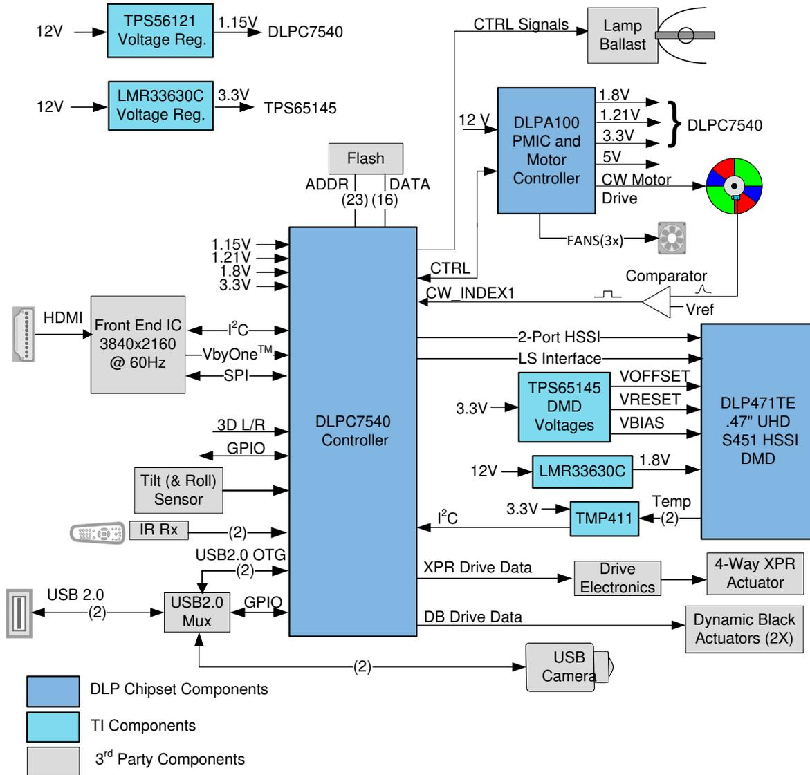
Figure 7-2. Typical 4K UHD Lamp Application Diagram
