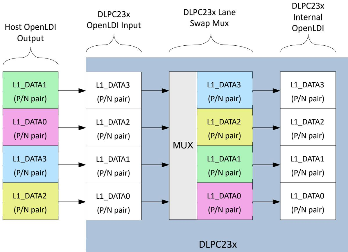
**Figure 7-4. Example of Alternate OpenLDI Port Lane Mapping**
