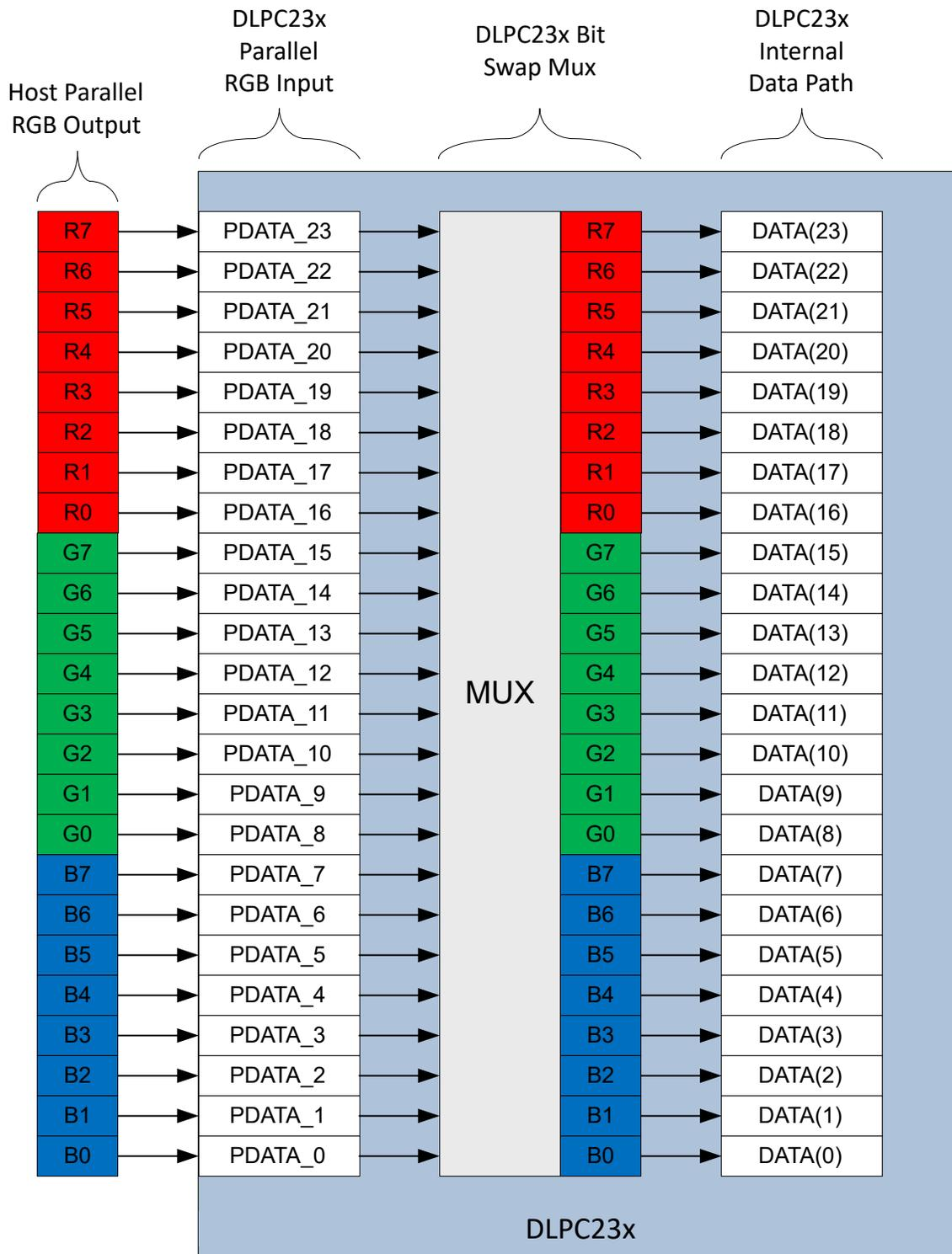
Figure 7-1. Example of Typical Parallel Port Bit Mapping
