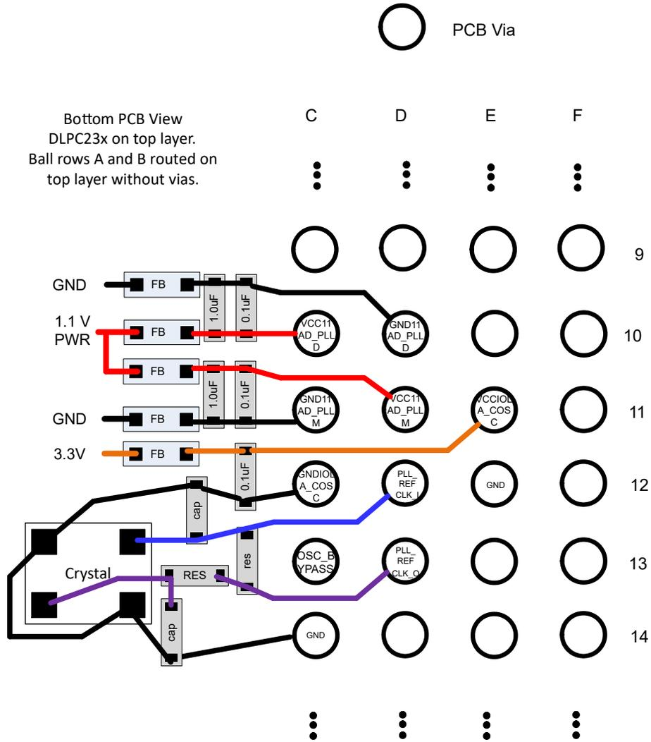
Figure 8-12. DLPC231-Q1 PLL Filter and Crystal Layout
