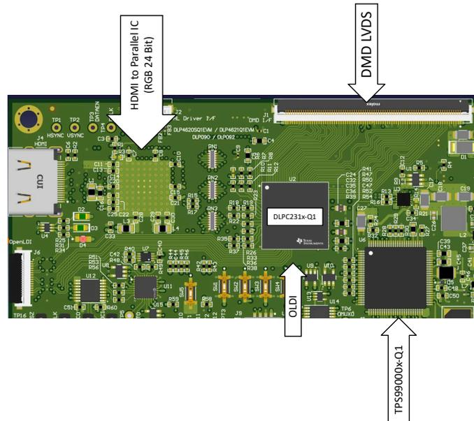
**Figure 8-16. Top level Layout Example—OLDI and DMD LVDS**
