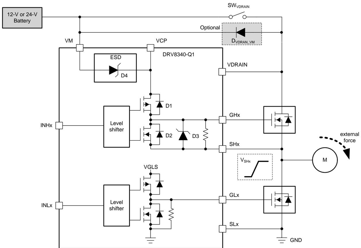
Figure 56. Power Supply Consideration in Generator mode
