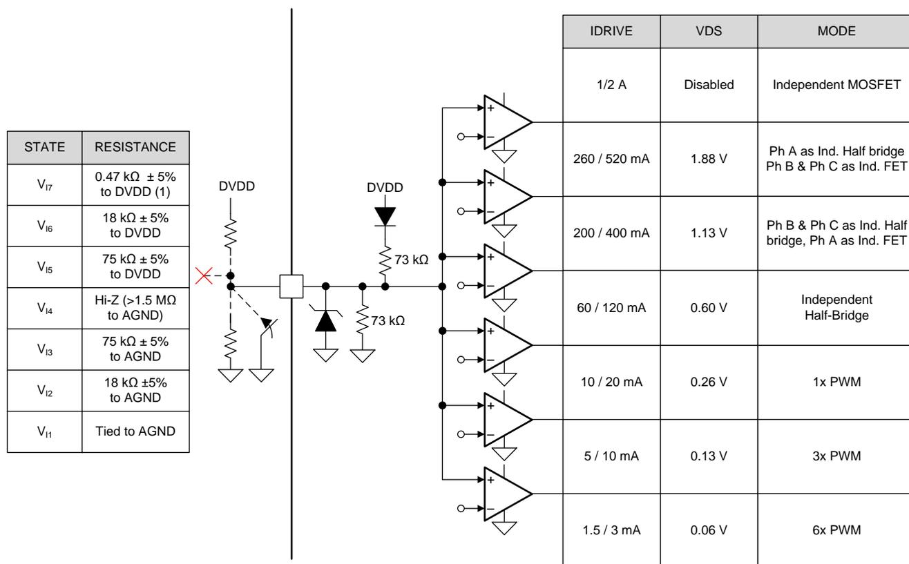
Figure 26. Seven Level Input Pin Structure <sup>(1)</sup>
