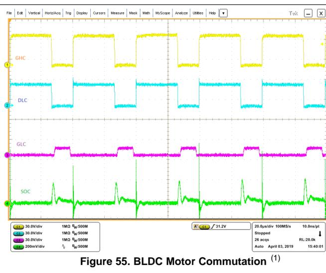
Figure 55. BLDC Motor Commutation (1)
