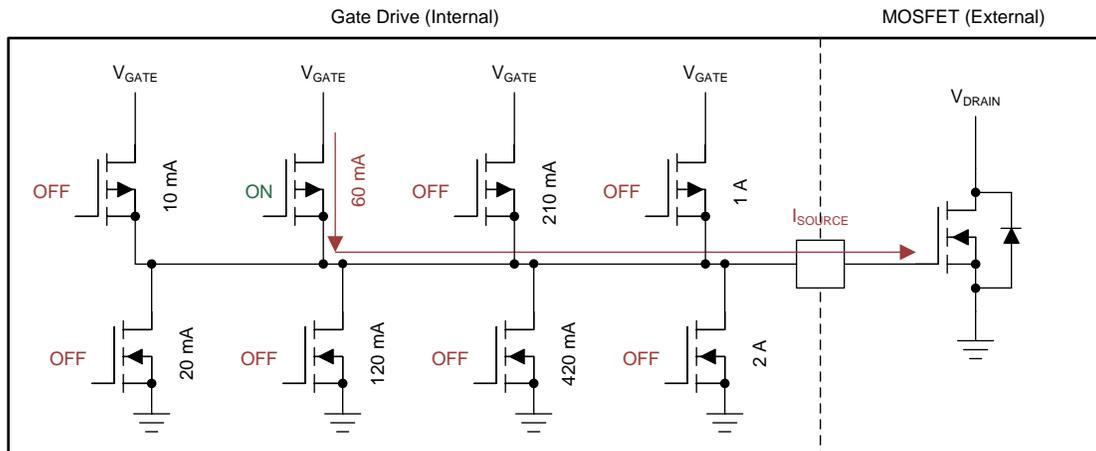
**Figure 19. Charge Pump Architecture**
