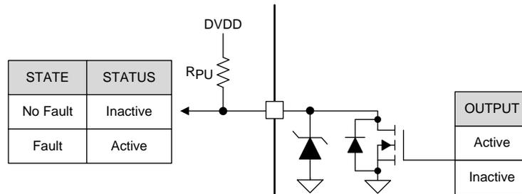
Figure 27. Open-Drain Output Pin Structure
