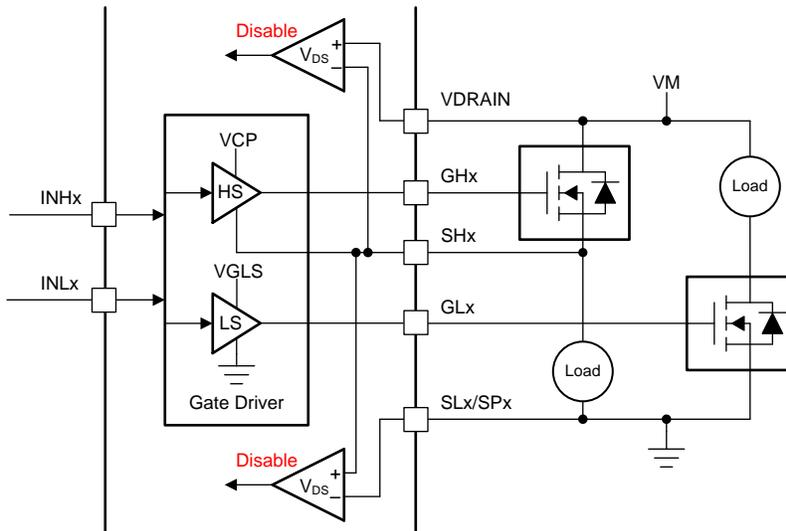
Figure 12. Independent PWM High-Side and Low-Side Drivers
