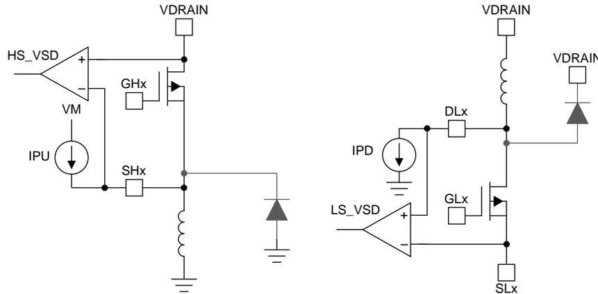
Figure 29. Load Configurations Not Supported
