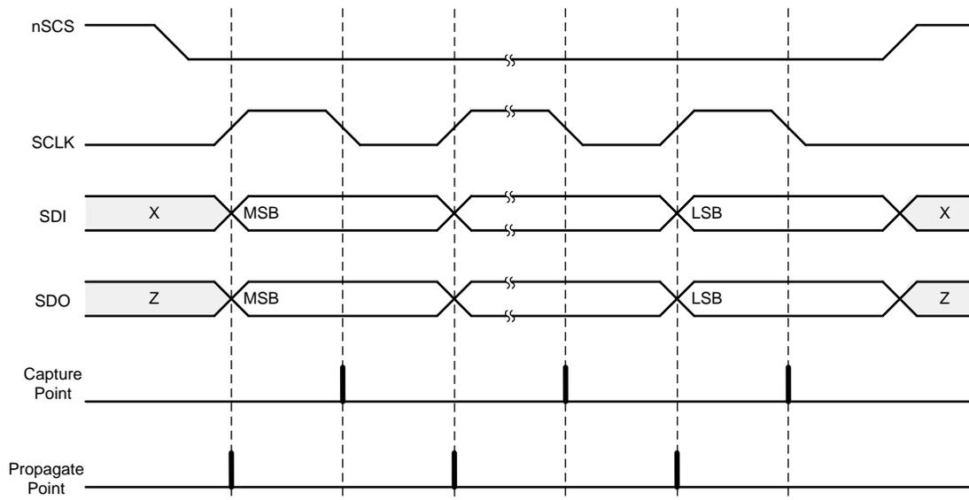
**Figure 34. SPI Slave Timing Diagram**
