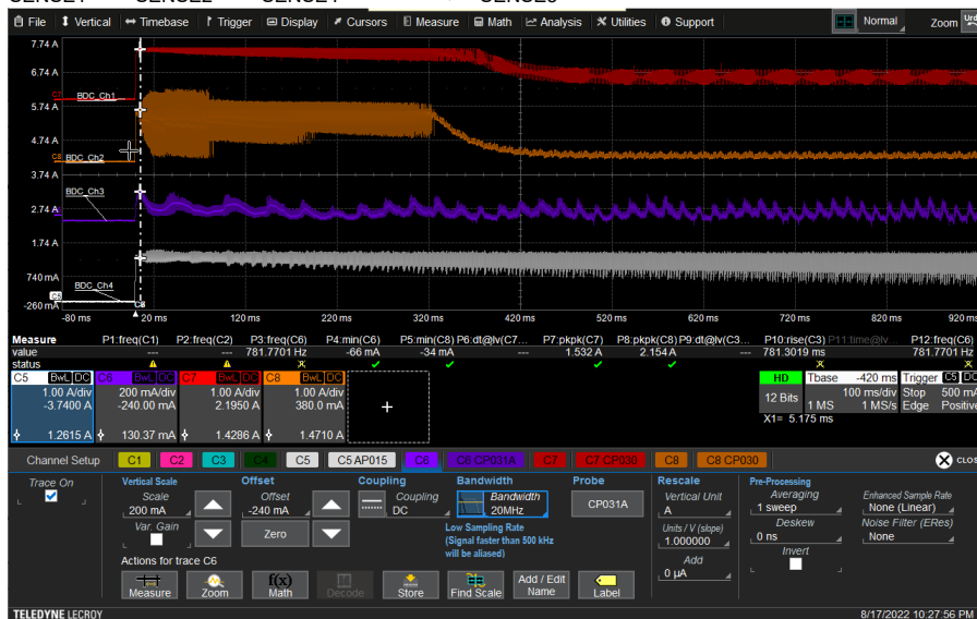
Figure 8-3. Driving four brushed-DC motors
