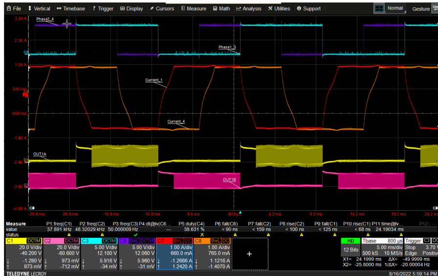
Figure 8-2. Driving two stepper motors in full-step
