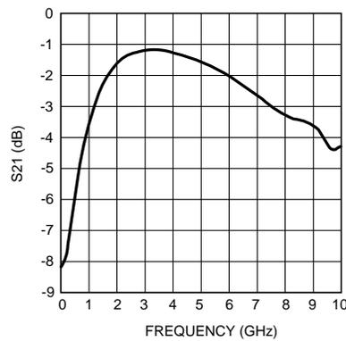
Figure 3. Typical Equalizer Transfer Function
