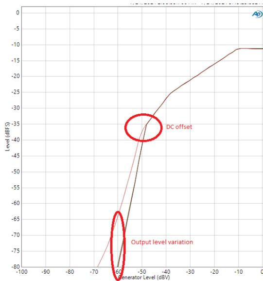
Figure 10: DRC Output Curve with 3 Knee Points
