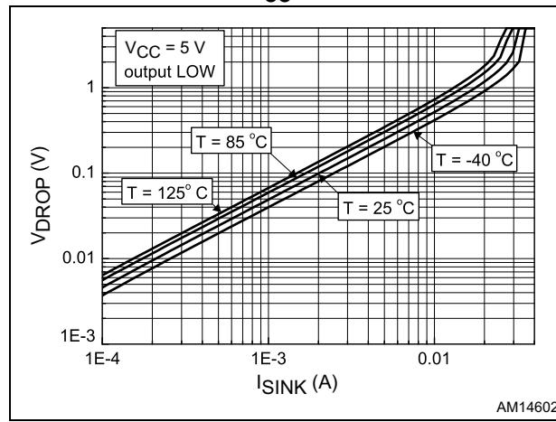
**Figure 19. Output voltage drop vs. source current at  $V_{CC} = 5$  V**
