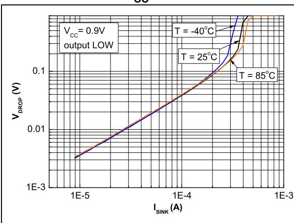
**Figure 37. Output voltage drop vs. source current at  $V_{CC} = 0.9\text{ V}$**
