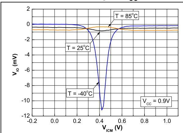
**Figure 35. Input voltage hysteresis vs. input common mode voltage at  $V_{CC} = 0.9\text{ V}$**
