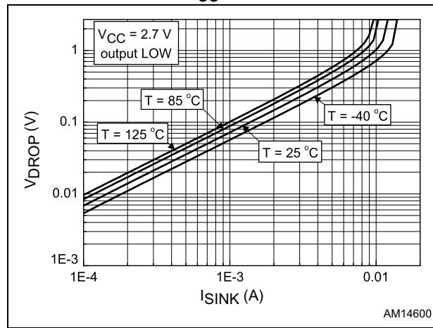
**Figure 17. Output voltage drop vs. source current at  $V_{CC} = 2.7$  V**
