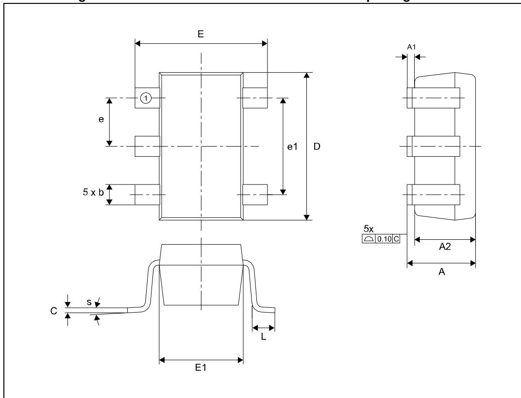
**Table 8. SOT23-5 - lead small outline transistor package mechanical data**
