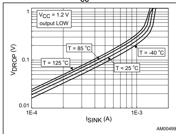
**Figure 15. Output voltage drop vs. source current at  $V_{CC} = 1.2$  V**
