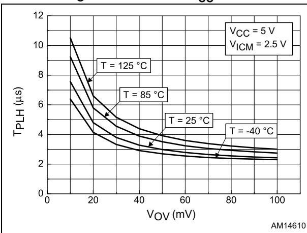
**Figure 27. Propagation delay  $T_{PHL}$  vs. input signal overdrive at  $V_{CC} = 5$  V**
