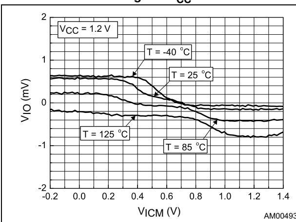
**Figure 9. Input hysteresis voltage vs. input common mode voltage at  $V_{CC} = 1.2\text{ V}$**
