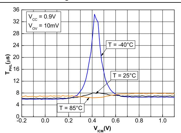
**Figure 41. Propagation delay  $T_{PHL}$  vs. input common mode voltage at  $V_{CC} = 0.9$  V and 100 mV signal overdrive**
