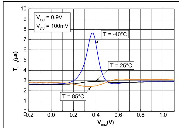
**Figure 42. Propagation delay  $T_{PLH}$  vs. input signal overdrive at  $V_{CC} = 0.9$  V**
