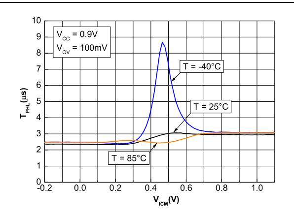
**Figure 43. Propagation delay  $T_{PHL}$  vs. input signal overdrive at  $V_{CC} = 0.9$  V**
