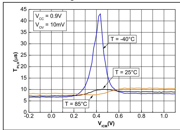
**Figure 40. Propagation delay  $T_{PLH}$  vs. input common mode voltage at  $V_{CC} = 0.9$  V and 100 mV signal overdrive**
