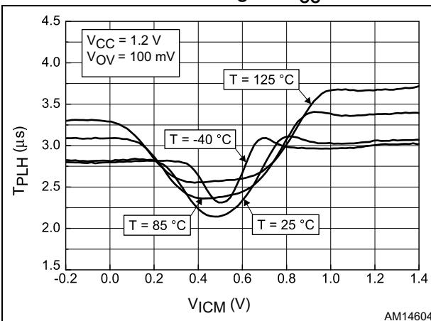
**Figure 21. Propagation delay  $T_{PHL}$  vs. input common mode voltage at  $V_{CC} = 1.2$  V**
