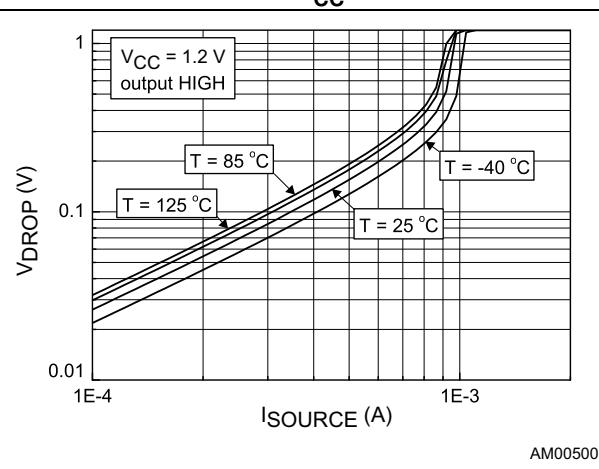
**Figure 16. Output voltage drop vs. sink current
