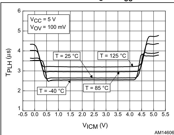
**Figure 23. Propagation delay  $T_{PHL}$  vs. input common mode voltage at  $V_{CC} = 5$  V**
