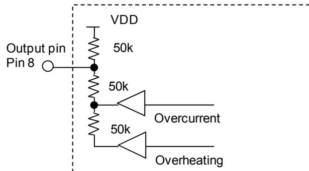
(The buffer has an open drain configuration.)
