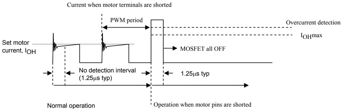
Overcurrent detection begins after an interval of no detection (a dead time of 1.25µs typ) during the initial ringing part during PWM operations. The no detection interval is a period of time where overcurrent is not detected even if the current exceeds  $I_{OH}$ .
