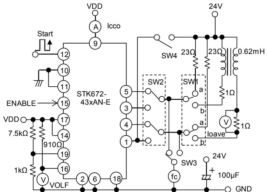
I<sub>oave</sub> measurement : Set switch SW2 in the setting SW1 to 'b'.
