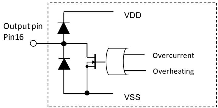
**2. Overcurrent detection, overheat detection functions**
