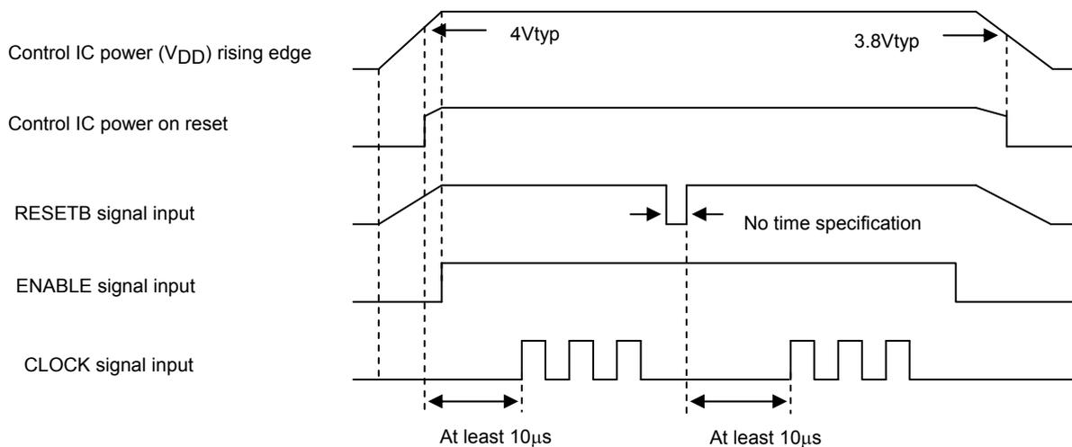
ENABLE, CLOCK, and RESETB Signals Input Timing
