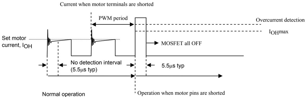
Overcurrent detection begins after an interval of no detection (a dead time of 5.5µs typ) during the initial ringing part during PWM operations. The no detection interval is a period of time where overcurrent is not detected even if the current exceeds IOH.
