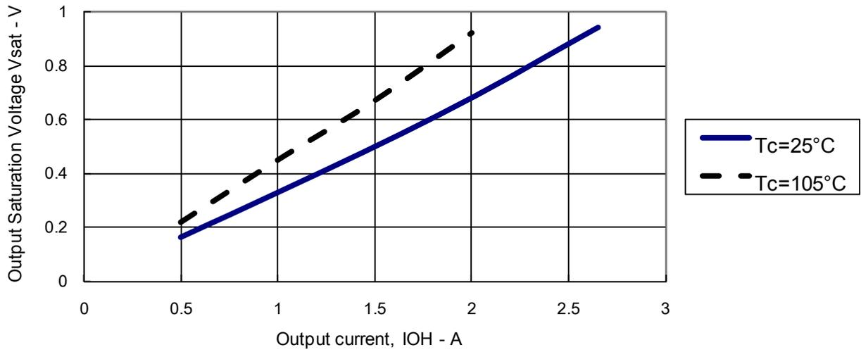
STK672-630AN/-632AN-E Forward voltage,  $V_{df}$  - Output current,  $I_{OH}$
