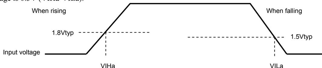
Input voltage specifications are as follows.  $V_{IH} = 2.5V_{min}$
