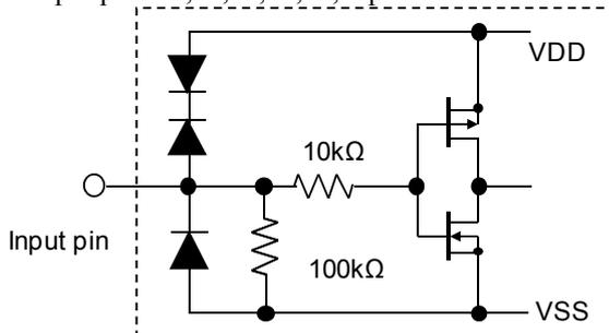
The input pins of this driver all use Schmitt input. Typical specifications at Tc=25°C are given below. Hysteresis voltage is 0.3V (VIHa-VILa).
