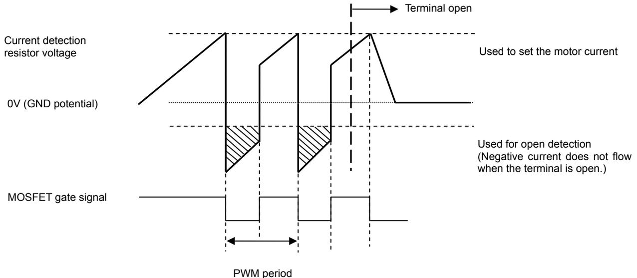
When the current level drops, the difference with the GND potential decreases, making detection difficult. The motor current that can be detected by motor terminal open detection is 1.1A or more with the STK672-432BN-E and 1.4A or more with the STK672-440BN-E/442BN-E.
