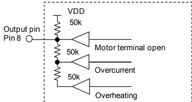
(The buffer has an open drain configuration.)
