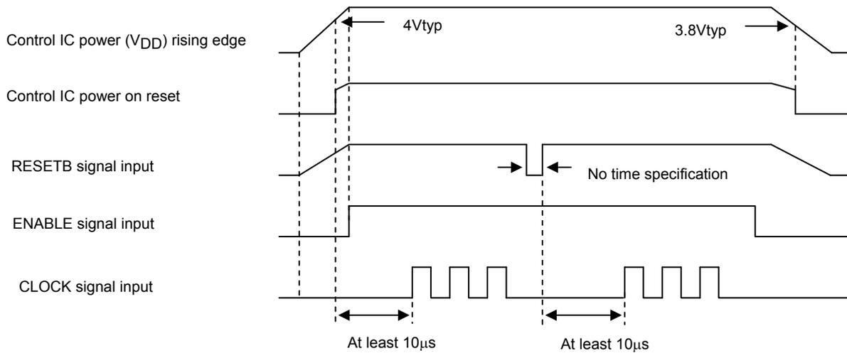
ENABLE, CLOCK, and RESETB Signals Input Timing
