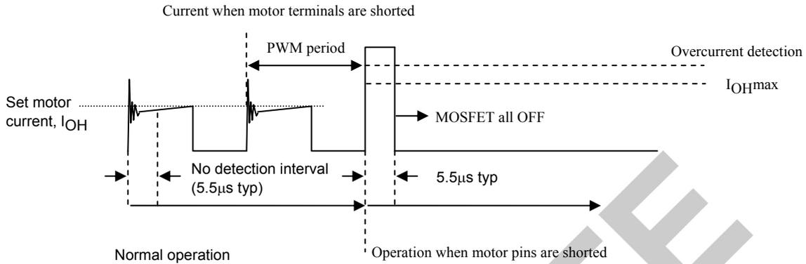
Overcurrent detection begins after an interval of no detection (a dead time of 5.5µs typ) during the initial ringing part during PWM operations. The no detection interval is a period of time where overcurrent is not detected even if the current exceeds  $I_{OH}$ .
