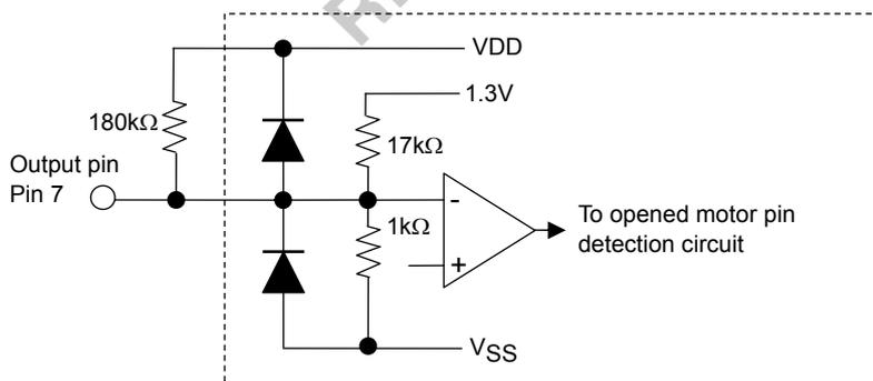
2. Overcurrent detection, overheat detection, and motor terminal open functions
