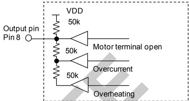
(The buffer has an open drain configuration.)
