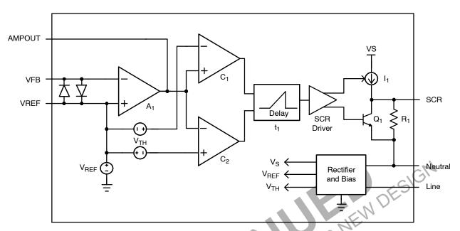
Figure 3. Block Diagram
