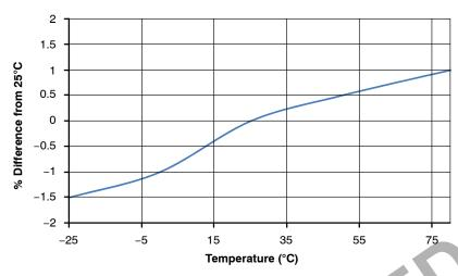
Figure 12. VThreshold ( $V_{TH}$ ) vs. Temperature
