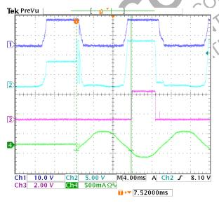
Ch1: V<sub>Line</sub> (Pin 3), 10 V/Div Ch2: AmpOut (Pin 6), 5 V/Div Ch3: SCR (Pin 1), 2 V/Div Ch4: I<sub>FAULT</sub>, 500 mA/Div
