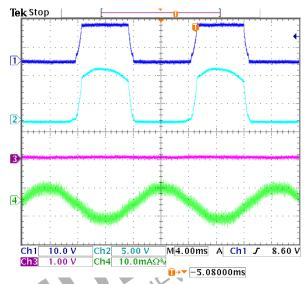
Ch1: V<sub>Line</sub> (Pin 3), 10 V/Div Ch2: AmpOut (Pin 6), 5 V/Div Ch3: SCR (Pin 1), 1 V/Div Ch4: I<sub>FAULT</sub>, 10 mA/Div
