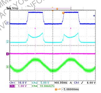
Ch1: V<sub>Line</sub> (Pin 3), 10 V/Div Ch2: AmpOut (Pin 6), 5 V/Div Ch3: SCR (Pin 1), 1 V/Div Ch4: I<sub>FAULT</sub>, 10 mA/Div
