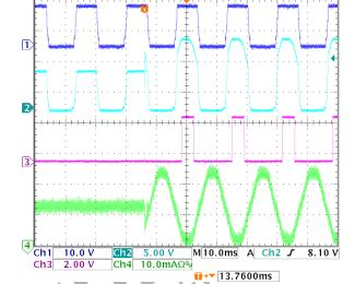
1 ms after AmpOut signal reaches 9.5 V, SCR is triggered.
