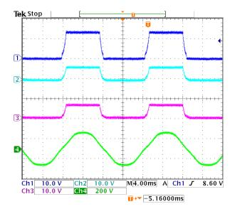
Ch1: V<sub>Line</sub> (Pin 3), 10 V/Div Ch2: AmpOut (Pin 6), 10 V/Div Ch3: V<sub>REF</sub> (Pin 4), 10 V/Div Ch4: V<sub>AC</sub> Input, 200 V/Div
