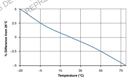
Figure 14. SCR Output Current (I<sub>OUT</sub>) vs. Temperature
