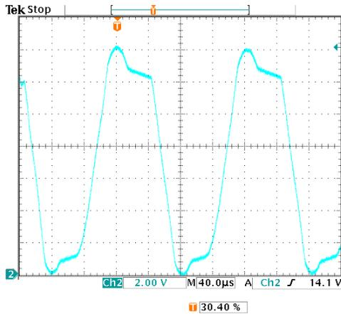
Ch2: AmpOut (Pin 6), 2 V/Div
