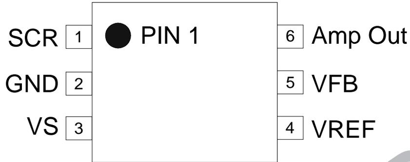
Figure 3. Pin Configuration
