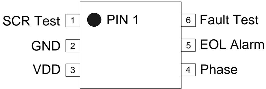
Figure 3. Pin Assignments
