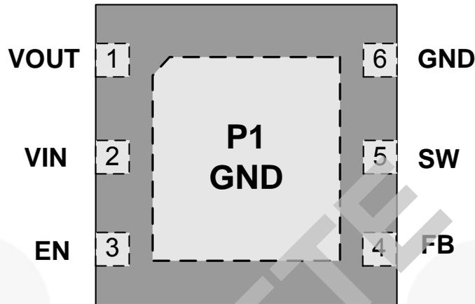
Figure 3. UMLP6 Package (Top View)
