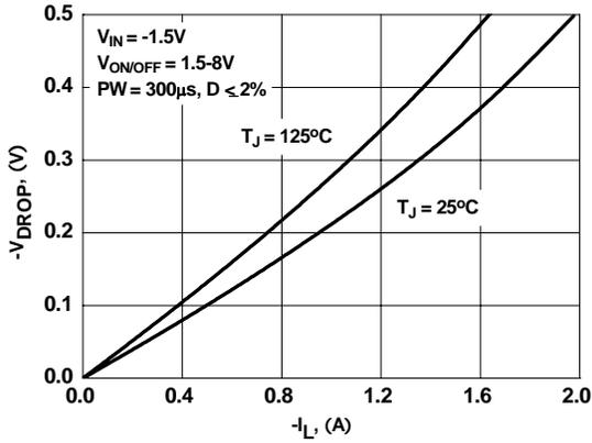
**Figure 1. Conduction Voltage Drop Variation with Load Current.**
