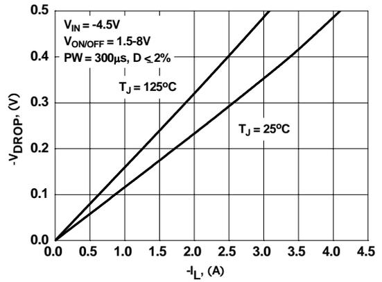
**Figure 4. Conduction Voltage Drop Variation with Load Current.**
