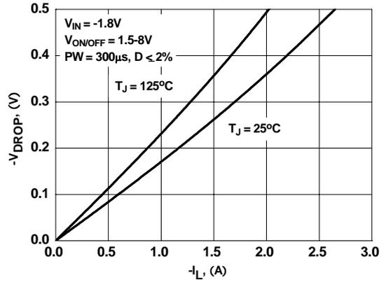
**Figure 2. Conduction Voltage Drop Variation with Load Current.**
